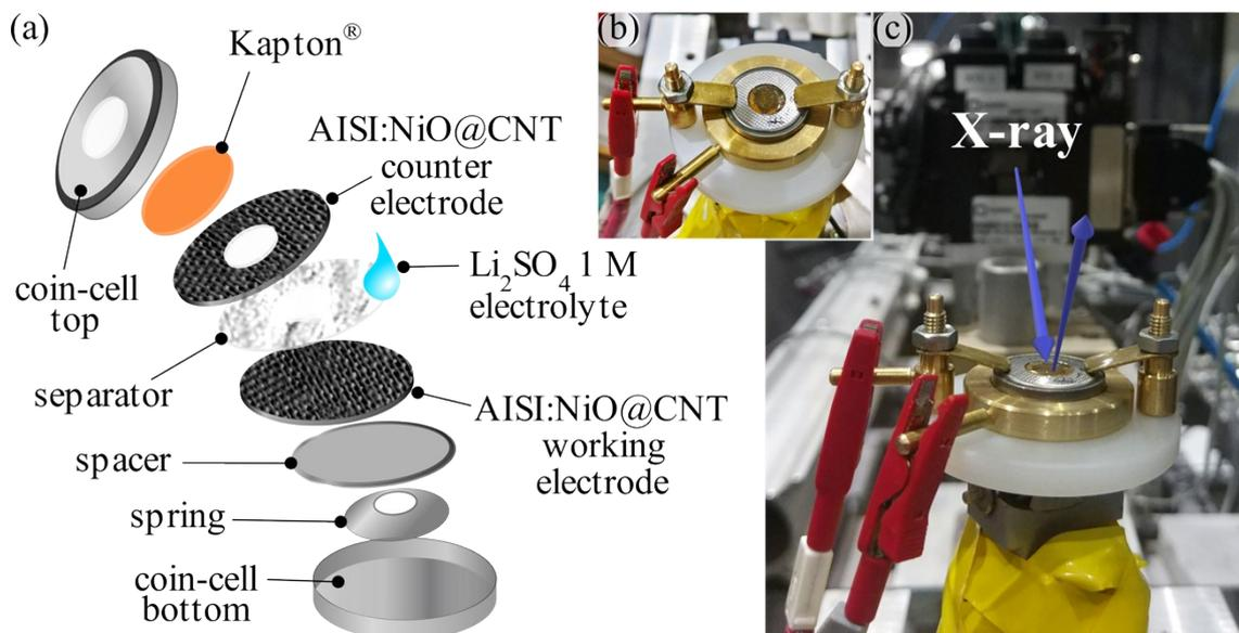
**Figure S1.** Measurements under dynamic polarization conditions: a) coin cell set up; b) top view of the coin cell installed in metallic adapter and positioned on the sample stage at the XPD beamline. There is a hole on the center of the coin cell which is covered with with a Kapton<sup>®</sup> foil to be transparent to the income and outcome x-ray and; c) a lateral view of the coin cell and the exhibiting the electrical contacts.
