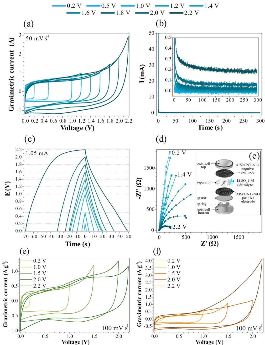
**Figure S2.** Electrochemical data from symmetric coin cell filled with a 1 M  $\text{Li}_2\text{SO}_4$  aqueous solution (a) Voltammetric curves up to 2.2 V; (b) chronoamperometry from 0.2 V to 2.2 V; (c) galvanostatic charge/discharge curves up to 2.2 V; (d) electrochemical impedance spectroscopy at constant cell voltages from 0.2V to 2.2V in steps of 0.4V and; (e) Coin cell set up for electrochemical measurements. (e) Cyclic voltamograms for MWCNT and (f) for NiO@MWCNT.
