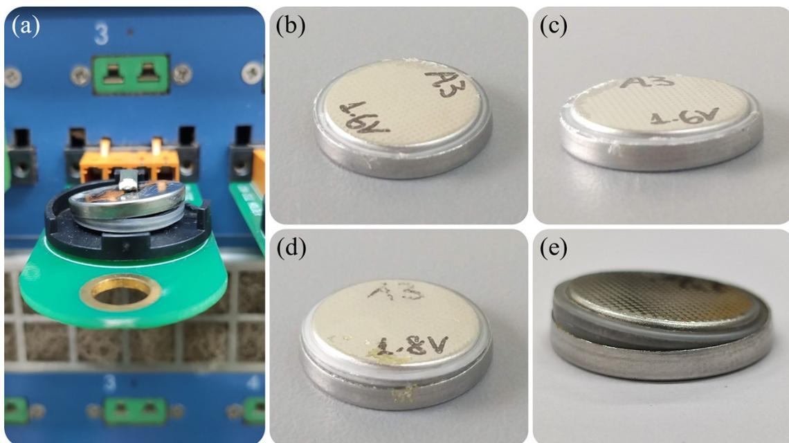
**Figure S5.** Coin cell used for electrochemical analysis: a) open-up coin cell after abusive regime of voltage applied; b) & c) undamaged coin cell under 1.6 V voltage; d) & e) damaged coin cell under 1.8 V voltage.
