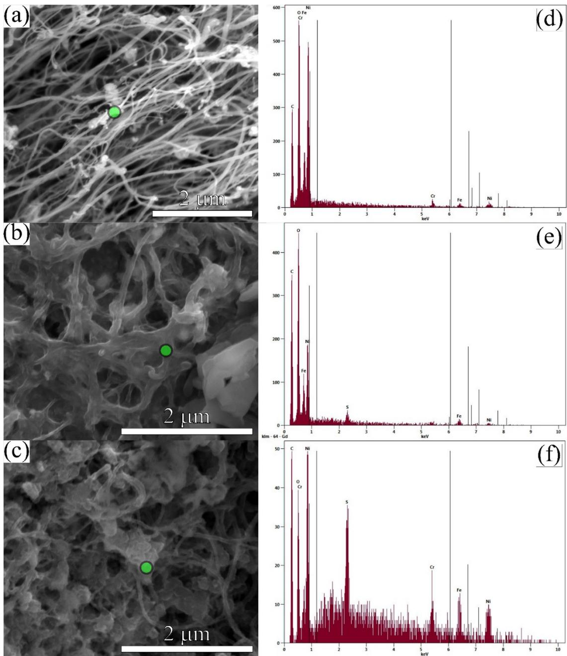
**Figure S4.** SEM data from (a) Pristine NiO@MWCNT electrode; electrodes after chronoamperometry of 30 min. (b) positive; (c) negative. EDS data from (d) Pristine NiO@MWCNT electrode; electrodes after chronoamperometry of 2.0 hours. (e) positive; (f) negative.
