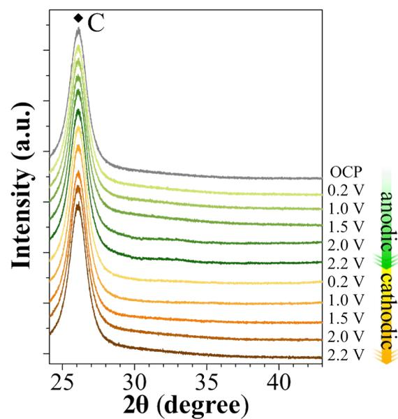
**Figure S3.** *Operando* XRD from MWCNTs electrodes in the coin cell. All XRD diffraction patterns were obtained under constant voltage during anodic polarization for MWCNTs anode (positive pole) green lines and MWCNTs cathode (negative pole) orange lines.
