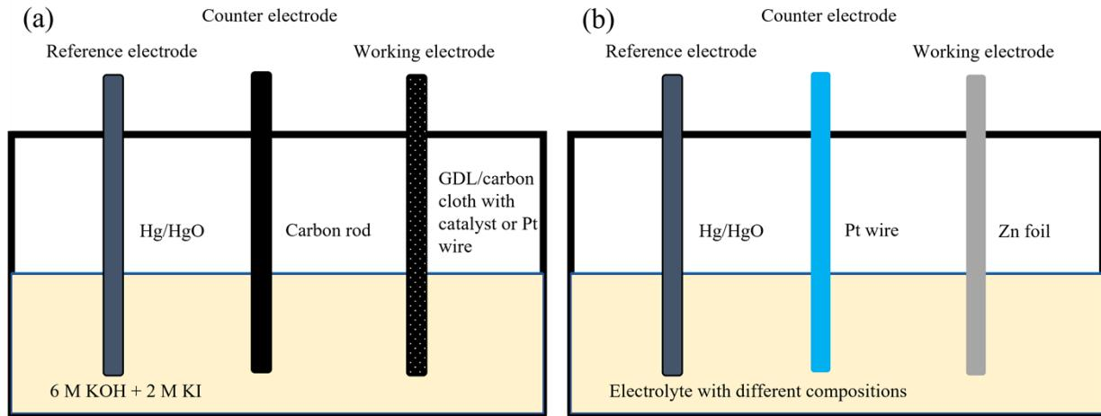
Figure S2. (a) Three-electrode setup for CV tests at the air electrode. (b) Three-electrode setup for CV tests at the Zn electrode.
