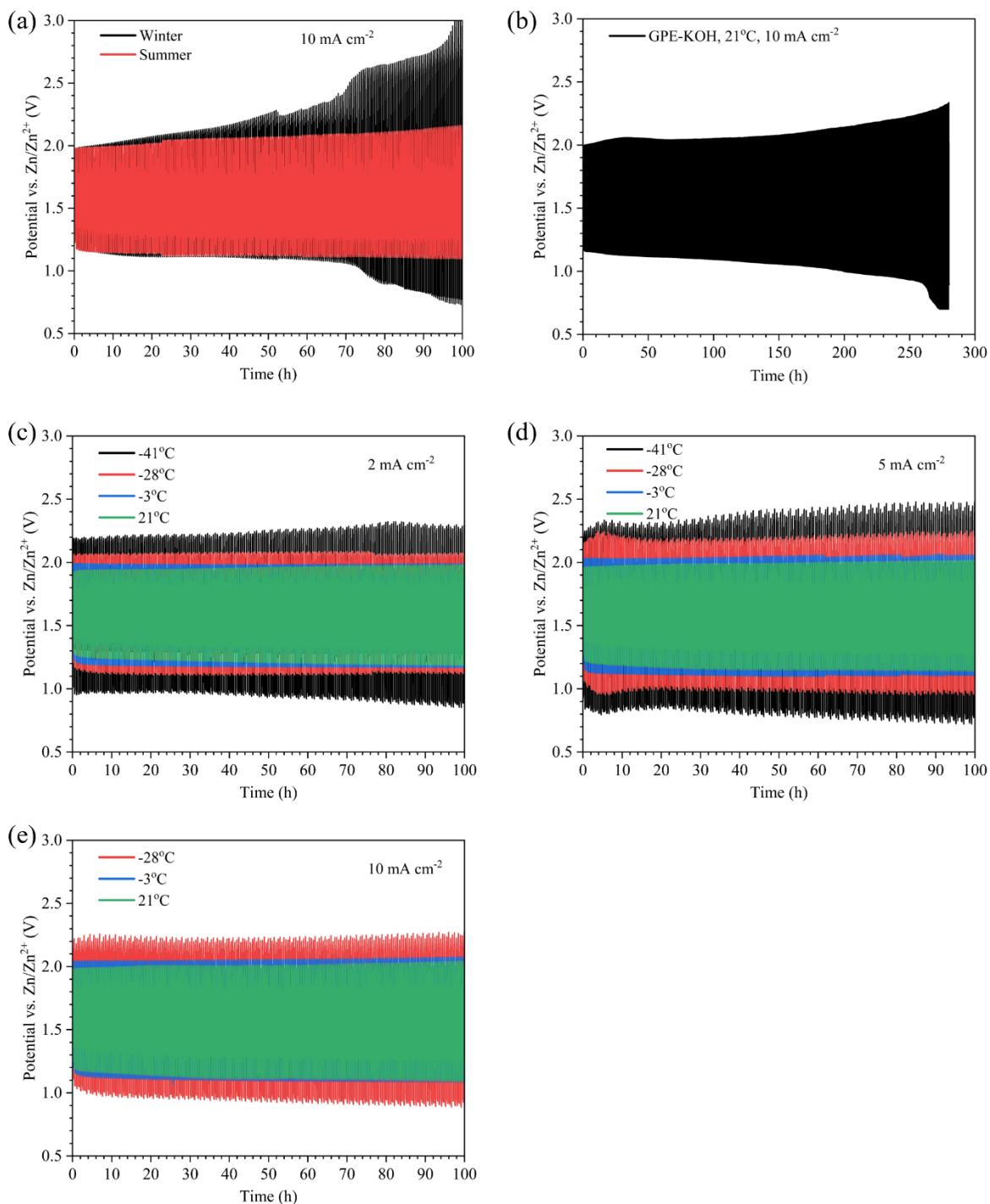
Figure S4. (a) Cyclability test at 21°C and 10 mA cm<sup>-2</sup> for ZAB using GPE-KOH in different seasons. (b) Full view of the lifetime test for ZAB using GPE-KOH. (c) Cyclability tests at different temperatures for ZABs using GPE-KOH and (Co,Fe)<sub>3</sub>O<sub>4</sub> coated GDL at (c) 2 mA cm<sup>-2</sup>, (d) 5 mA cm<sup>-2</sup>, (e) 10 mA cm<sup>-2</sup>.
