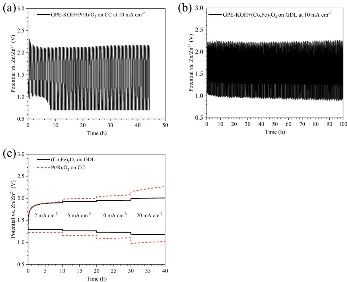
Figure S3. (a) Cyclability test at 21°C and 10 mA cm<sup>-2</sup> for ZAB using GPE-KOH and Pt/RuO<sub>2</sub> coated CC as the air electrode. (b) Cyclability test at 21°C and 10 mA cm<sup>-2</sup> for ZAB using GPE-KOH and (Co,Fe)<sub>3</sub>O<sub>4</sub> coated GDL. (c) Rate test results for ZABs using GPE-KOH with (Co,Fe)<sub>3</sub>O<sub>4</sub> on GDL and Pt/RuO<sub>2</sub> on CC as the air electrode at 21°C.
