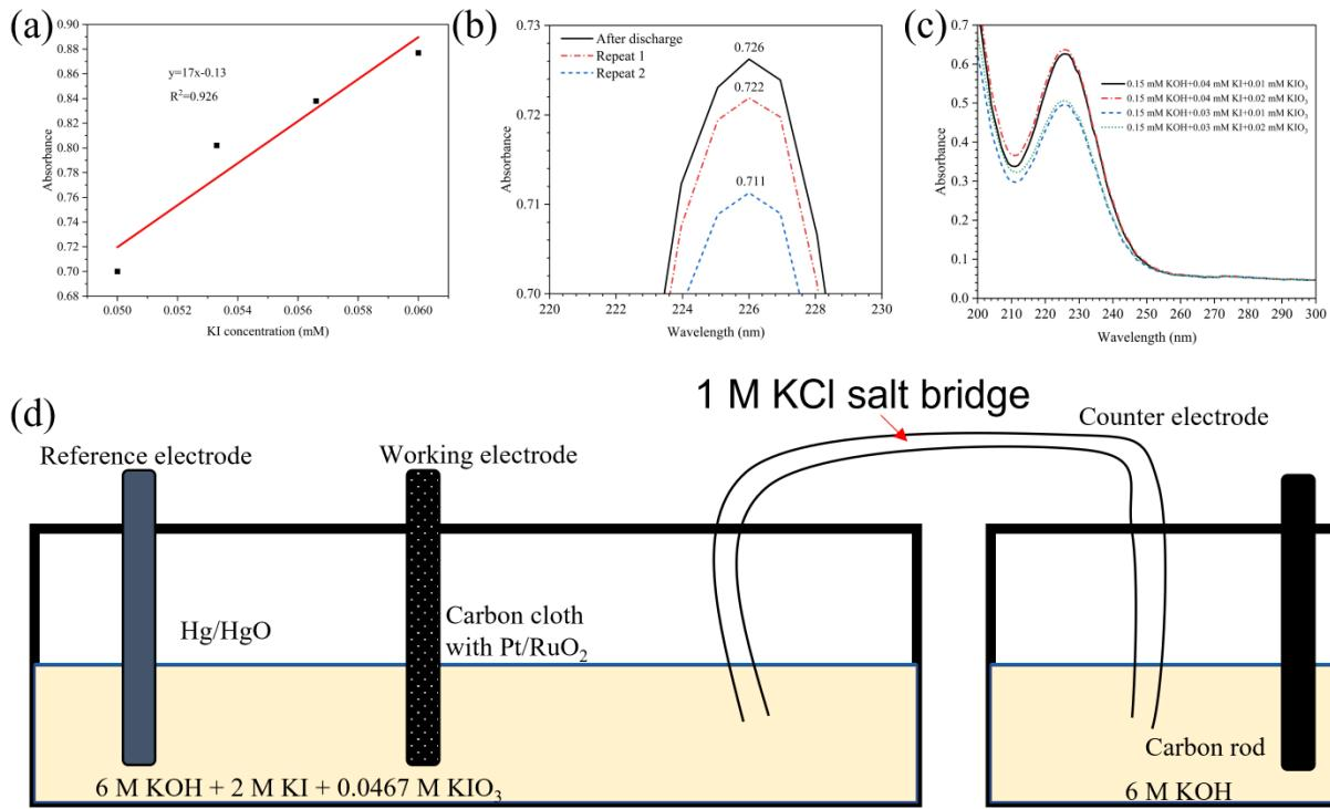
Figure S10. (a) Absorbance vs. KI concentration. This plot was created using the data in Figure 7d. UV-vis spectra for (b) sample A after discharge and with repeated diluted samples to confirm reproducibility, and (c) solutions with different concentrations of KI and KIO<sub>3</sub>. (d) The three-electrode setup for the half-cell discharge process.
