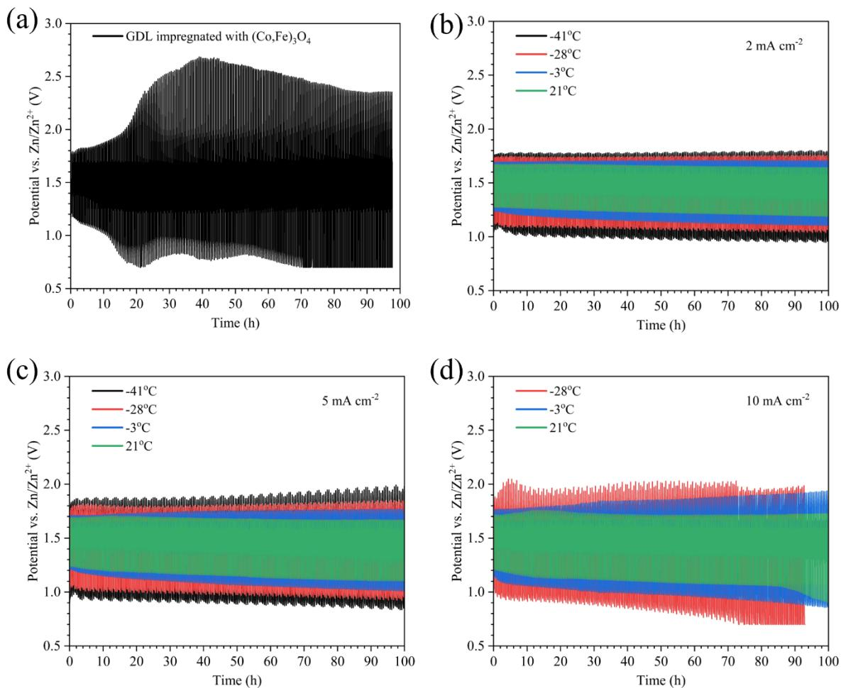
Figure S5. (a) Cyclability test at  $10 \text{ mA cm}^{-2}$  using aqueous  $6 \text{ M KOH} + 2 \text{ M KI} + 0.4 \text{ M ZnO}$  as the electrolyte and GDL with  $(\text{Co},\text{Fe})_3\text{O}_4$  decorated N-CNTs as the air electrode. Cyclability tests at different temperatures for ZABs using GPE-KOH-KI and Pt/RuO<sub>2</sub> coated CC at (b)  $2 \text{ mA cm}^{-2}$ , (c)  $5 \text{ mA cm}^{-2}$ , and (d)  $10 \text{ mA cm}^{-2}$ .
