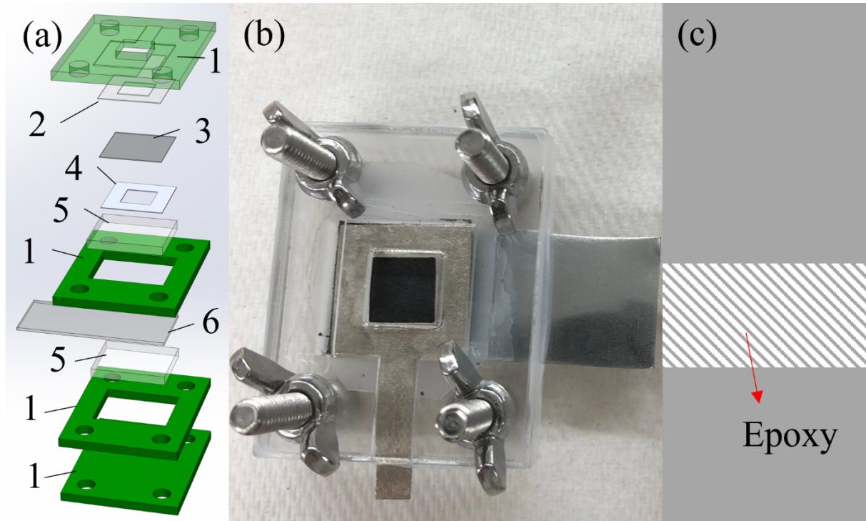
Figure S1. (a) Schematic of the sandwich-type cell in a disassembled view. (b) Optical image of the sandwich-type cell in an assembled view. (c) Illustration of Zn foil coated with epoxy. Note that the numbers correspond to the following: 1) Acrylic sheets, 2) Ni current collector, 3) GDL or carbon cloth coated with electrocatalyst, 4) polypropylene film, 5) GPE, and 6) Zn foil.
