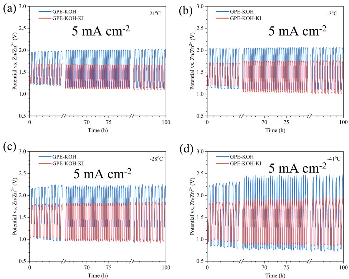
Figure S8. Comparison of cyclability test results for ZABs using  $(\text{Co},\text{Fe})_3\text{O}_4$  coated GDL with GPE-KOH and Pt/RuO<sub>2</sub> coated CC with GPE-KOH-KI at  $5 \text{ mA cm}^{-2}$  at (a)  $21^\circ\text{C}$ , (b)  $-3^\circ\text{C}$ , (c)  $-28^\circ\text{C}$ , and (d)  $-41^\circ\text{C}$ .
