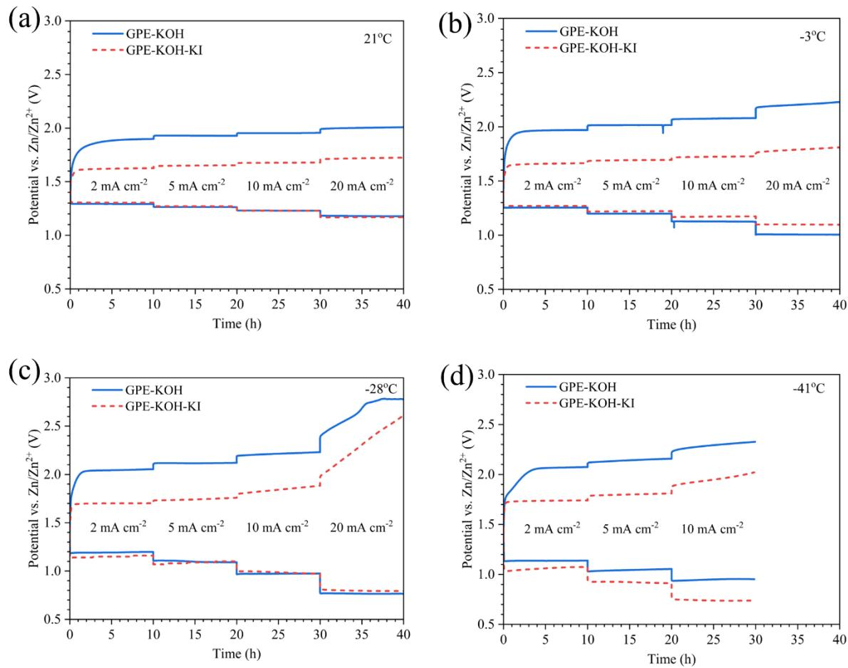
Figure S6. Comparison of rate test results for ZABs using  $(\text{Co},\text{Fe})_3\text{O}_4$  coated GDL with GPE-KOH and Pt/RuO<sub>2</sub> coated CC with GPE-KOH-KI at (a) 21°C, (b) -3°C, (c) -28°C, and (d) -41°C.
