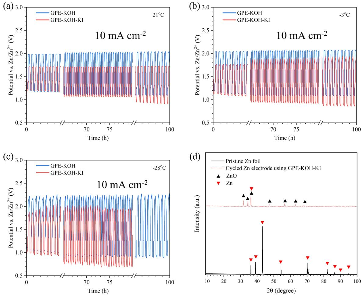
Figure S9. Cyclability test results for ZABs using  $(Co,Fe)_3O_4$  coated GDL with GPE-KOH and Pt/RuO<sub>2</sub> coated CC with GPE-KOH-KI at  $10 \text{ mA cm}^{-2}$  at (a)  $21^{\circ}C$ , (b)  $-3^{\circ}C$ , and (c)  $-28^{\circ}C$ . (d) XRD patterns for pristine Zn foil and the Zn electrode after cycling using GPE-KOH-KI at  $21^{\circ}C$  and  $10 \text{ mA cm}^{-2}$  for 100 h.
