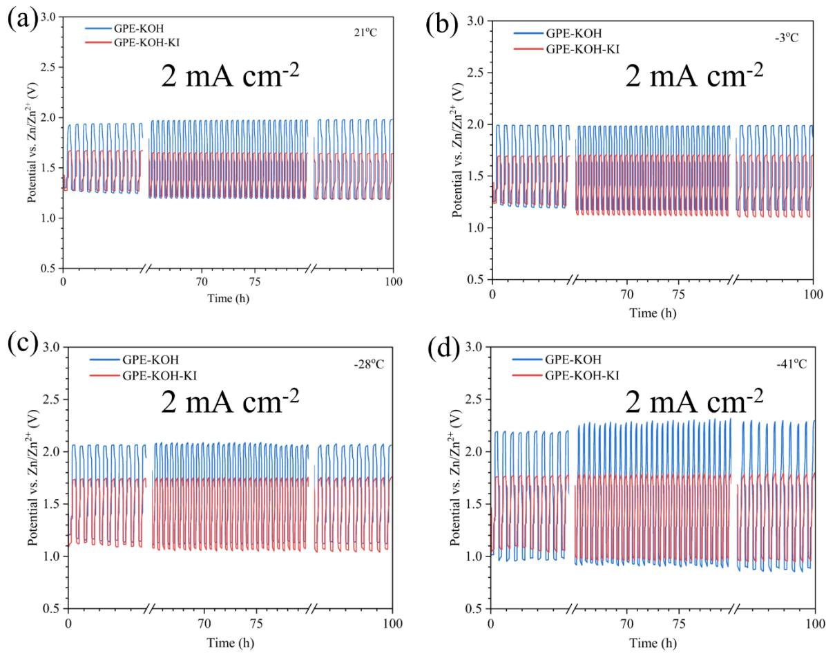
Figure S7. Cyclability test results for ZABs using  $(\text{Co}, \text{Fe})_3\text{O}_4$  coated GDL with GPE-KOH and Pt/RuO<sub>2</sub> coated CC with GPE-KOH-KI at  $2 \text{ mA cm}^{-2}$  at (a)  $21^\circ\text{C}$ , (b)  $-3^\circ\text{C}$ , (c)  $-28^\circ\text{C}$ , and (d)  $-41^\circ\text{C}$ .
