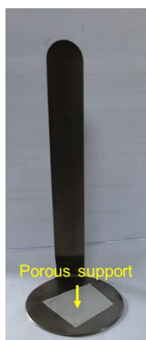
Figure S2 | Fabricated stainless-steel plate for transferring the COF nanofilm to the porous substrate after interfacial polymerization.
