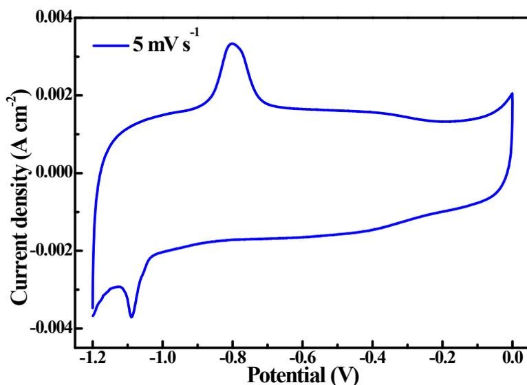
**Supplementary Fig. 7** The enlarged CV curve of Fe<sub>2</sub>O<sub>3</sub>@ACC at a scan rate of 5 mV s<sup>-1</sup>.
