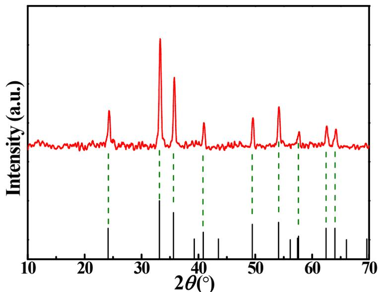
**Supplementary Fig. 5** The measured PXRD pattern of as-synthesized Fe<sub>2</sub>O<sub>3</sub>@ACC and the PXRD pattern of Fe<sub>2</sub>O<sub>3</sub> (PDF # 33-0664) obtained from the powder diffraction file (PDF). Note: the interference peaks from the ACC are subtracted in the measured PXRD for clarity.
