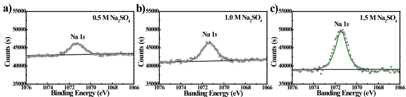
**Supplementary Fig. 3** High resolution XPS spectra of Na 1s region for a series of  $\delta$ - $(\text{Na}^+\text{Mn}^{3+y}\text{Mn}^{4+1-y})\text{O}^{2-}_2@ACC$ , in which  $\text{Na}^+$  was inserted by CV sweep at electrolyte concentration of (a) 0.5 M  $\text{Na}_2\text{SO}_4$ , (b) 1.0 M  $\text{Na}_2\text{SO}_4$ , and (c) 1.5 M  $\text{Na}_2\text{SO}_4$ , respectively, for 500 times.
