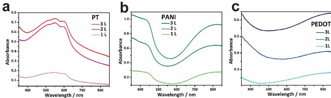
**Figure S2.** Absorbance spectra of the original ECP films with different number of layers.
