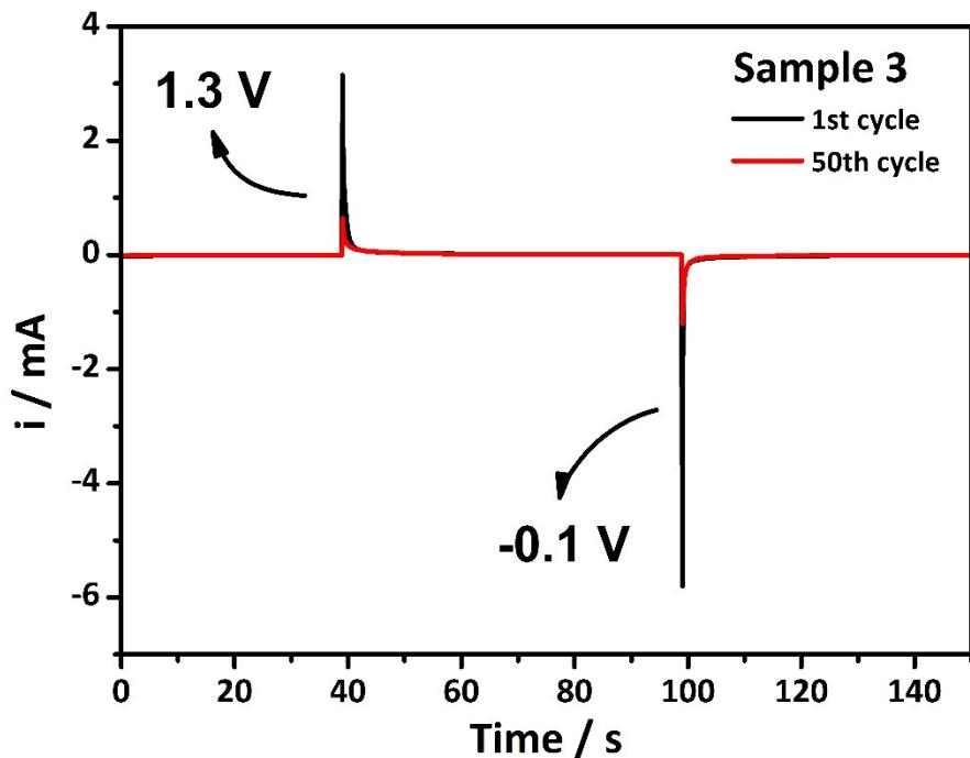
**Figure S9.** Chronoamperograms curves. Current response during time as a function of the applied potential for the 1<sup>st</sup> and 50<sup>th</sup> cycles for PEDOT-1L/PT-1L.
