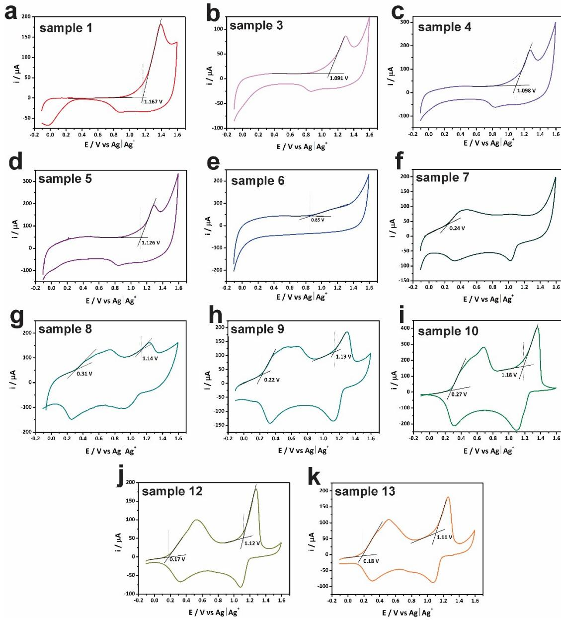
**Figure S8.** Cyclic voltammetry curves showing onset potentials were recorded at  $10 \text{ mV s}^{-1}$  in acetonitrile with lithium perchlorate  $0.1 \text{ mol L}^{-1}$ . The electrochemical potential was calibrated using the ferrocene/ferrocenium redox pair. The electrolyte was bubbling with  $\text{N}_2(\text{g})$  for 10 minutes previously each measurement.
