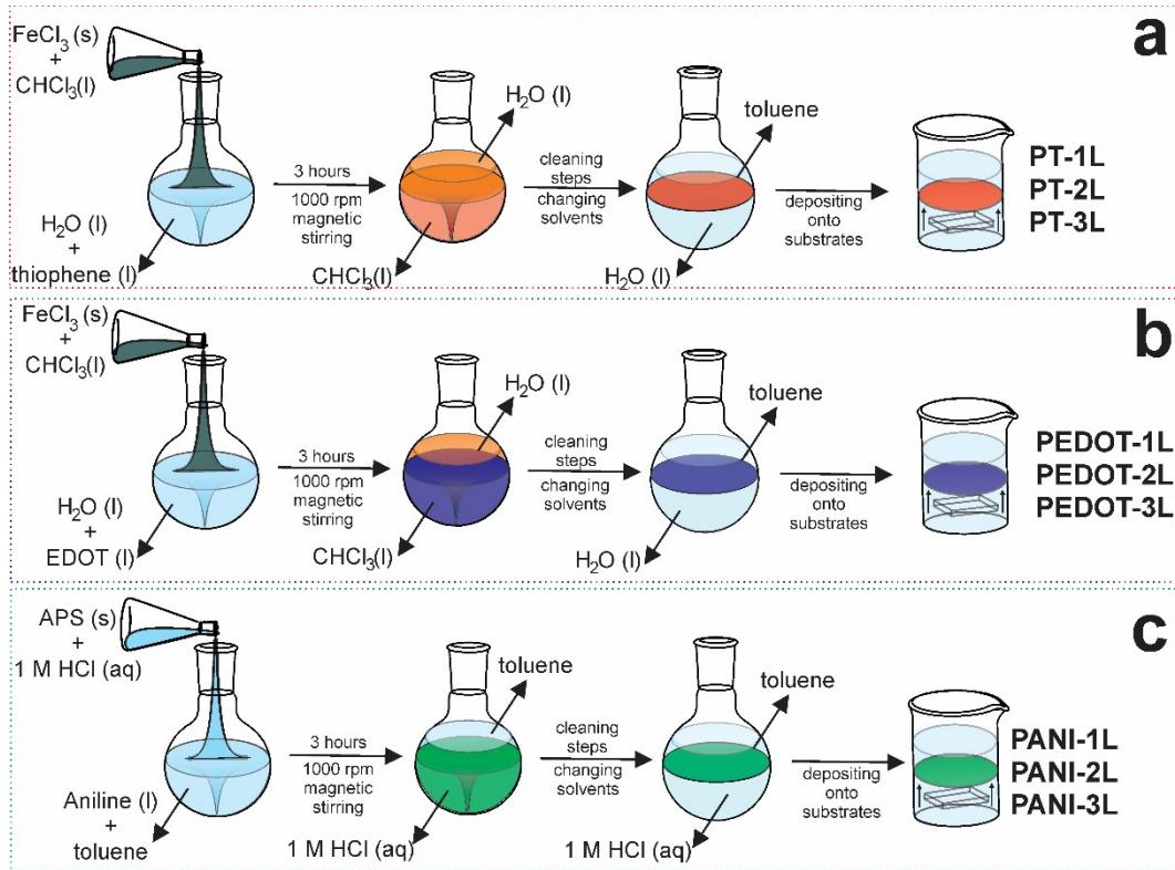
**Figure S1.** Synthesis of the ECPs. Schematic representation of liquid-liquid interfacial route to produce self-assembly thin film of a) polythiophene (PT), b) polydioxothiophene (PEDOT), and c) polyaniline (PANI).
