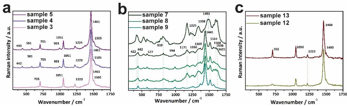
**Figure S6.** Representative Raman spectra of the color palette samples. (a) Sample 3 (light pink), sample 4 (violet), sample 5 (purple); (b) sample 9 (teal, one spectrum), sample 8 (green, two spectra), sample 7 (dark green, two spectra); (c) sample 12 (dark yellow), sample 12 (brown).
