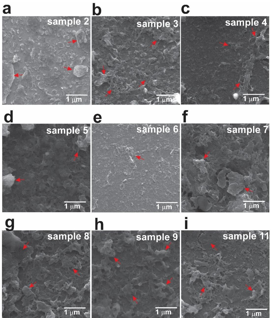
**Figure S7.** Scanning electron microscopy images of original and stacking samples. Red arrows point out the fibrillary aggregates of polymers.
