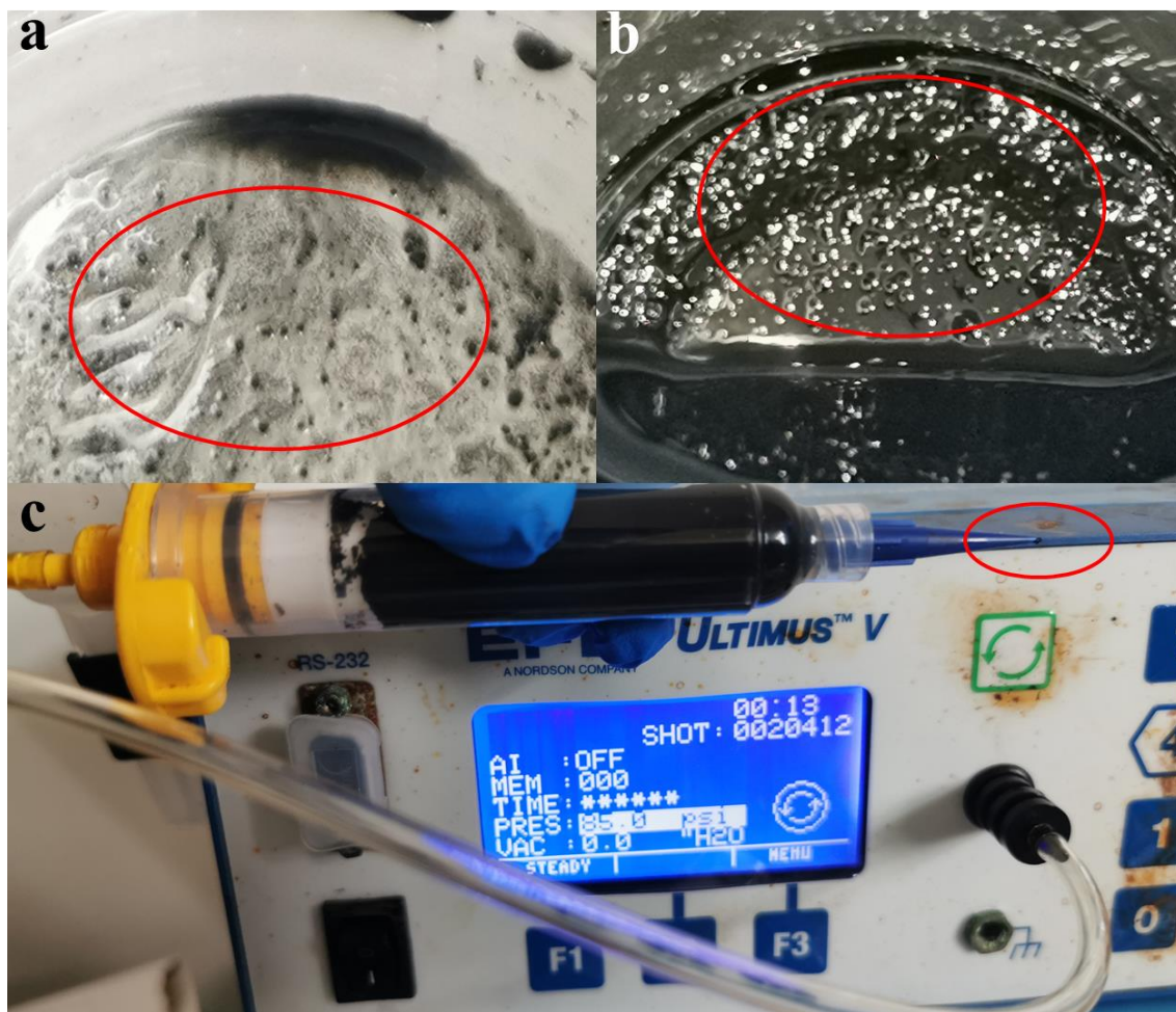
Fig. S5. The photographs of the plastic cup's bottom (red marked)-remaining PA ink with a higher CNT content of 16.4 wt%: a) the freshly prepared ink, b) the ink after resting for some time (before gelation); and c) a photograph of the needle (inner diameter: 410 \mu\text{m} ) becoming blocked (red marked) when the ink (CNT content: 16.4 wt%) was forced out even at a maximum applied pressure of 85 psi ( \approx 5.86 bar).
