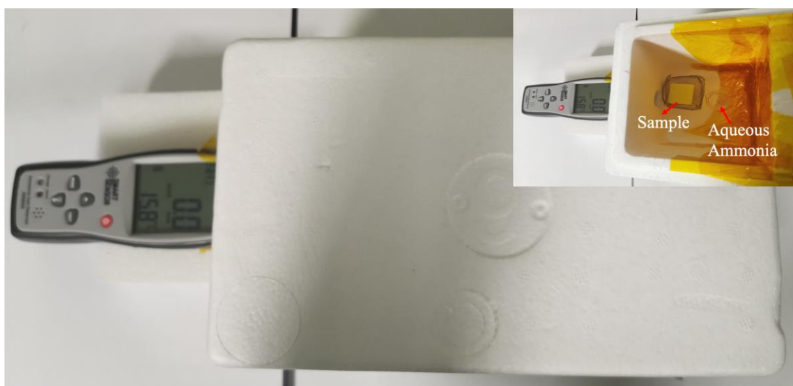
Fig. S22. A designed simplistic experiment setup of ammonia adsorption tests.
