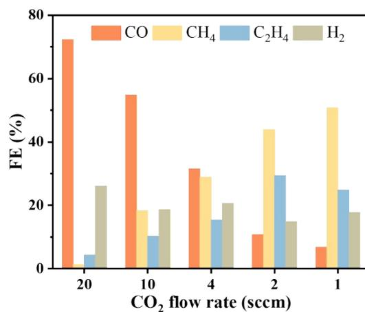
**Supplementary Figure S6.** FEs of HPH-Cu in acidic electrolytes at different CO<sub>2</sub> flow rates.
