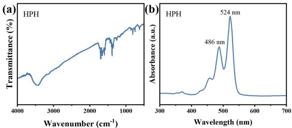
Supplementary Figure S1. (a) FTIR spectrum and (b) UV-vis absorption spectrum of HPH.
