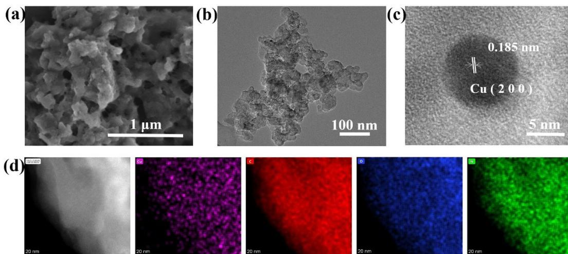
**Supplementary Figure S9.** (a) SEM image, (b) TEM image, (c) High-resolution TEM image and (d) Elemental mapping images of HPH-Cu after electrolysis.
