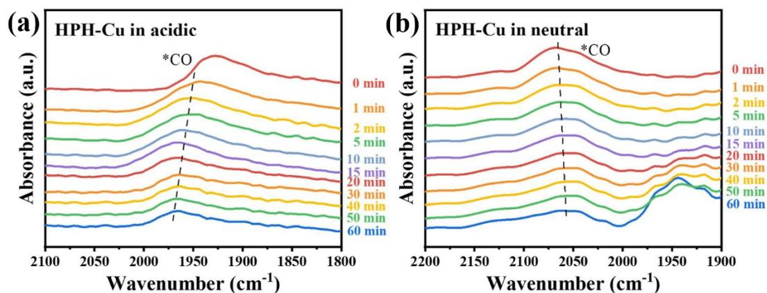
**Supplementary Figure S13.** In situ ATR-SEIRAS spectra of CO desorption after -1.2 V vs. Ag/AgCl electrolysis in CO<sub>2</sub>-saturated (a) acidic and (b) neutral electrolytes.
