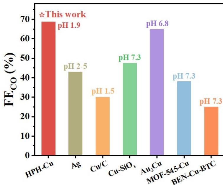
**Supplementary Figure S5.** Comparison of Faradaic efficiency of CO and pH of electrolyte with HPH-Cu and other reported CO<sub>2</sub>RR catalysts.
