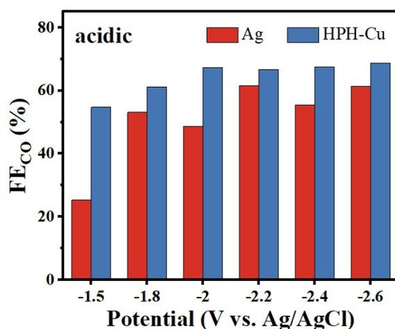
**Supplementary Figure S12.** The FE<sub>CO</sub> of HPH-Cu and Ag in acidic electrolyte.
