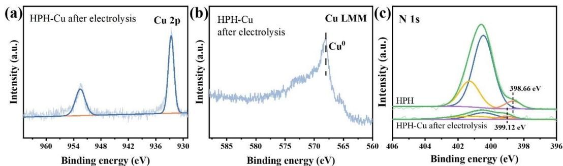
**Supplementary Figure S11.** (a) Cu 2p and (b) Cu LMM XPS spectra of HPH-Cu after electrolysis; (c) XPS N 1s spectra of HPH and HPH-Cu after electrolysis.
