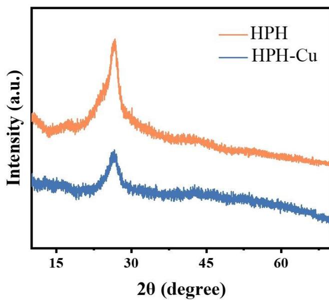
**Supplementary Figure S10.** XRD patterns of HPH and HPH-Cu.
