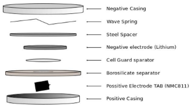
Figure S4: Schematic diagram of coin cell set up for electrochemistry.
