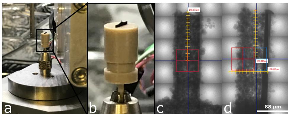
Figure S5: a) Photograph of electrode set up within tomography microscope. b) Zoomed in photograph of the electrode with tab appendage inside custom built holder. c) Radiograph of tab front view with ROI box in red. d) Radiograph of tab side view with ROI boxes in red and blue showing the position at which tomographies were taken.
