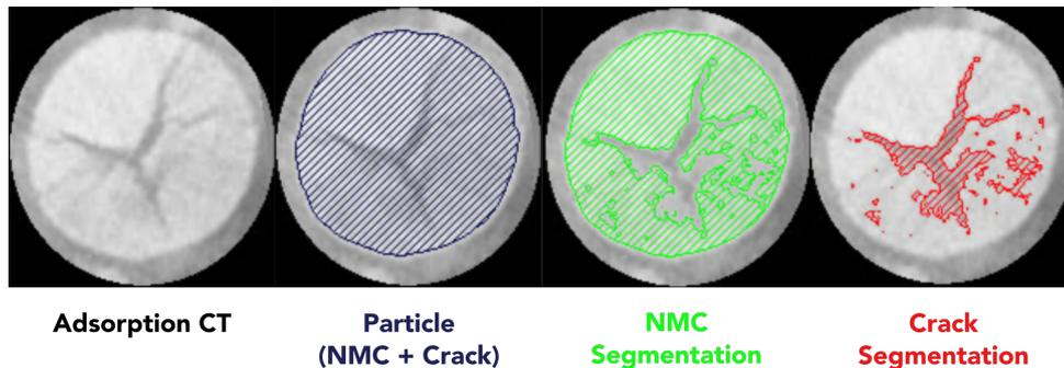
Figure S2: Ortho slices of Particle 3 showing segmentation of different phases used in analysis as shown. Particle analysis was used for particle volume expansion. NMC and crack segmentations were
