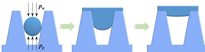
Fig. S7 Schematic depicting the condensation process and the effect of air pressure on the surfaces of Compact
