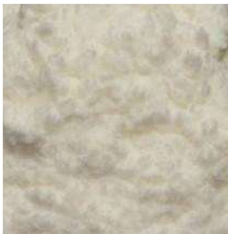
Fig. S1. Photograph of the delignified sorghum. *Note: To capture a photograph, a solid sample was intentionally prepared through freeze-drying.
