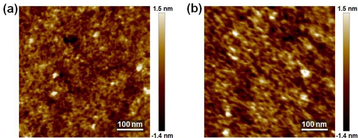
**Fig. S4** AFM topological images of the (a) PBI-monoPip-2.5 and (b) PBI-bisPip-2.5 membranes.
