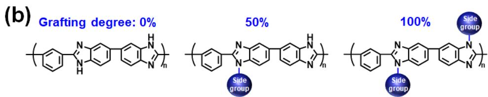
**Fig. S5** (a) Grafting degree vs. IEC of the PBI-monoPip and PBI-bisPip membranes, and (b) schematic representations of PBI units with different grafting degrees.
