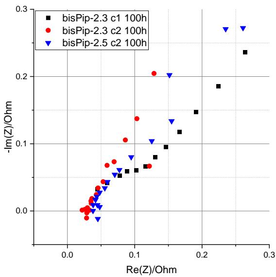
**Fig. S9.** The high frequency end of the impedance spectra of the cells with the PBI-bisPip membranes after the 100 h test shows no significant change of the intercept. No spectrum was available for PBI-bisPip-2.5 c1. The c indicates the number of the cell.
