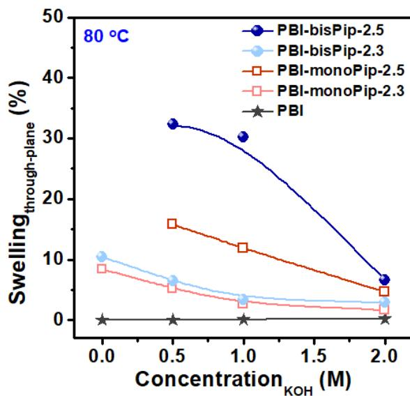
**Fig. S6** Through-plane swelling of the membranes as a function of the aq. KOH concentration.
