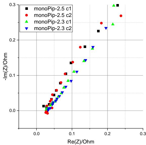
**Fig. S7.** High frequency end of the impedance spectra of the cells with the PBI-monoPip membranes. The c indicates the number of the cell.
