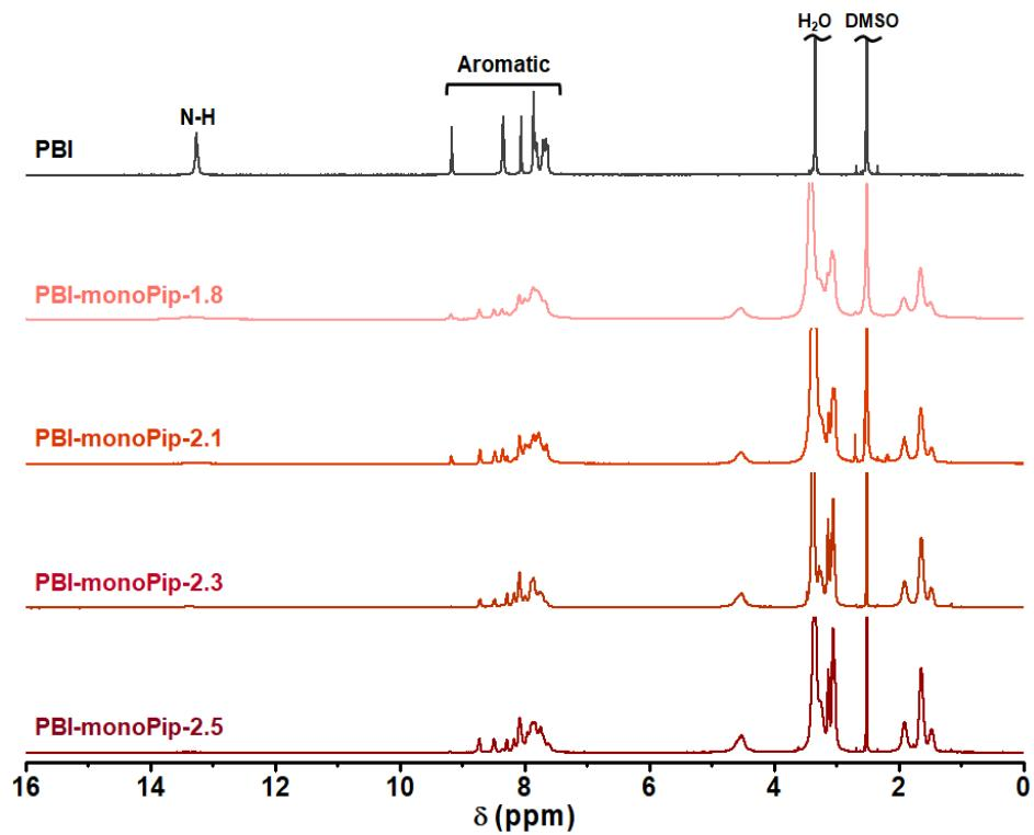
**Fig. S1** <sup>1</sup>H NMR spectra of the PBI-monoPip samples.
