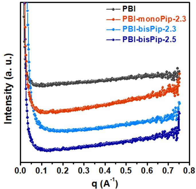
**Fig. S3** SAXS profiles of PBI and membranes in the PBI-monoPip and PBI-bisPip series.
