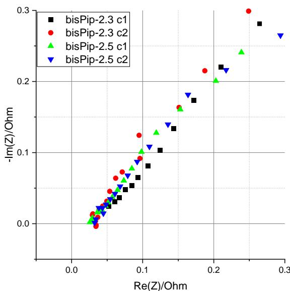
**Fig. S8.** High frequency end of the impedance spectra of the cells with the PBI-bisPip membranes before the 100 h test. The c indicates the number of the cell.
