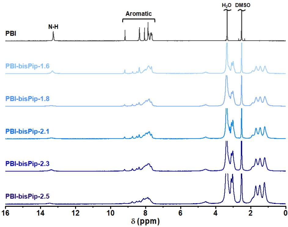
**Fig. S2** <sup>1</sup>H NMR spectra of the PBI-bisPip samples.
