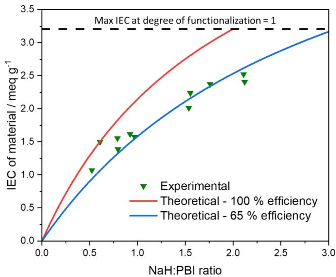
**Fig. S10** Comparison of NaH to PBI molar ratios used and the impact on the final IEC of monoPip materials. Shown are also the theoretical values for 100 % ( $DF=Ratio/2$ ) and 65 % ( $DF=0.65*Ratio/2$ ) effective reactions.
