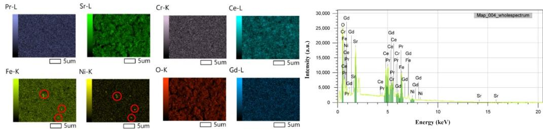
**Figure S7** SEM-EDS mapping images of the re-PSCFN<sub>0.2</sub> anode after the stability tests. The red circles represent Ni-Fe alloys.
