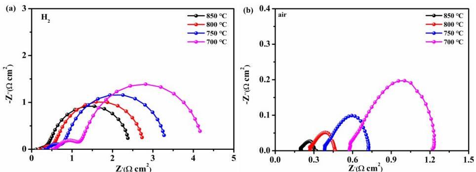
**Figure S3** The electrochemical impedance of PSCFN<sub>0.1</sub> electrode in the symmetrical half-cell in H<sub>2</sub> and air.
