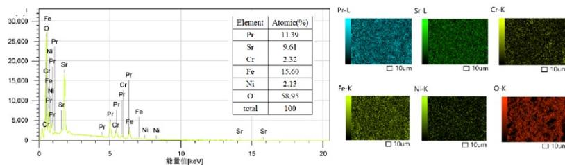
**Figure S2** SEM-EDS mappings of the PSCFN<sub>0.2</sub> powder
