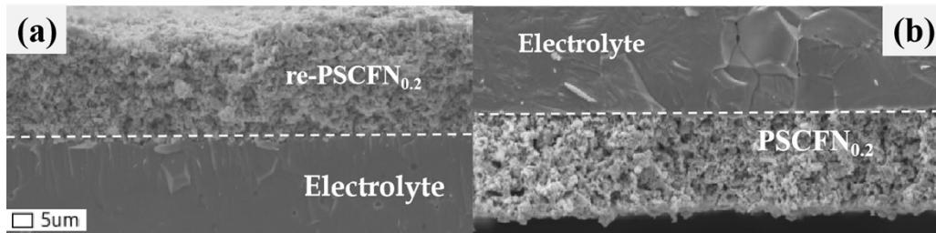
**Figure S6** SEM images of the LSGM-supported single cell with a configuration of an re-PSCFN<sub>0.2</sub> anode, LSGM electrolyte, and PSCFN<sub>0.2</sub> air electrode.
