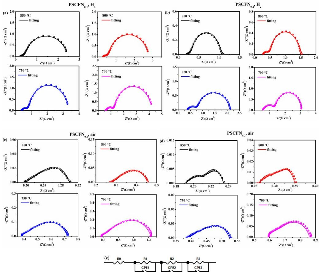
**Figure S8** (a-d) Experimental and fitting results of impedance spectra for PSCFN<sub>x</sub>/LSGM/PSCFN<sub>x</sub> symmetric half-cells at 700 °C-850 °C, (e) equivalent circuit for the impedance spectra.
