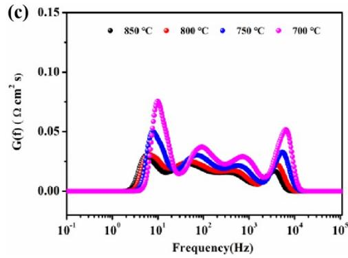
**Figure S4** (a) Typical I-V-P curves, (b) Temperature dependence of the polarization resistance ( $R_p$ ), (c) DRT analysis of the single cells with the anode (re-PSCFN<sub>0.1</sub>) fueled with H<sub>2</sub>.
