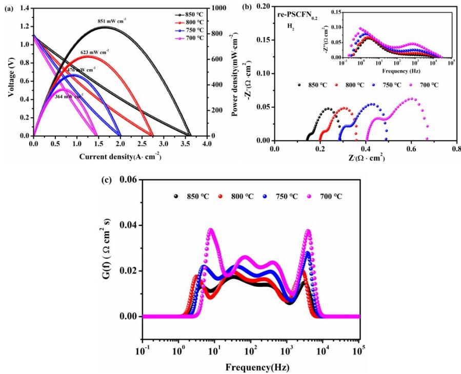
**Figure S5** (a) Typical I-V-P curves, (b) Temperature dependence of the polarization resistance ( $R_p$ ), (c) DRT analysis of the single cells with the anode (re-PSCFN<sub>0.2</sub>) fueled with H<sub>2</sub>.
