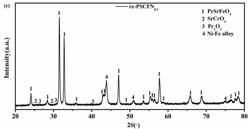
**Figure S1** (a) XRD patterns of PSCFN<sub>x</sub>, LSGM and calcined PSCFN<sub>x</sub>-LSGM mixture (1:1 mass ratio), re-PSCFN<sub>x</sub>: reduced at 850 °C for 10 h in 5% H<sub>2</sub>/Ar, (b) Rietveld XRD refinement of the PSCFN<sub>0.1</sub> powder, (c) re-PSCFN<sub>0.1</sub> powder.
