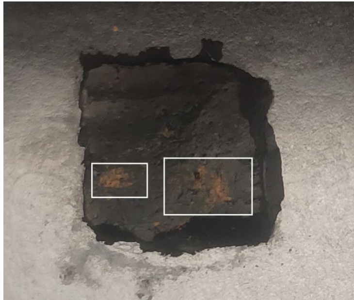
Figure S24. Photograph of the dried post-cycling slurry cathode of 0.5 M TTF battery.
