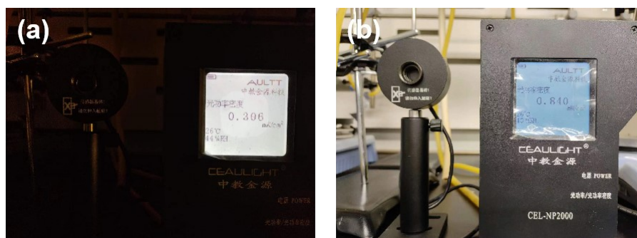
Fig S12. Images of optical intensities (a) in the darkness and (b) under ambient light through optical power meter.
