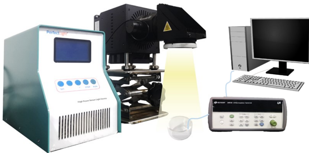
Fig. S1 Light-thermal conversion performance testing device diagram.
