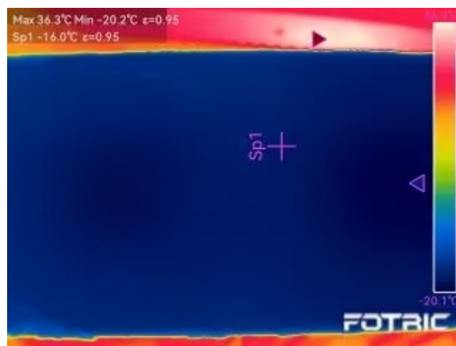
Fig. S10 Infrared thermal imaging of the cold platform surface.
