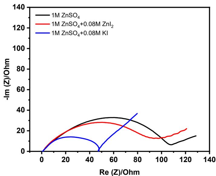
**Fig. S7** Comparative EIS curves of fabricated ZHC cells with electrolytes 1M ZnSO<sub>4</sub>, and AZHBC cells with electrolytes 1M ZnSO<sub>4</sub> + 0.08 M ZnI<sub>2</sub>, and 1M ZnSO<sub>4</sub> + 0.08 M KI.
