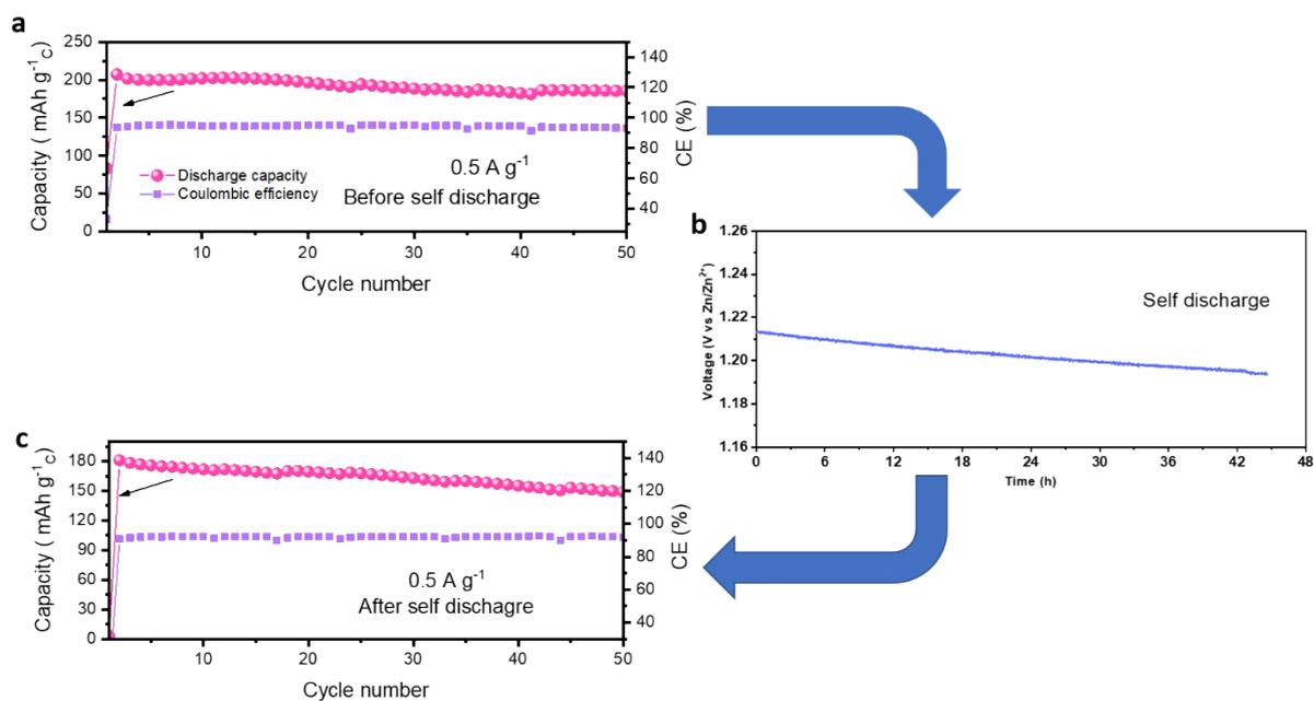
**Fig. S15** (a) Cyclic stability before self-discharge (b) self-discharge and (c) Cyclic stability after self-discharge of AZHBC in 1M ZnSO<sub>4</sub> + 0.08 M KI at 0.5 A g<sup>-1</sup>.
