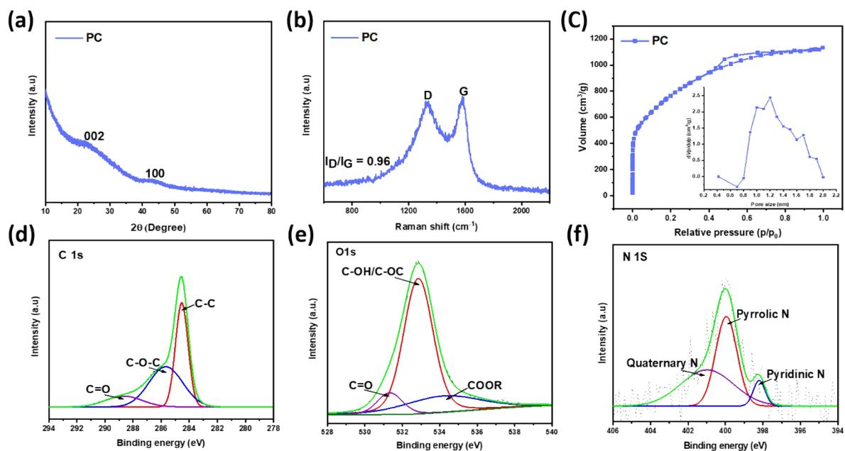
**Fig. S2** (a) XRD pattern, (b) Raman spectrum, (c) Nitrogen adsorption–desorption isotherms with pore-size distribution plot (inset), (d) XPS C1s, (e) XPS O1s, and (f) XPS N1s spectra of PC cathode.
