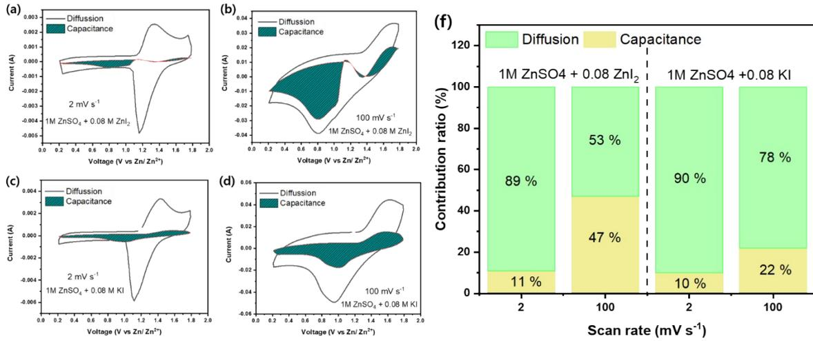
**Fig. S9** Diffusion and capacitance contribution plots of AZHBC cells with electrolytes (a & b) 1M ZnSO<sub>4</sub> + 0.08 M ZnI<sub>2</sub>, (c & d) 1M ZnSO<sub>4</sub> + 0.08 M KI and (f) bar diagram of contribution ratios at different scan rates.
