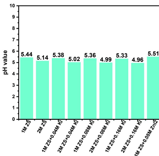
**Fig. S1** pH values of the aqueous zinc electrolytes.
