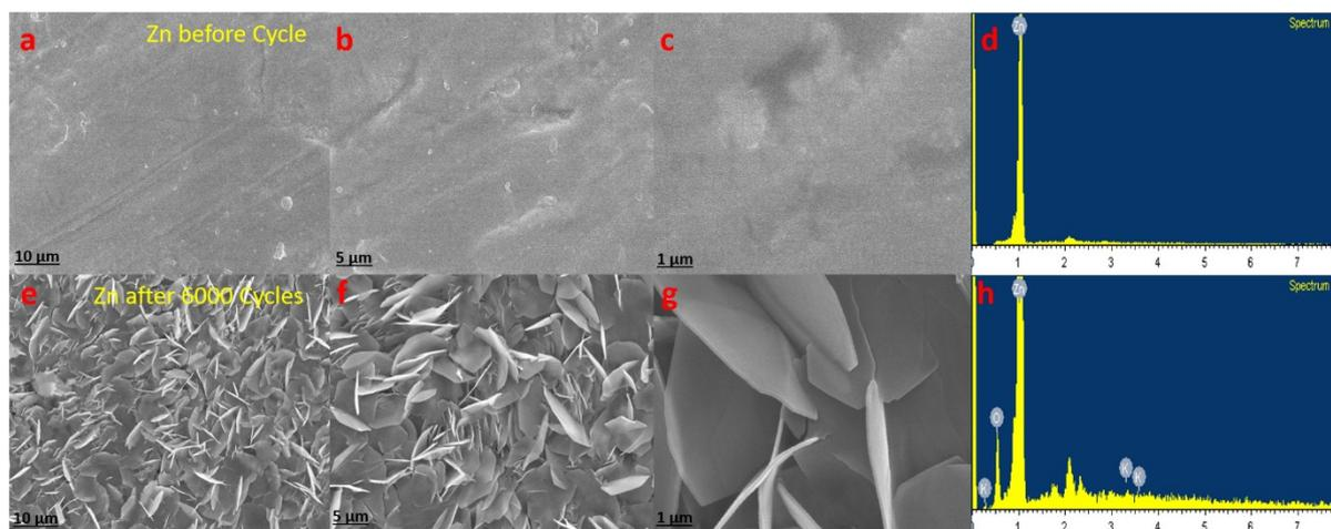
**Fig. S11** SEM images and EDAX of Zinc anode (a, b, c & d) before cycle and (e, f, g & h) after 6000 cycles in 1 M ZnSO<sub>4</sub> + 0.08 M KI.
