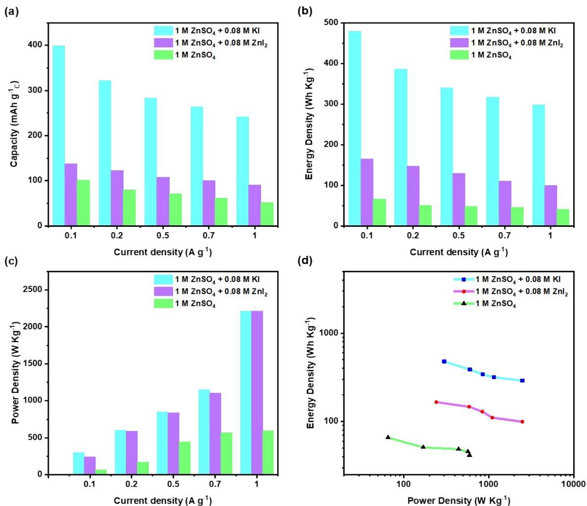
**Fig. S6** (a) Specific capacities, (b) Energy densities, (c) Power densities at current densities from 0.1 to 1 A g<sup>-1</sup> and (d) Rangone plots of ZHC cells with electrolyte 1M ZnSO<sub>4</sub>, and AZHBC cells with electrolytes 1M ZnSO<sub>4</sub> + 0.08 M ZnI<sub>2</sub>, and 1M ZnSO<sub>4</sub> + 0.08 M KI respectively.
