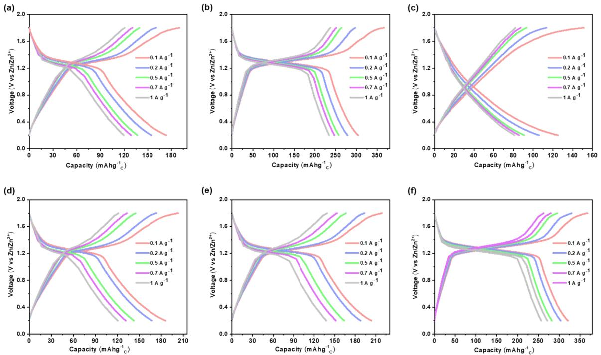
**Fig. S10** GCD curves of fabricated AZHBC cells at different current densities (0.1, 0.2, 0.5, 0.7, and 1 A g<sup>-1</sup>) in (a) 1 M ZnSO<sub>4</sub> + 0.04 M KI, (b) 1 M ZnSO<sub>4</sub> + 0.16 M KI, (c) 2 M ZnSO<sub>4</sub>, (d) 2 M ZnSO<sub>4</sub> + 0.04 M KI, (e) 2 M ZnSO<sub>4</sub> + 0.08 M KI, and (f) 2 M ZnSO<sub>4</sub> + 0.16 M KI electrolyte solutions, respectively.
