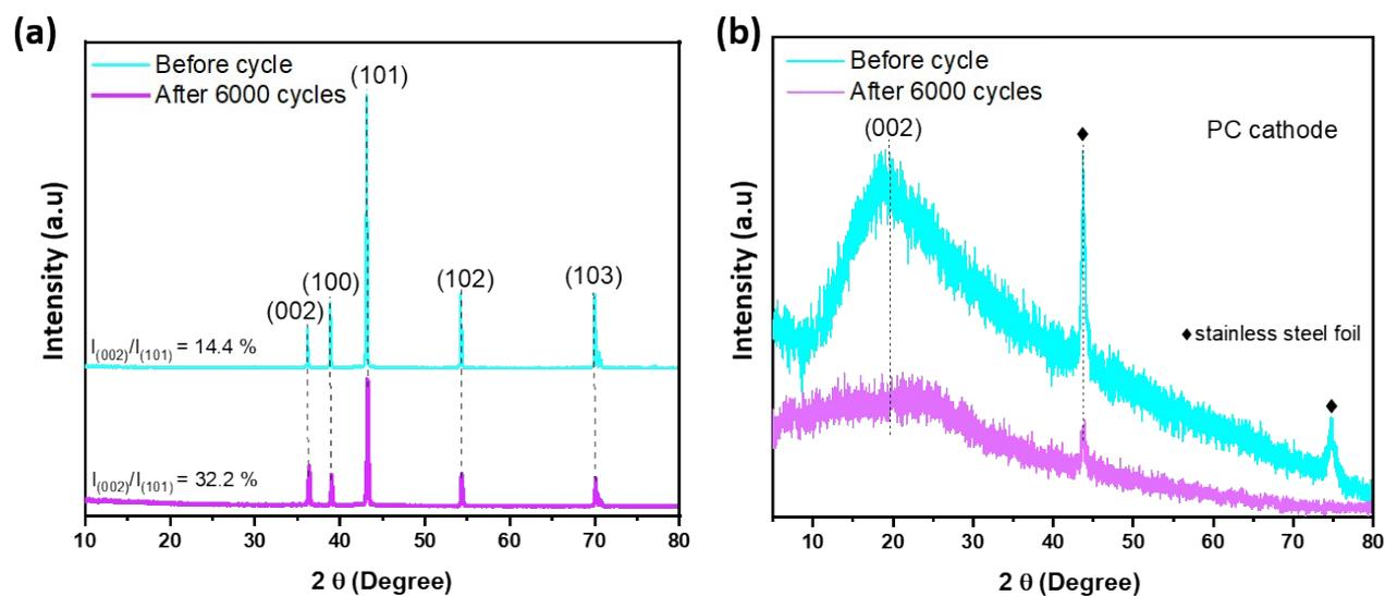
**Fig. S12** XRD of (a) Zinc anodes, (b) PC cathodes before and after cycling.
