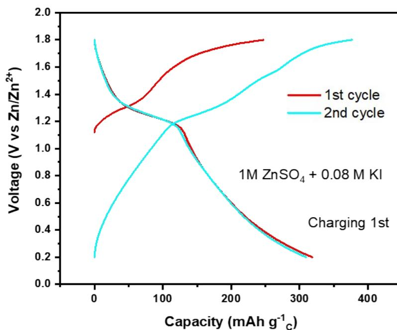
**Fig. S5** Initial charge/discharge curves of fabricated AZHBC cells with electrolytes 1M ZnSO<sub>4</sub> + 0.08 M KI at a current density of 0.1 A g<sup>-1</sup>.
