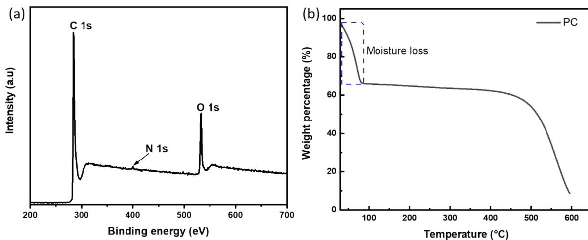
**Fig. S3** (a) XPS survey spectrum and (b) TGA of PC.
