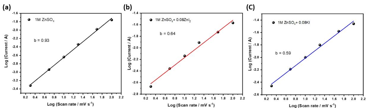
**Fig. S8** Linear fit of  $\log(v)$  and  $\log(i)$  of fabricated ZHC cells with electrolytes (a) 1M ZnSO<sub>4</sub>, and AZHBC cells with electrolytes (b) 1M ZnSO<sub>4</sub> + 0.08 M ZnI<sub>2</sub>, and (c) 1M ZnSO<sub>4</sub> + 0.08 M KI.
