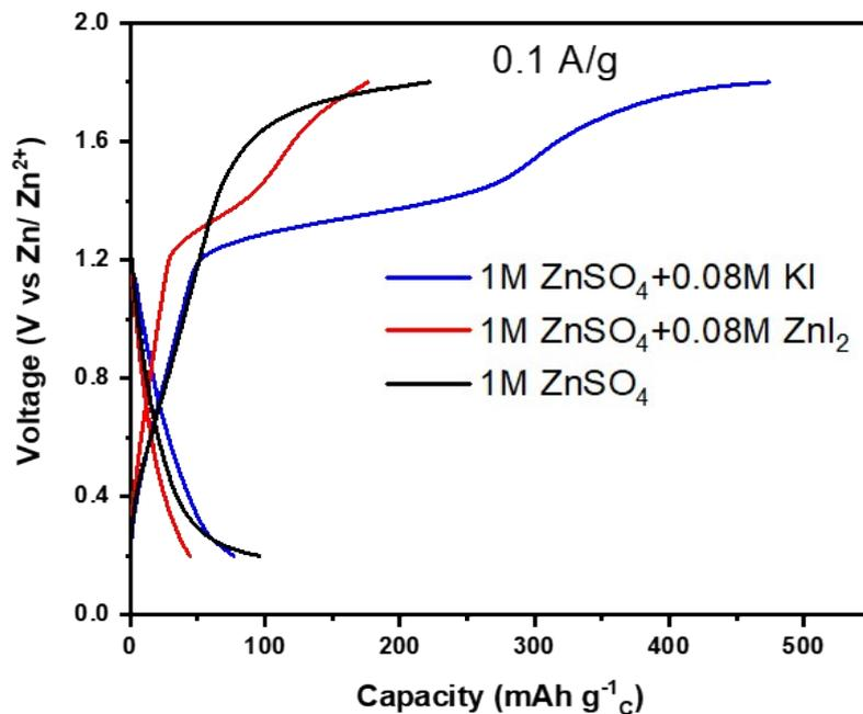
**Fig. S4** Comparative initial discharge/charge curves of fabricated ZHC cell with electrolytes 1M ZnSO<sub>4</sub>, and AZHBC cells with electrolytes 1M ZnSO<sub>4</sub> + 0.08 M ZnI<sub>2</sub>, and 1M ZnSO<sub>4</sub> + 0.08 M KI at a current density of 0.1 A g<sup>-1</sup>.
