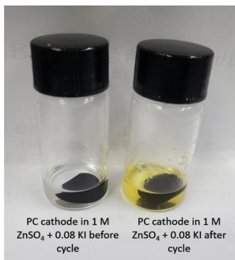
**Fig. S13** Color change of electrodes immersed in fresh KI electrolyte (a) before and (b) after complete charging to confirm the presence of I<sub>3</sub><sup>-</sup>.
