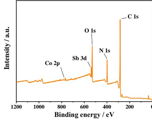
**Figure S4.** XPS survey spectrum of NC@CoSb/CNTs-400.
