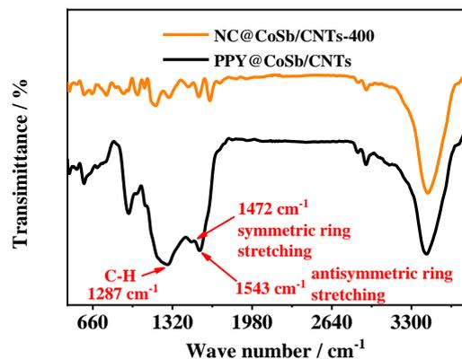
**Figure S1.** FTIR spectra of PPY@CoSb/CNTs and NC@CoSb/CNTs-400.
