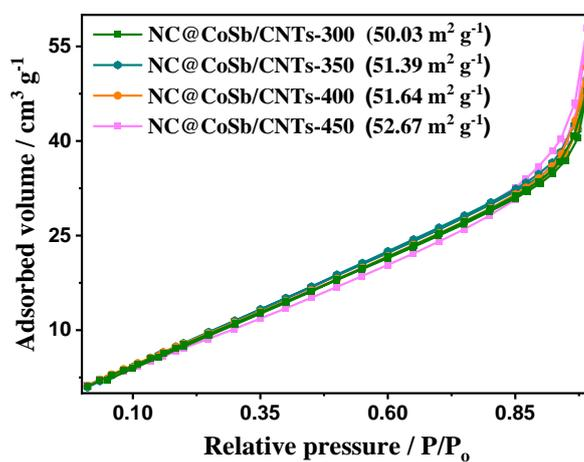
**Figure S11.** N<sub>2</sub> adsorption/desorption isotherms of NC@CoSb/CNTs-300, NC@CoSb/CNTs-350, NC@CoSb/CNTs-400 and NC@CoSb/CNTs-450. The BET specific surface areas of the samples are given in the brackets.
