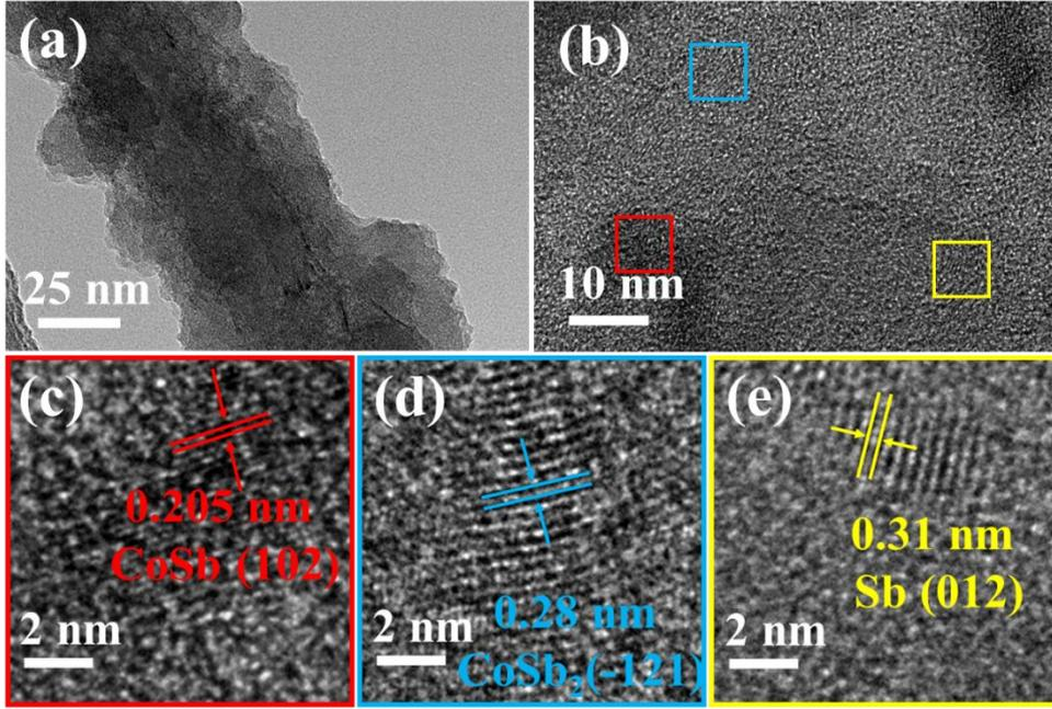
**Figure S12.** (a) TEM and (b) HRTEM images of NC@CoSb/CNTs-450. (c), (d) and (e) magnified HRTEM images of CoSb/CNTs indicated in (b).
