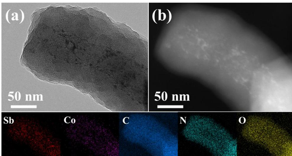
**Figure S10.** (a) TEM and (b) Elemental mapping images of the NC@CoSb/CNTs-400 after 500 cycles.
