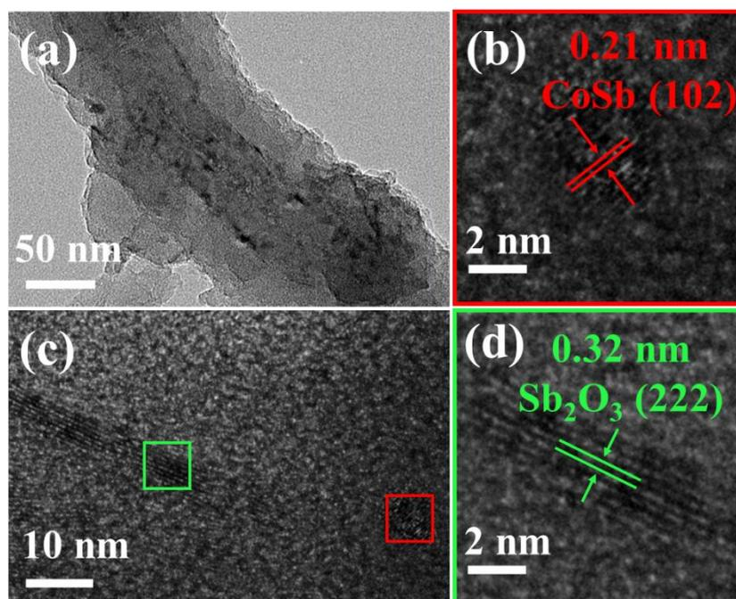
**Figure S9.** (a) TEM and (c) HRTEM images of NC@CoSb/CNTs-300. (b) and (d) magnified HRTEM images of CoSb/CNTs indicated in (c).
