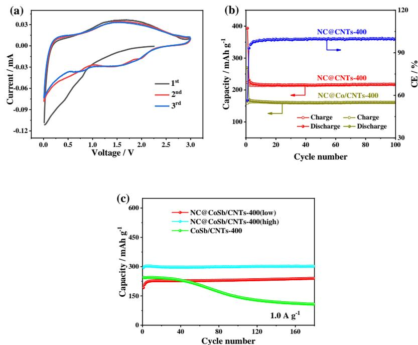
**Figure S8.** (a) CV curves of NC@CNTs-400. (b) Cycling performance of NC@CNTs-400 and NC@Co/CNTs-400 at 0.1 A g<sup>-1</sup>. (c) Cycling performance of CoSb/CNTs-400, NC@CoSb/CNTs-400(low), and NC@CoSb/CNTs-400(high) at 1.0 A g<sup>-1</sup>.
