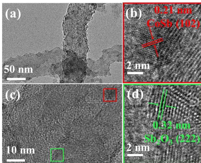
**Figure S7.** (a) TEM image and (c) HRTEM images of CoSb/CNTs. (b) and (d) magnified HRTEM images of CoSb/CNTs indicated in (c).
