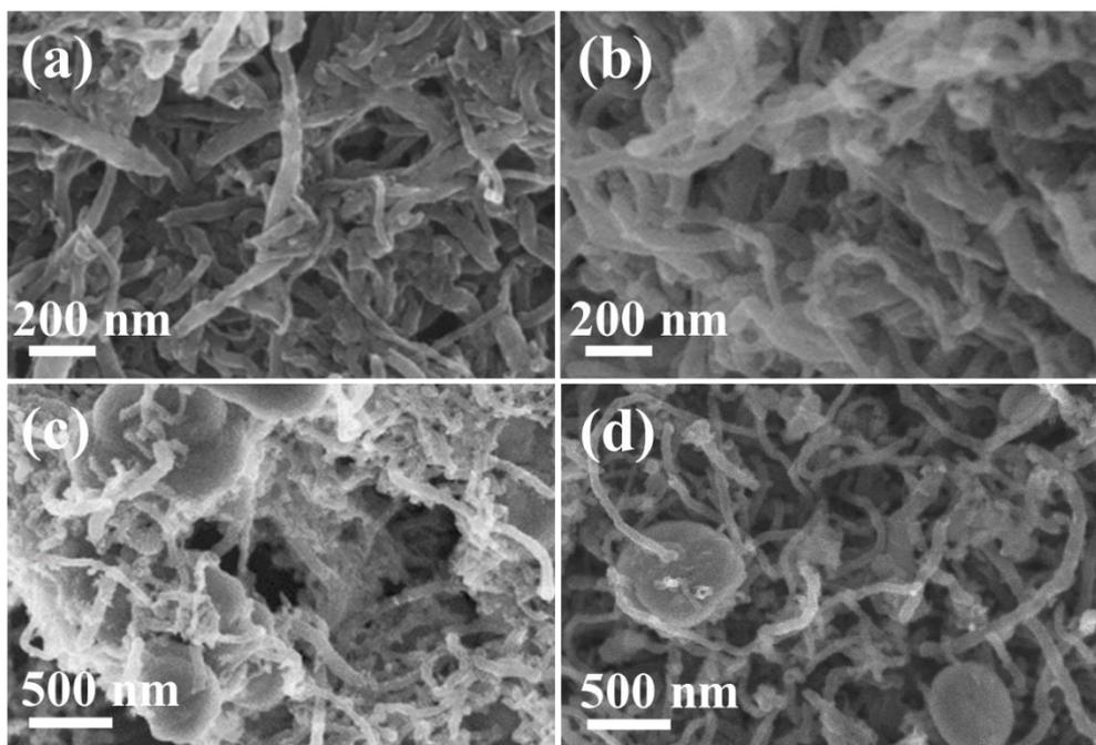
**Figure S6.** SEM images of (a) Sb<sub>2</sub>O<sub>3</sub>/CNTs, (b) Co/CNTs, (c) CoSb/CNTs (high) and (d) CoSb/CNTs-400.
