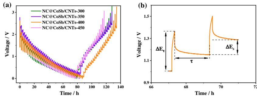
**Figure S13.** (a) GITT profiles of the discharge/charge process. (b) Schematic illustration of  $\Delta E_s$  and  $\Delta E_\tau$  used for the calculation.
