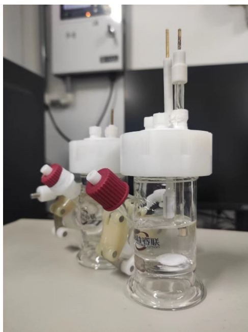
Figure S13. The sealed H-type electrolytic cell is used for the determination of gaseous products.
