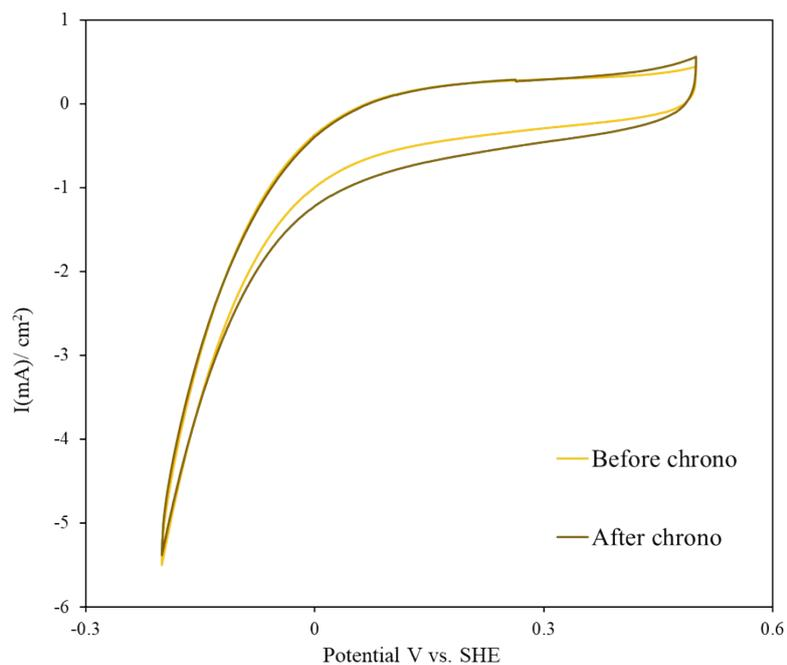
**Figure S15:** CV before and after the 12 h of chronoamperometry test with an applied voltage of -0.150V vs. RHE for the prepared WS<sub>2</sub>/C catalyst indicates that the catalyst is stable even after a long duration of hydrogen production.
