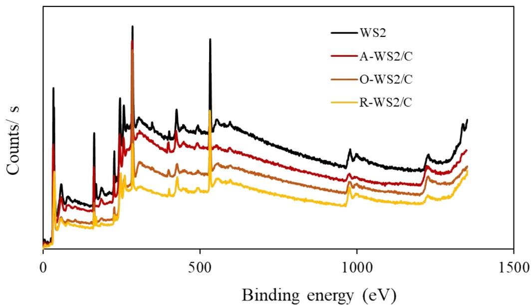
**Figure S6:** Full XPS spectrum of the WS<sub>2</sub>, A-WS<sub>2</sub>/C, O-WS<sub>2</sub>/C, R-WS<sub>2</sub>/C.
