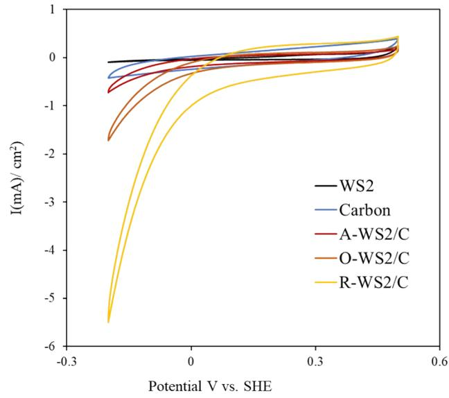
**Figure S11:** CV for all the samples in 0.5 M H<sub>2</sub>SO<sub>4</sub>.
