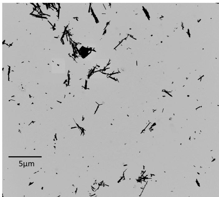
**Figure S1:** Low magnification STEM image of WS<sub>2</sub> NTs/carbon composite showing the NTs are well dispersed throughout the grid.
