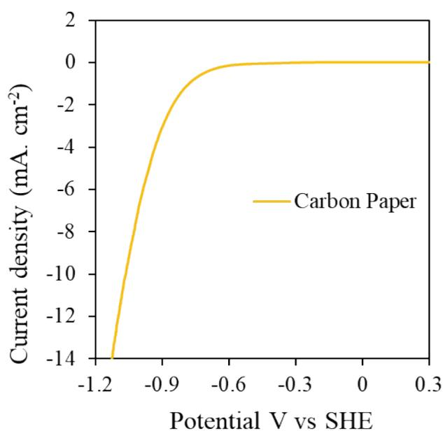
**Figure S10:** LSVs of the Toray carbon paper showing a negligible effect on the catalytic performance.
