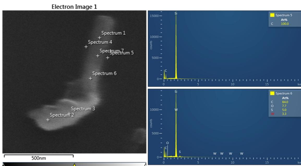
**Figure S2:** *left.* Low voltage SEM image of the carbon-coated WS<sub>2</sub> tube on silicon wafer. *Right.* EDS analysis of different points on the nanotube shown, revealing 100% carbon adjacent to the wall of the tube (point #5) as compared to elements content in the middle of the tube (point #6). The high content carbon proves that the carbon efficiently wraps all over the nanotube.
