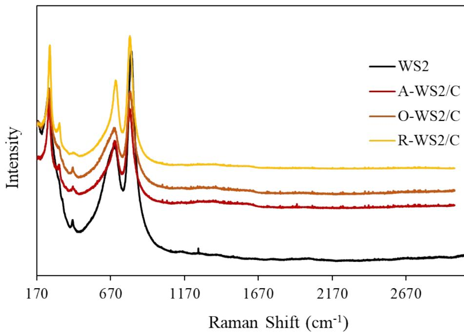
**Figure S5:** Raman spectroscopy of the WS<sub>2</sub>/C composites.
