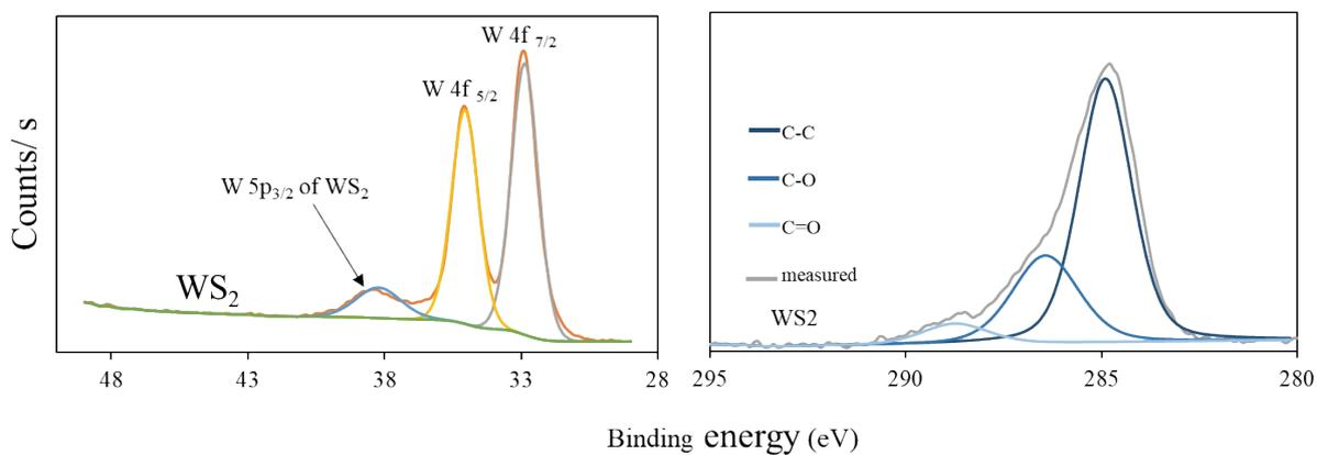
**Figure S8:** XPS spectrum of pristine WS<sub>2</sub> after peak splitting of W<sub>4f</sub> and C<sub>1s</sub> scan.
