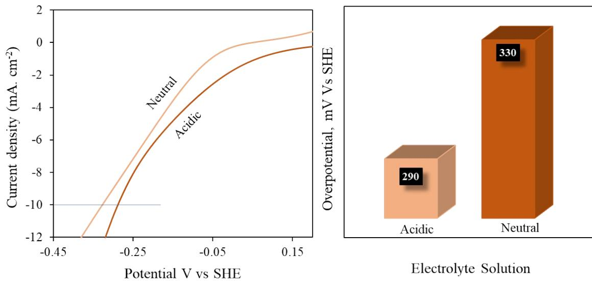
**Figure S12:** Onset potential at a current density of  $-10 \text{ mAcm}^{-2}$  of O-WS<sub>2</sub>/C at acidic and neutral solutions.
