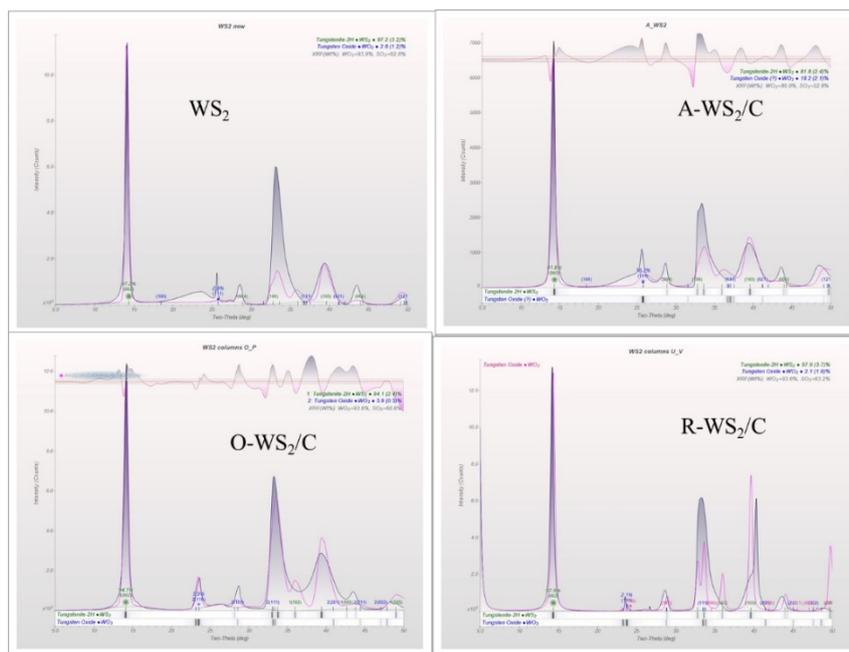
Figure S3. XRD analysis of three different samples with pristine WS<sub>2</sub> shows the presence of WO<sub>2</sub> oxide phase in pristine and first annealed (A-WS<sub>2</sub>/C) sample whereas the other two samples (O-WS<sub>2</sub>/C AND R-WS<sub>2</sub>/C) contain WO<sub>3</sub> phase. Importantly, for every sample WS<sub>2</sub> (002) peak at 2 $\theta$ =14.5 remains a higher percentage proving the unharmed crystallinity.
