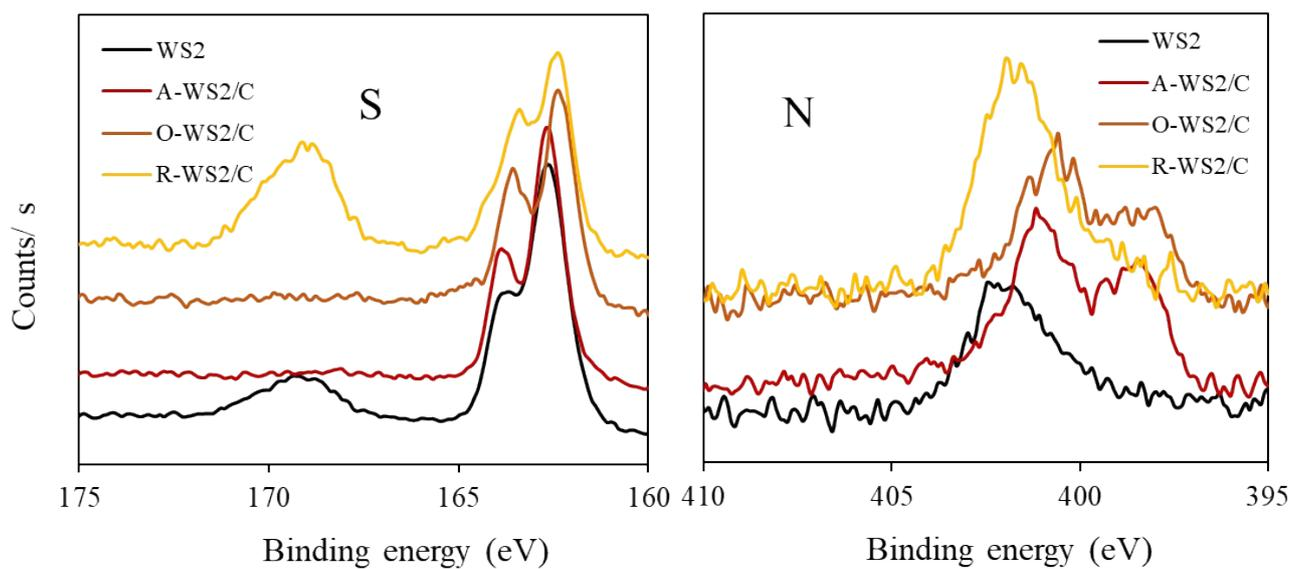
**Figure S7:** XPS of S<sub>2p</sub> and N<sub>1s</sub> for all samples.
