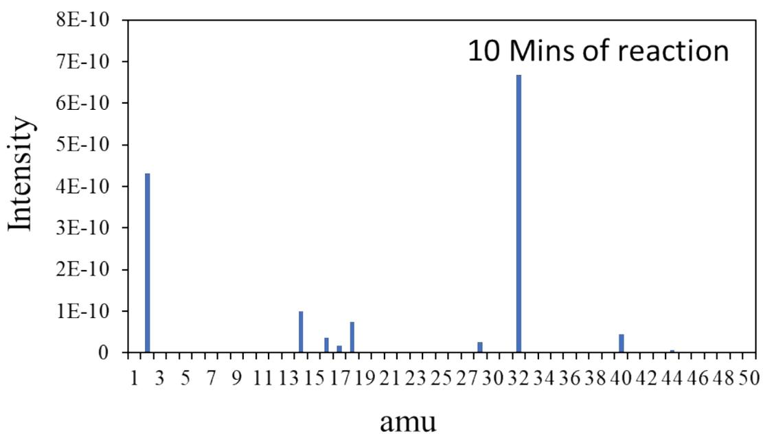
**Figure S9.** Mass spectroscopy (MS) was collected from A-WS2/C after 10 minutes of CA at its overpotential, confirming hydrogen production.
