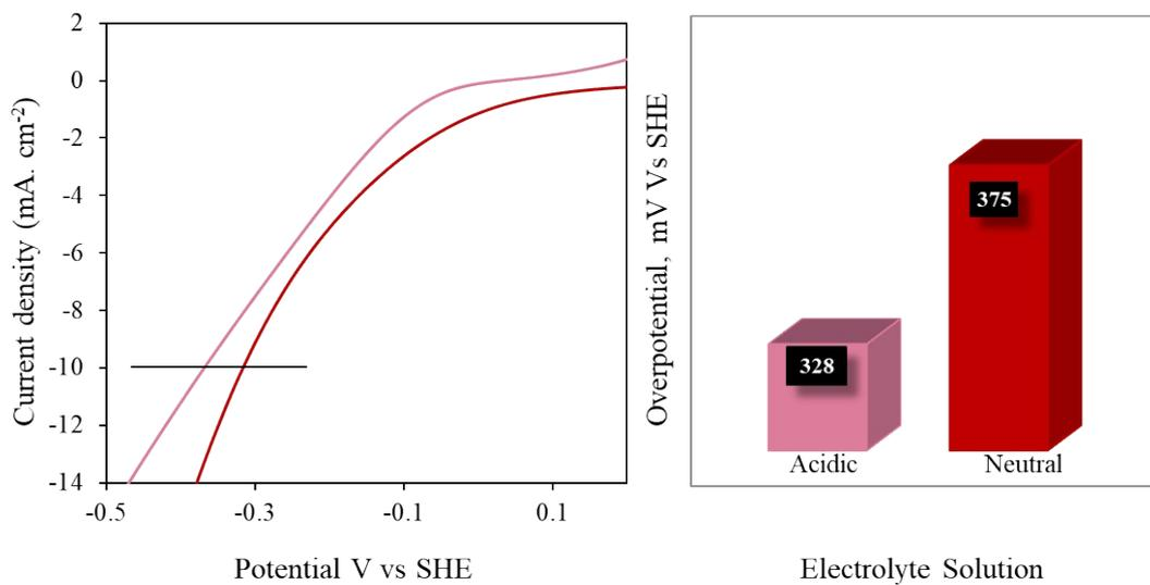
**Figure S13:** Onset potential at a current density of  $-10 \text{ mA cm}^{-2}$  of A-WS<sub>2</sub>/C at acidic and neutral solutions
