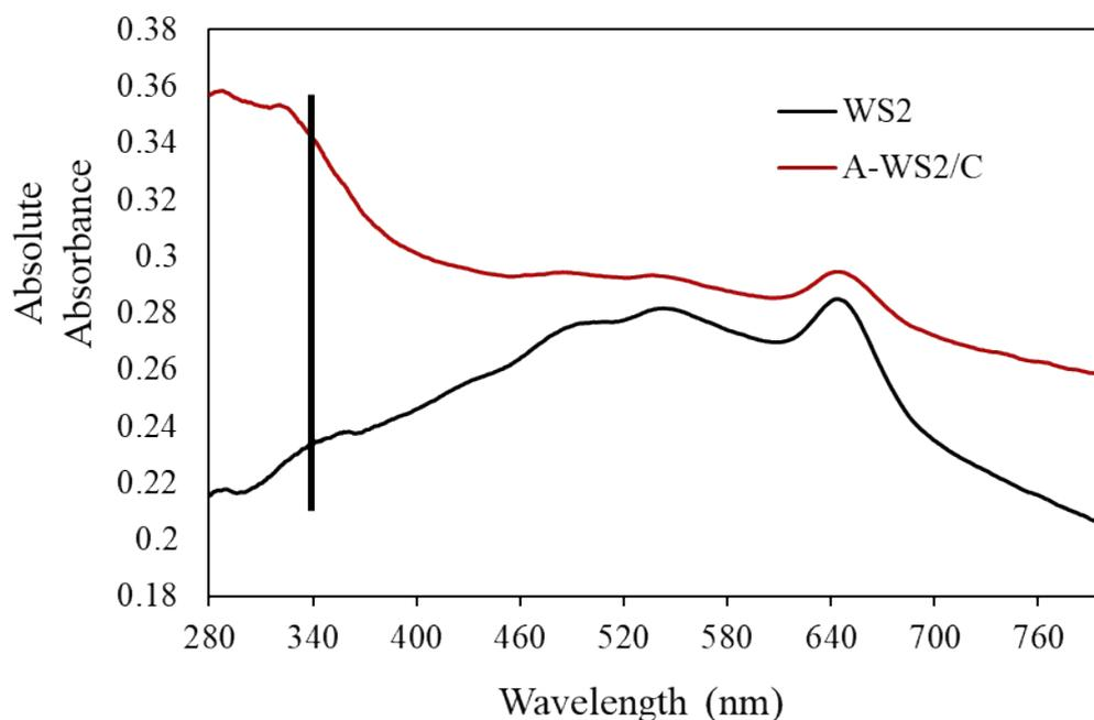
**Figure S4:** Absolute absorption spectra of prepared A-WS<sub>2</sub>/C showing no shift at the exciton of the nanotube. An additional peak near 340 nm appears due to the attachment of carbon with the nanotube.
