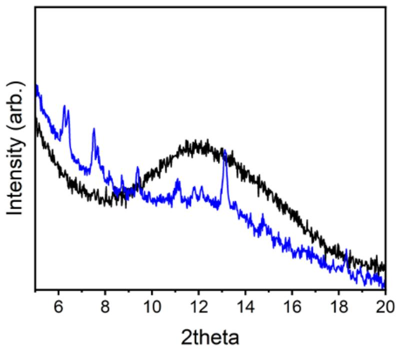
Figure S13. Grazing incidence diffraction patterns of black: HKUST-1 solvothermally grown on ppgNH<sub>2</sub> modified surface after click reaction with azide gold surface; and blue: HKUST-1 nanoparticles introduced to ppgNH<sub>2</sub> modified surface after synthesis.
