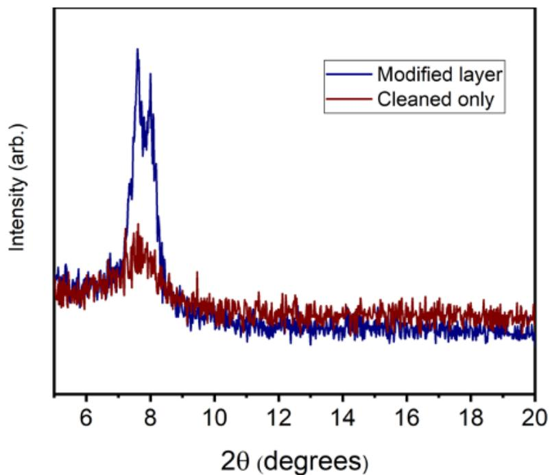
Figure S14. PXRD patterns of Co 5-ppg calixarene cage crystallized out of DMF on top of a cleaned, unmodified surface (red), and on an azide-modified surface after a click reaction with Co 5-ppg calixarene cage (blue).
