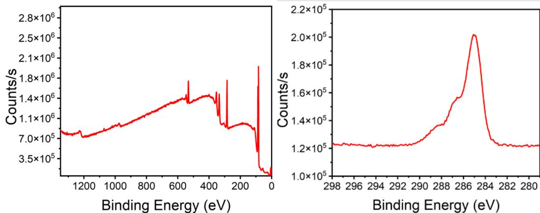
Figure S4. XPS survey spectra and high resolution C spectra for carboxylate modified gold surface.
