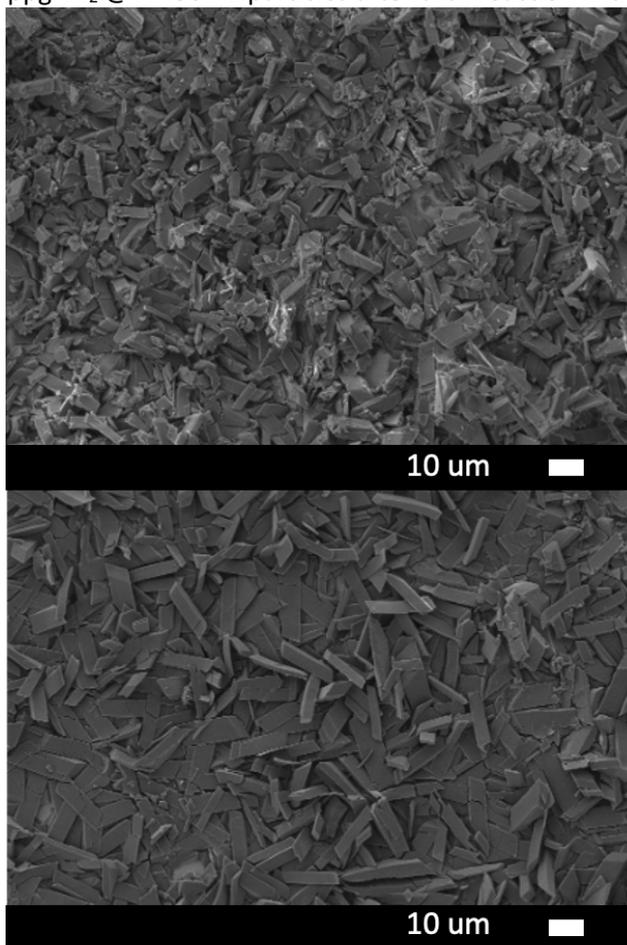
Figure S30. SEM image of Co 5-ppg calixarene cage crystallized out of DMF on top of a clean, unmodified gold surface (top), and on top of an azide modified surface after click reaction with Co 5-ppg calixarene cage (bottom.)
