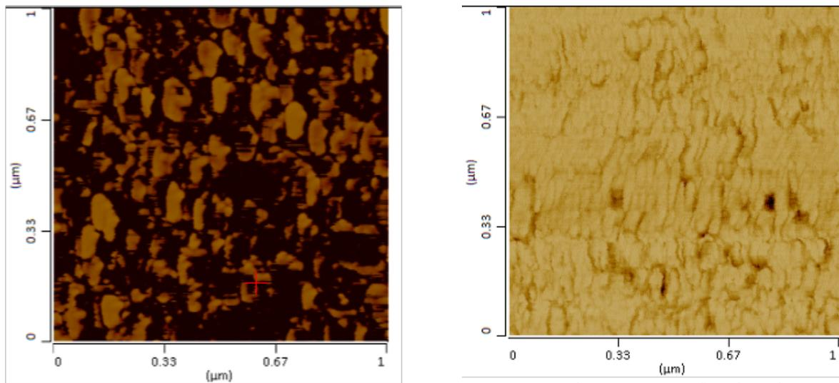
Figure S43. AFM phasing maps of carboxylate modified surface before (left), and after (right) ion exchange reaction with Zr diMe OTf cage.
