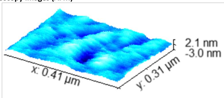
Figure S34. AFM image of cleaned gold surface.
