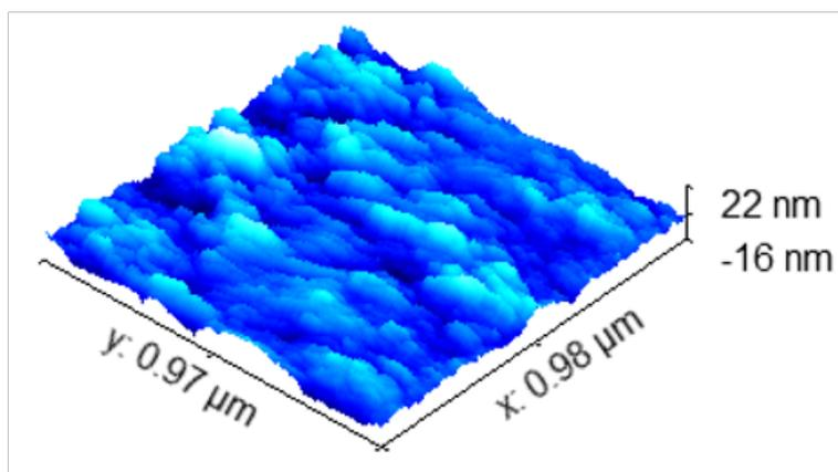
Figure S42. AFM image of carboxylate modified surface following ion exchange reaction with Zr diMe OTf cage.
