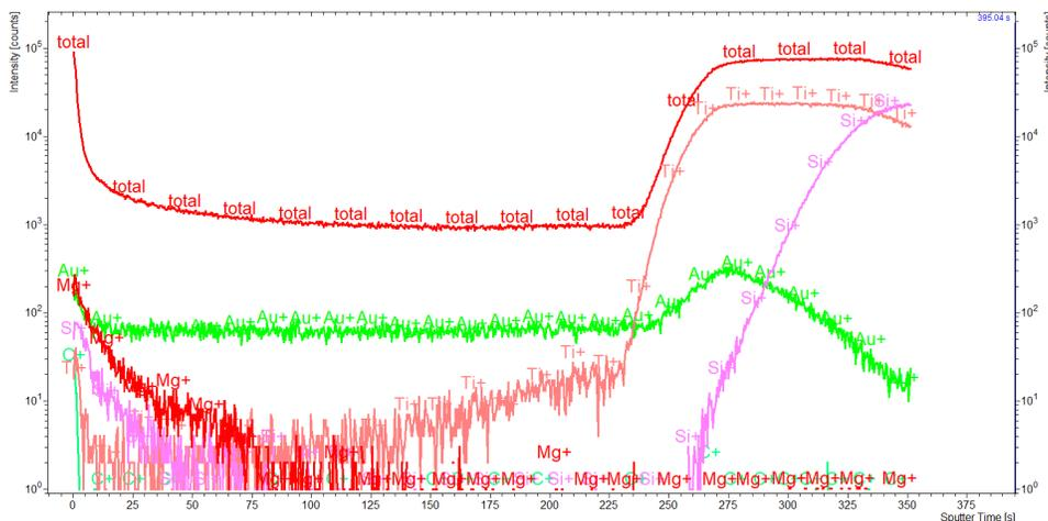
Figure S23. Depth profile of bromide functionalized surface after SN2 reaction with Mg 5-OH calixarene cage. Traces of note include, red corresponding to Mg, & green corresponding to Au. Etching was carried out using an O<sub>2</sub><sup>+</sup> sputter source.
