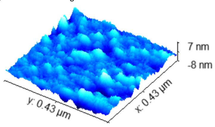
Figure S36. AFM image of bromide modified gold surface.
