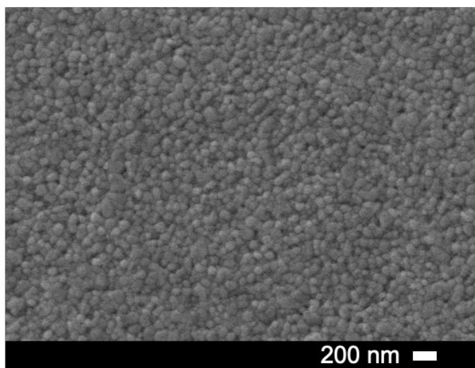
Figure S32. SEM image of bromide modified surface following SN<sub>2</sub> reaction with Mg 5-OH calixarene cage.
