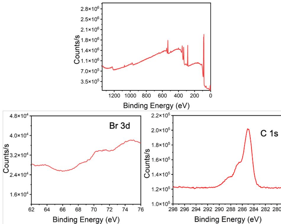
Figure S3. XPS survey spectra and high resolution C & Br spectra for bromide modified gold surface.
