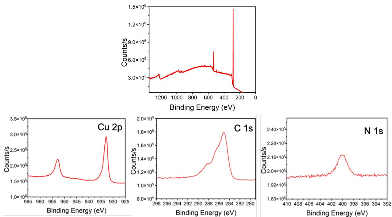
Figure S5. XPS survey spectra and high resolution C, N, & Cu for azide modified surface following click reaction with ppgNH<sub>2</sub>@HKUST-1.
