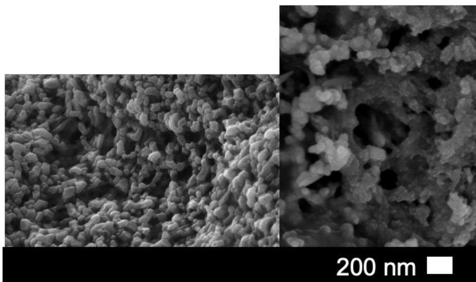
Figure S27. SEM image of HKUST-1 (left) and ppgNH<sub>2</sub> @ HKUST-1 particles (right.)
