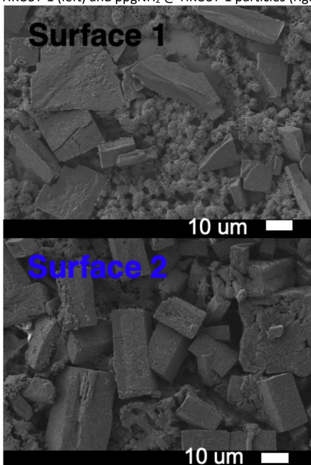
Figure S28. SEM image of HKUST-1 solvothermally grown on ppgNH<sub>2</sub> modified surface after click reaction with azide gold surface (surface 1); and HKUST-1 nanoparticles introduced to ppgNH<sub>2</sub> modified surface after synthesis (surface 2.)
