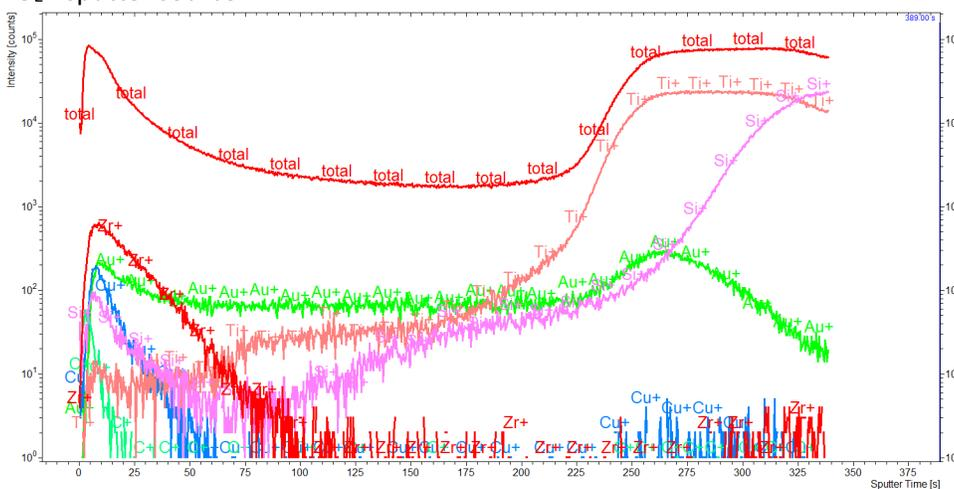
Figure S24. Depth profile of carboxylate functionalized surface after ion exchange reaction with Zr diMe OTf cage. Traces of note include, red corresponding to Zr, & green corresponding to Au. Etching was carried out using an O<sub>2</sub><sup>+</sup> sputter source.
