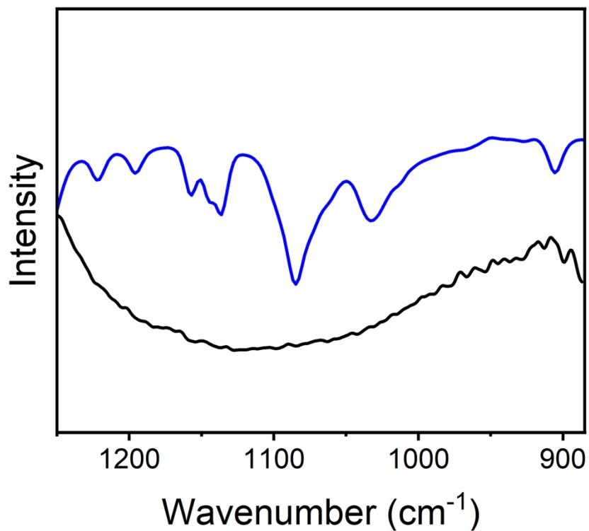
Figure S46. NanoIR spectra of Mg 5-OH calixarene cage on bromide modified gold surface (black) stacked with Mg 5-OH calixarene cage bulk IR spectra (blue).
