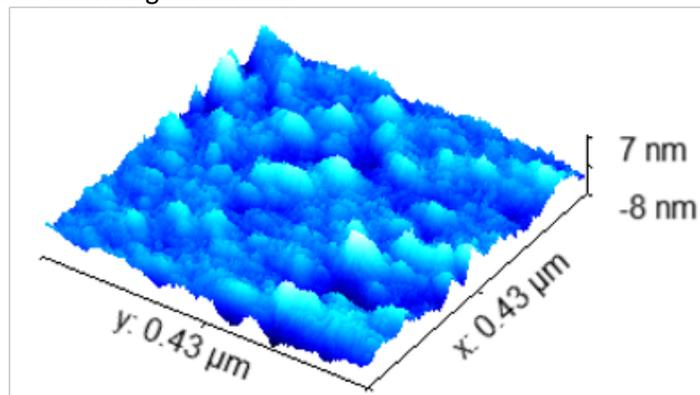
Figure S35. AFM image of azide modified gold surface.
