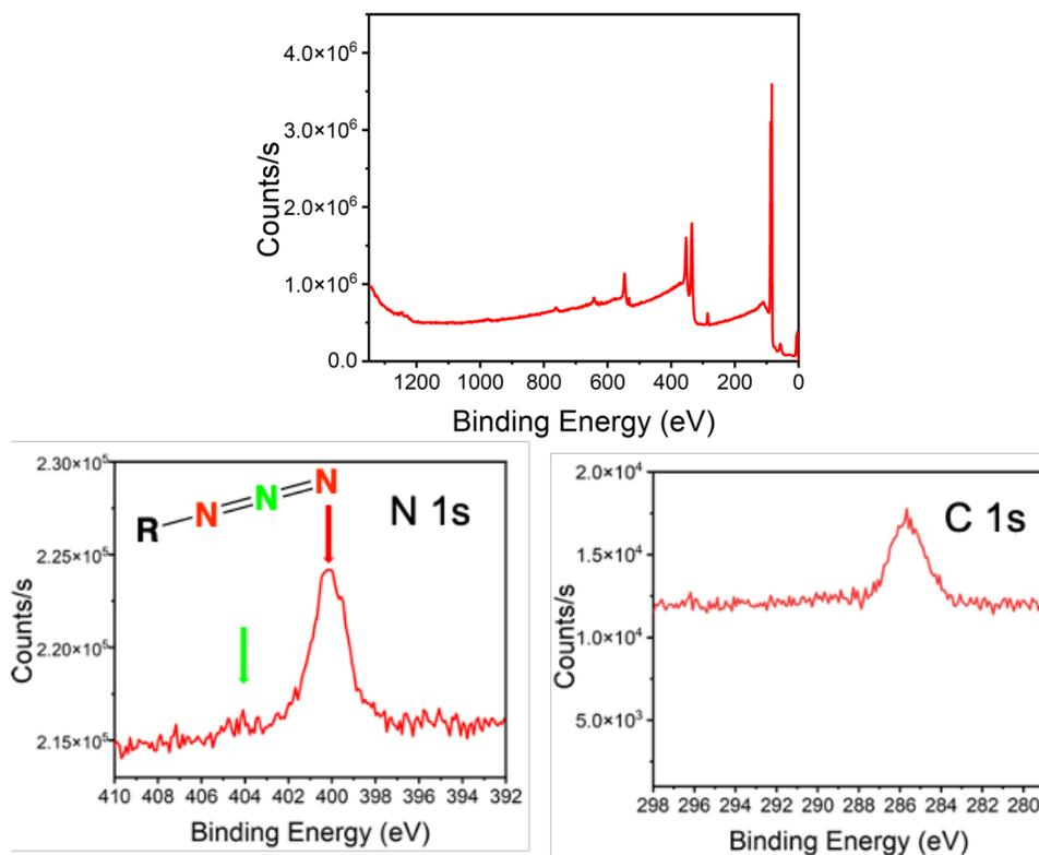
Figure S2. XPS survey spectra and high resolution C & N spectra for azide modified gold surface.
