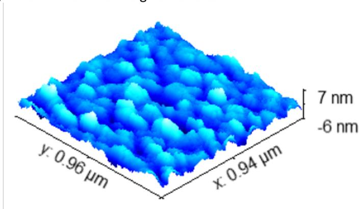
Figure S37. AFM image of carboxylate modified gold surface.
