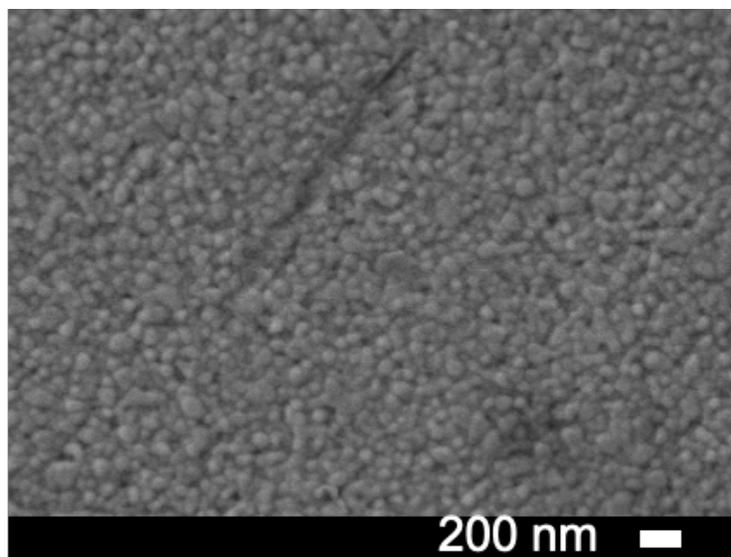
Figure S29. SEM image of ppgNH<sub>2</sub> @ HKUST-1 particles after click reaction with azide-modified surface.
