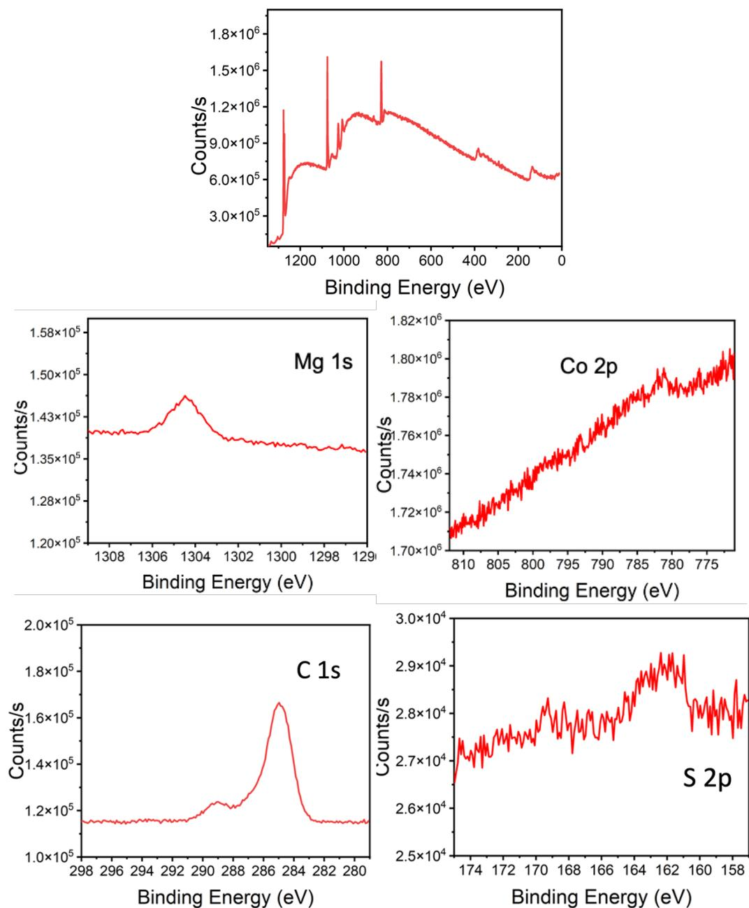
Figure S7. XPS survey spectra and high resolution Mg, Co, C, & S spectra for Co 5-ppg calixareneppg cage after click reaction with azide modified gold surface followed by click reaction with Mg 5-N3 calixarene cage.
