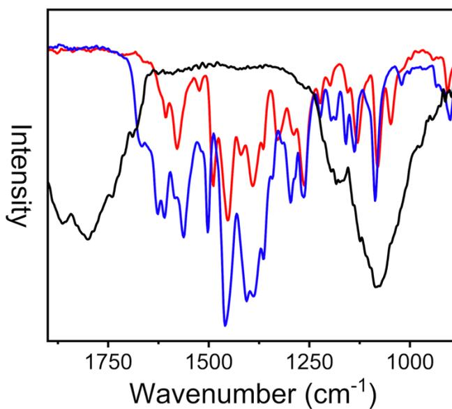
Figure S45. NanoIR spectra of clicked Co 5-ppg calixarene cage on azide modified gold surface followed by clicked Mg 5-N3 calixarene cage (black) stacked Co 5-ppg calixarene (red) and Mg 5-N3 calixarene (blue) bulk IR spectra.
