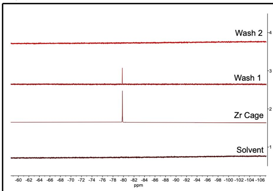
Figure S10.  $^{19}\text{F}$  NMR spectra of MeOD (bottom), Zr diMe OTf cage in MeOD (second bottom), MeOD wash 1 after ion exchange reaction with surface (second top), and wash 2 after ion exchange reaction with surface (top).
