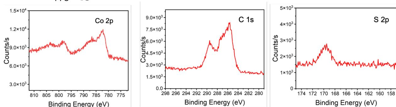
Figure S6. XPS survey spectra and high resolution C, Co, & S spectra for Co 5-ppg calixarene cage after click reaction with azide modified gold surface.
