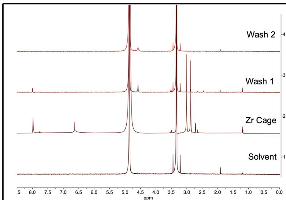
Figure S11.  $^1\text{H}$  NMR spectra of MeOD (bottom), Zr diMe OTf cage in MeOD (second bottom), MeOD wash 1 after ion exchange reaction with surface (second top), and wash 2 after ion exchange reaction with surface (top).
