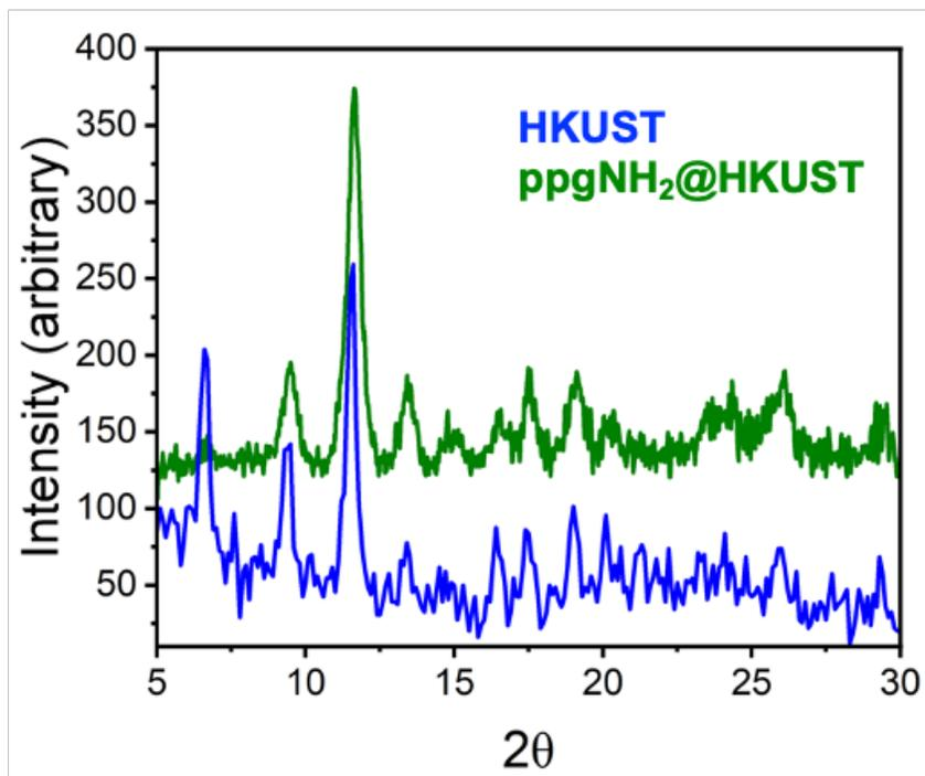
Figure S12. Stacked PXRD patterns of HKUST 1 nanoparticles (blue) and ppgNH<sub>2</sub>@HKUST-1 (green.)
