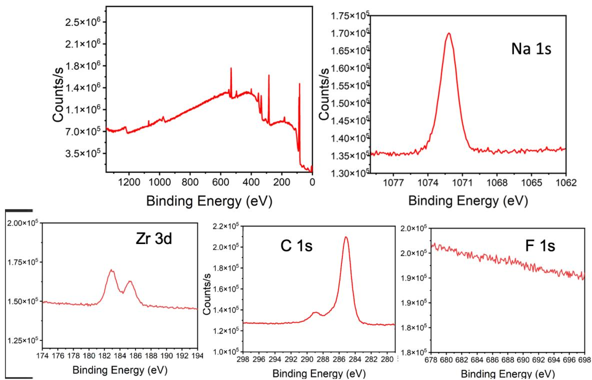
Figure S9. XPS survey spectra and high resolution Na, Zr, C, & F spectra for Zr diMe OTf cage after ion exchange reaction with carboxylate modified gold surface.
