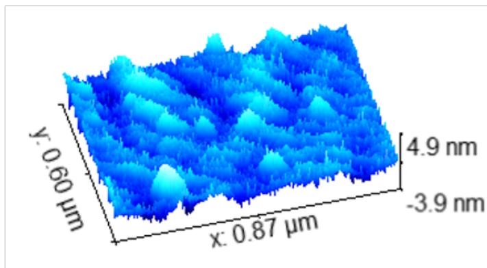
Figure S39. AFM image of azide modified surface following click reaction with Co 5-ppg calixarene cage.
