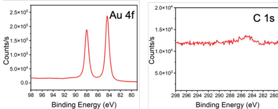
Figure S1. XPS high resolution Au & C spectra for cleaned gold surface.
