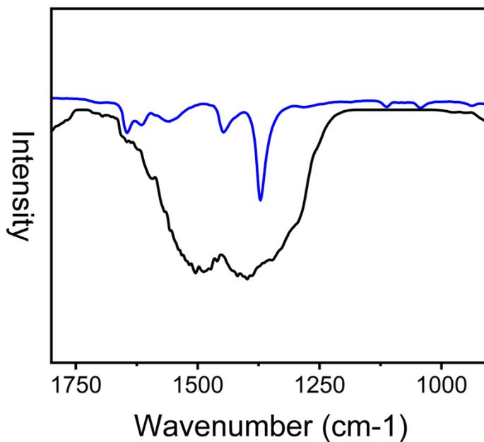
Figure S44. NanoIR spectra of ppgNH<sub>2</sub> @ HKUST-1 on azide modified gold surface stacked with ppgNH<sub>2</sub> @ HKUST-1 bulk IR spectra.
