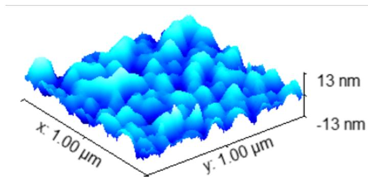
Figure S41. AFM image of bromide modified surface following SN2 reaction with Mg 5-OH calixarene cage.
