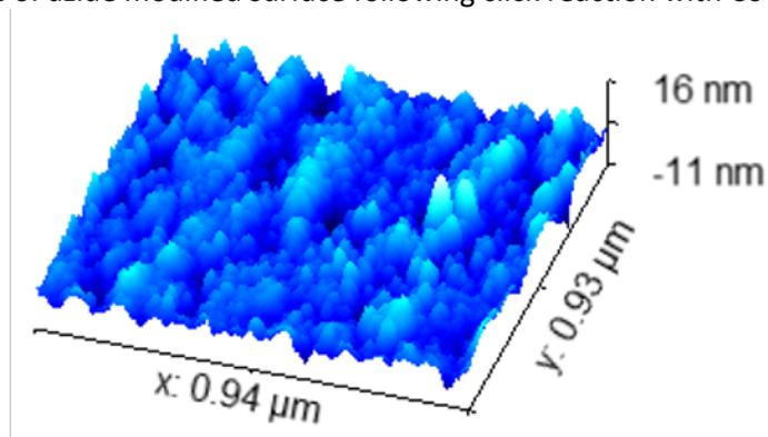
Figure S40. AFM image of azide modified surface following click reaction with Co 5-ppg calixarene cage followed by Mg 5-N3 calixarene cage.
