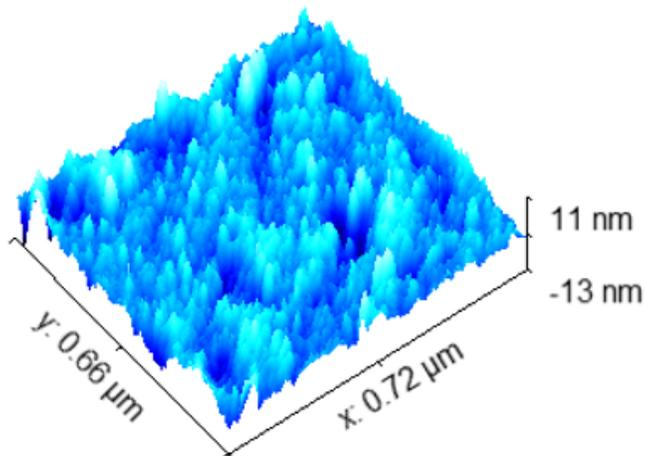
Figure S38. AFM image of azide modified surface following click reaction with ppgNH<sub>2</sub> @ HKUST-1 particles.
