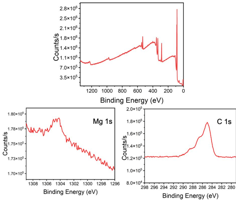
Figure S8. XPS survey spectra and high resolution Mg & C spectra for Mg 5-OH calixarene cage after SN2 reaction with bromide modified gold surface.
