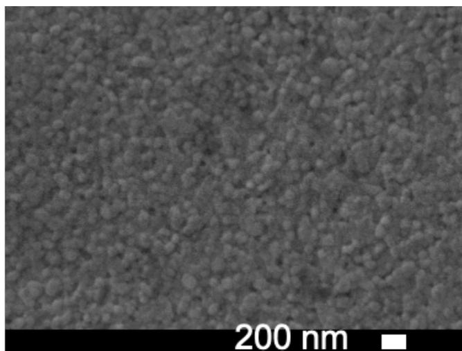
Figure S33. SEM image of carboxylate modified surface following an ion exchange reaction with Zr diMe OTf cage.
