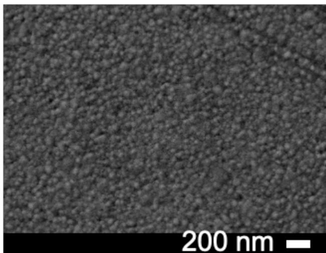
Figure S31. SEM image of azide modified surface following click reaction with first Co 5-ppg calixarene cage followed by Mg 5-N<sub>3</sub> calixarene cage.
