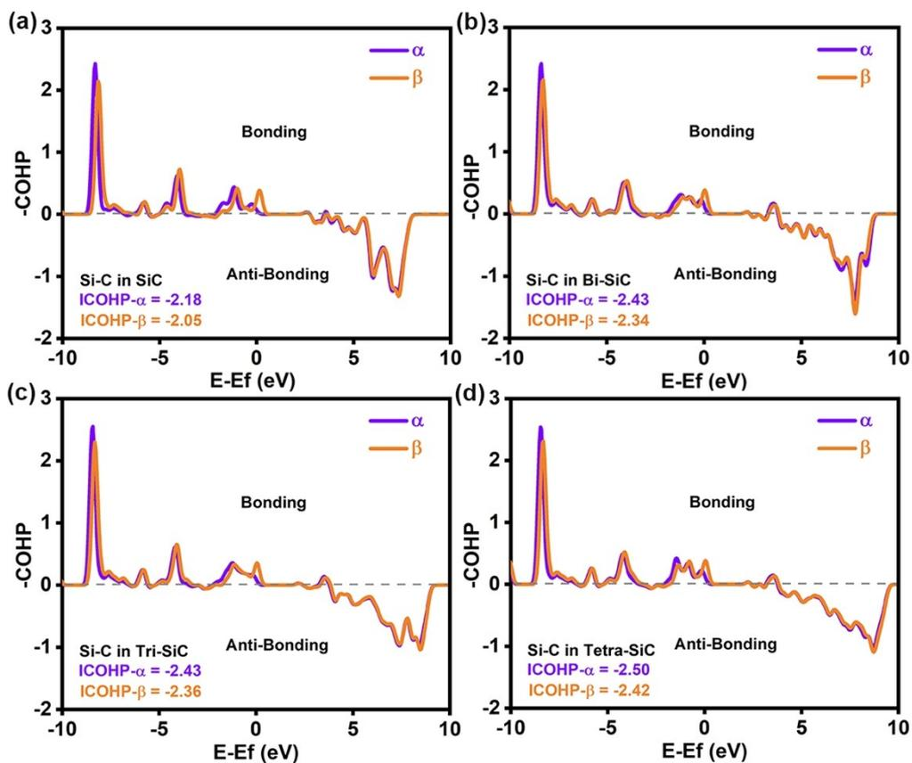
**Fig. S9.** COHP for the C in COOH\* bonded to the SiC (a), Bi-SiC (b), Tri-SiC (c), Tetra-SiC (d). The bonding and antibonding states are shown on the up and the down of the horizontal zero line.  $\alpha$  and  $\beta$  represent spin up and down, respectively.
