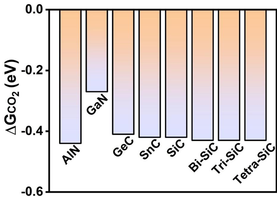
Fig. S2. Gibbs free energies of CO<sub>2</sub> adsorption at the 2D catalysts.
