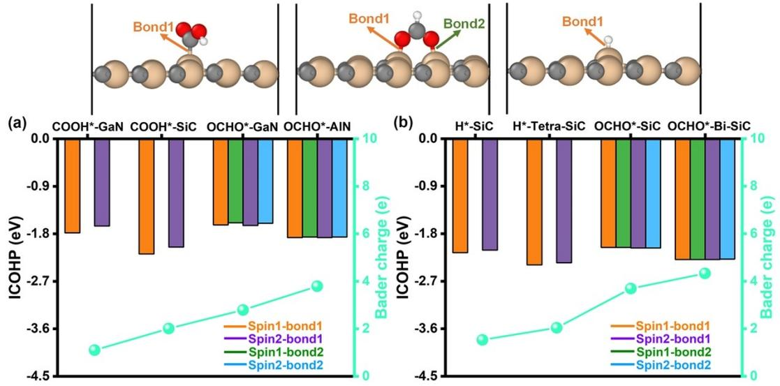
**Fig. S3.** The integrated crystal orbital Hamilton population (ICOHP) and charge variation for (a) COOH\* on GaN and SiC, and OCHO\* on GaN and AlN; (b) H\* on SiC and Tetra-SiC and OCHO\* on SiC and Bi-SiC, where positive values represent electrons lost.
