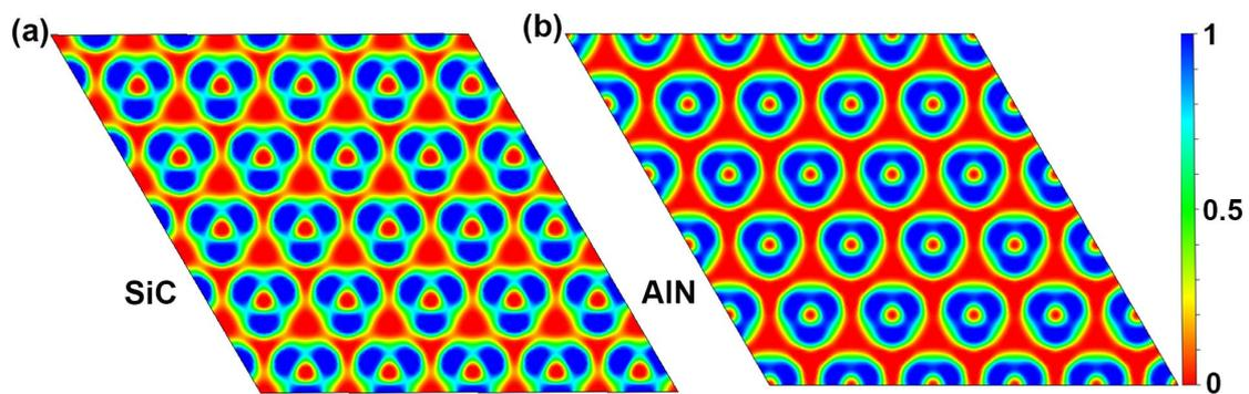
**Fig. S4.** Electron localization functions of (a) SiC and (b) AlN.
