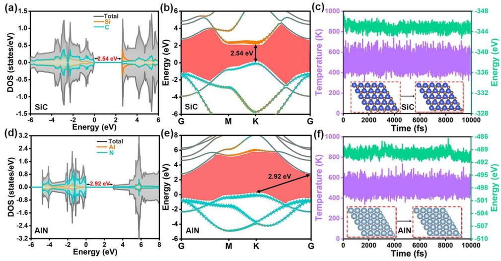
**Fig. S5.** Projected density of states of (a) SiC and (d) AlN. Projected band structure of (b) SiC and (e) AlN. *Ab initio* molecular dynamics (AIMD) simulations under 500 K at (c) SiC and (f) AlN.
