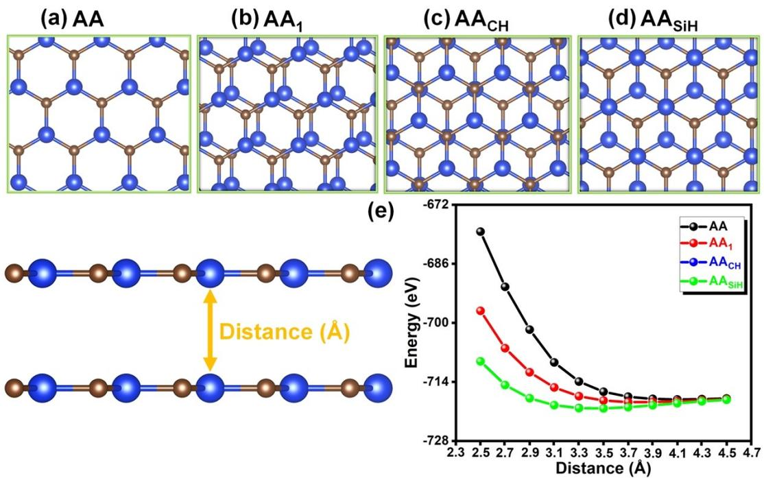
**Fig. S7** Possible stacking modes of the bi-SiC model: (a) AA, (b) AA<sub>1</sub>, (c) AA<sub>CH</sub>, and (d) AA<sub>SiH</sub>. (e) Single point energy as a function of interlayer distance for bi-SiC. Si and C elements are presented by blue and gray balls, respectively.
