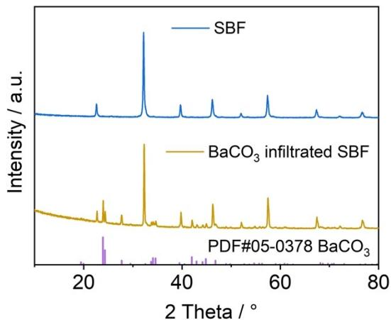
**Fig. S3.** XRD patterns of pristine SBF and BaCO<sub>3</sub> infiltrated SBF electrode after calcining at 650 °C in air.
