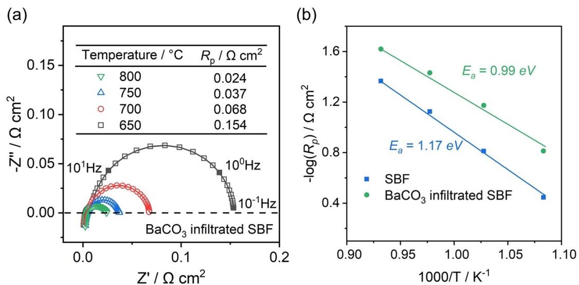
**Fig. S4.** (a) EIS of BaCO<sub>3</sub> infiltrated SBF air electrode recorded in temperature range of 650-800 °C in air. (b) Arrhenius plots of polarization resistance of pristine SBF (based on the data shown in Fig. 2a) and BaCO<sub>3</sub> infiltrated SBF electrodes.
