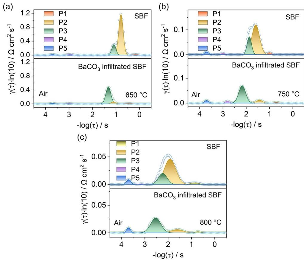
**Fig. S7.** DRT spectra of bare SBF and BaCO<sub>3</sub> infiltrated SBF electrode in air at 650 °C (a), 750 °C (b), and 800 °C (c).
