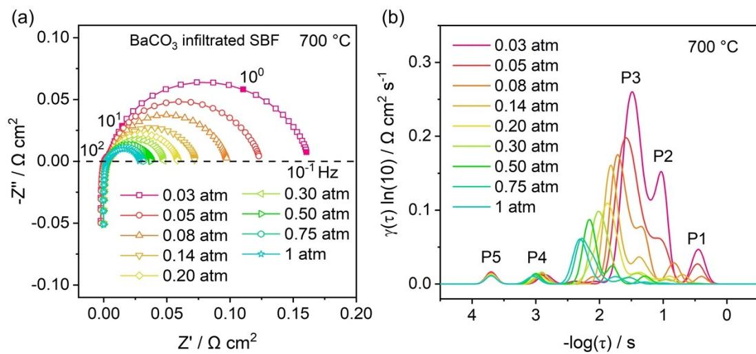
**Fig. S6.** Nyquist plots (a) and DRT spectra (b) of a symmetrical cell with BaCO<sub>3</sub> infiltrated SBF electrode measured under different oxygen partial pressures at 700 °C.
