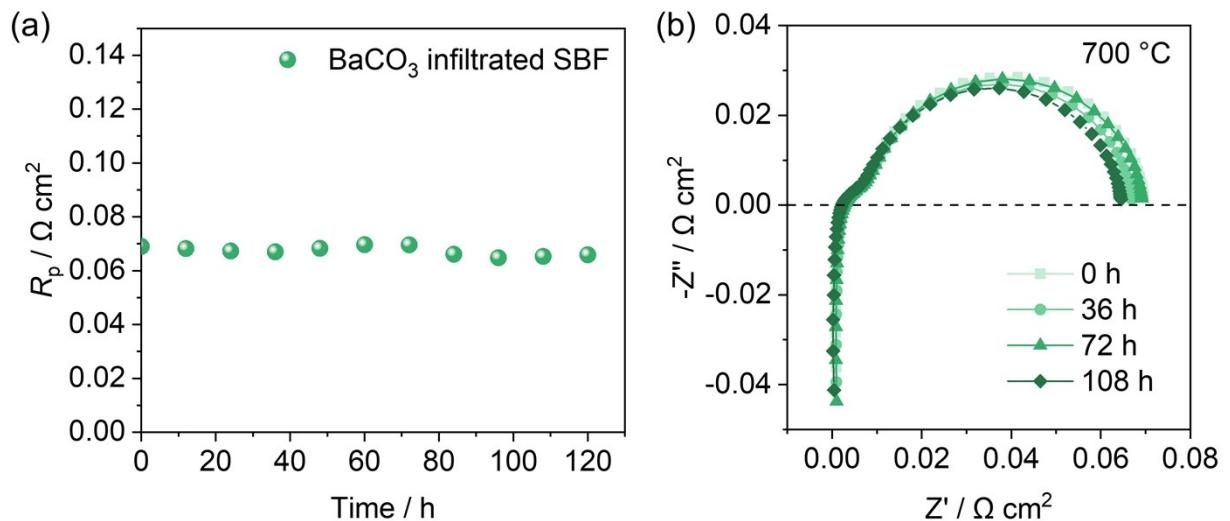
**Fig. S5.** (a) Polarization resistance and (b) Nyquist plots of symmetrical cell with BaCO<sub>3</sub> infiltrated SBF electrodes during short-term test at 700 °C in air.
