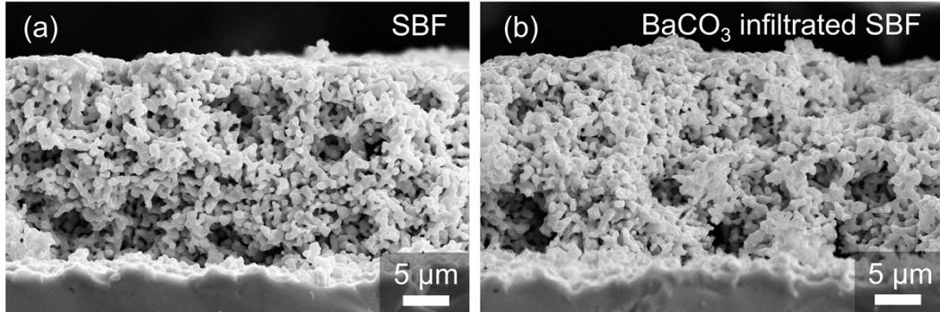
**Fig. S9.** Microstructure of cross-section of SBF (a) and  $\text{BaCO}_3$  infiltrated SBF (b) electrodes.
