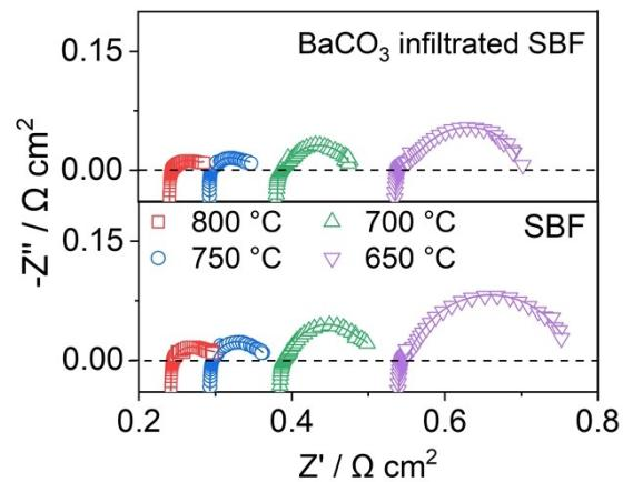
**Fig. S11.** EIS of single cells based on SBF and BaCO<sub>3</sub> infiltrated SBF air electrode with 40% H<sub>2</sub>O/H<sub>2</sub> at fuel side under open-circuit condition.
