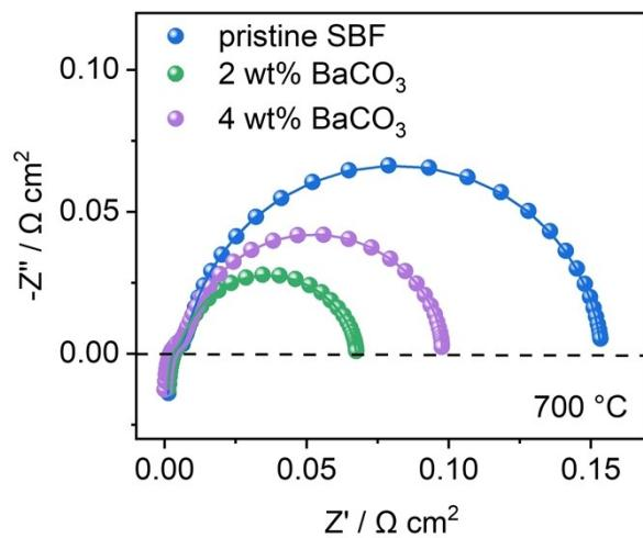
**Fig. S8.** Nyquist plots of symmetrical cell with SBF, 2 wt% and 4 wt% BaCO<sub>3</sub> infiltrated SBF electrodes measured in air at 700 °C.
