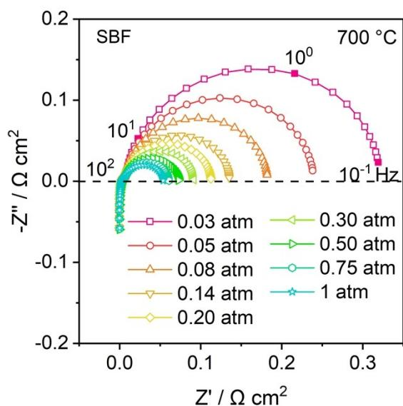
**Fig. S2.** Nyquist plots of a symmetrical cell with LSGM electrolyte and SBF electrode measured under different oxygen partial pressures at 700 °C.
