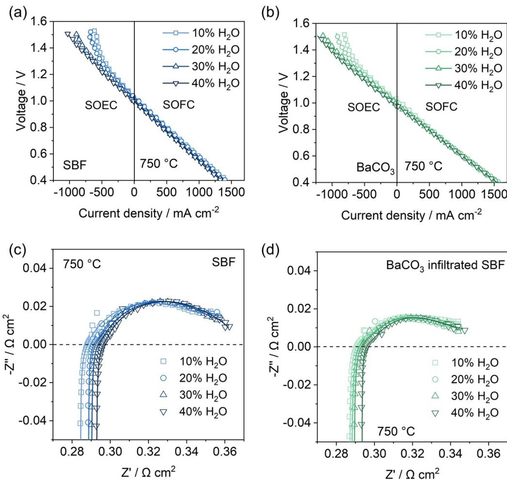
**Fig. S10.** Typical  $I$ - $V$  curves of single cells of  $\text{Ni-GDC|LDC|LSGM|SBF}$  (a) and  $\text{Ni-GDC|LDC|LSGM|BaCO}_3$  infiltrated SBF (b) at 750 °C with different humidity. EIS of single cells based on SBF (a) and  $\text{BaCO}_3$  infiltrated SBF (b) air electrode under open-circuit conditions.
