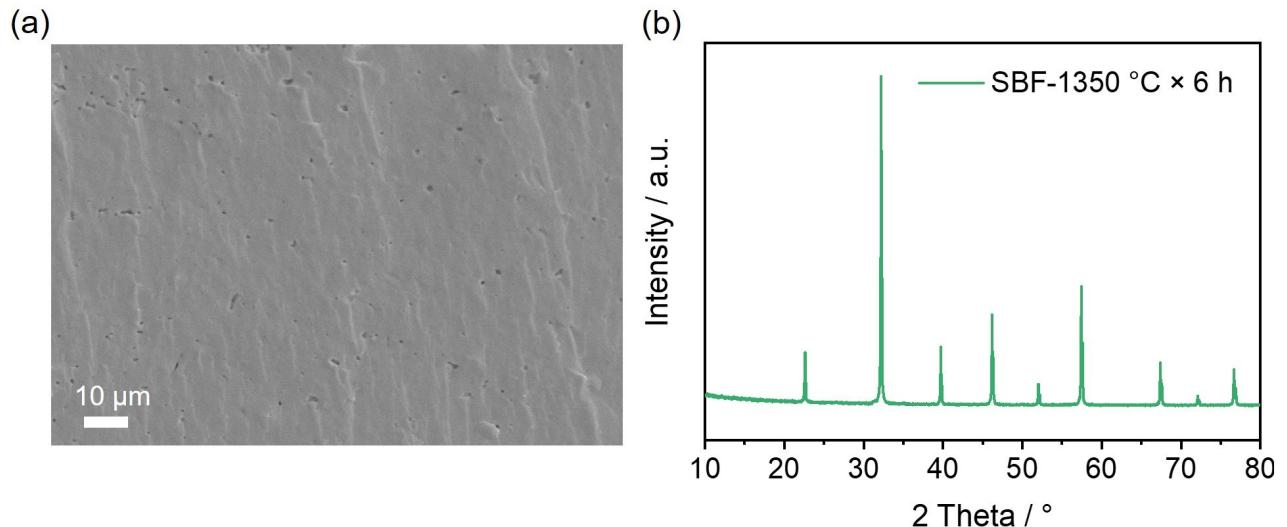
**Fig. S1.** Cross-section SEM image (a) and XRD pattern of SBF bar for TEC and electrical conductivity measurement after sintering at 1350 °C for 6 h.
