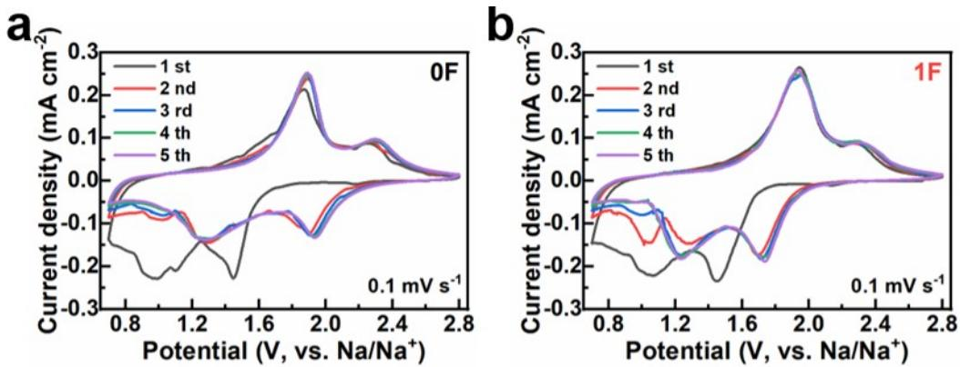
**Fig. S14.** The CV curves of (a) Na-0F battery and (b) Na-1F battery at  $0.1 \text{ mV s}^{-1}$ .
