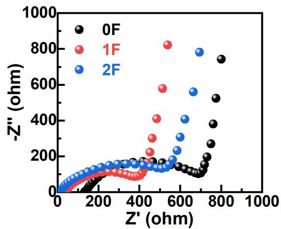
**Fig. S6.** The electrochemical impedance spectroscopy (EIS) of 0F, 1F and 2F.
