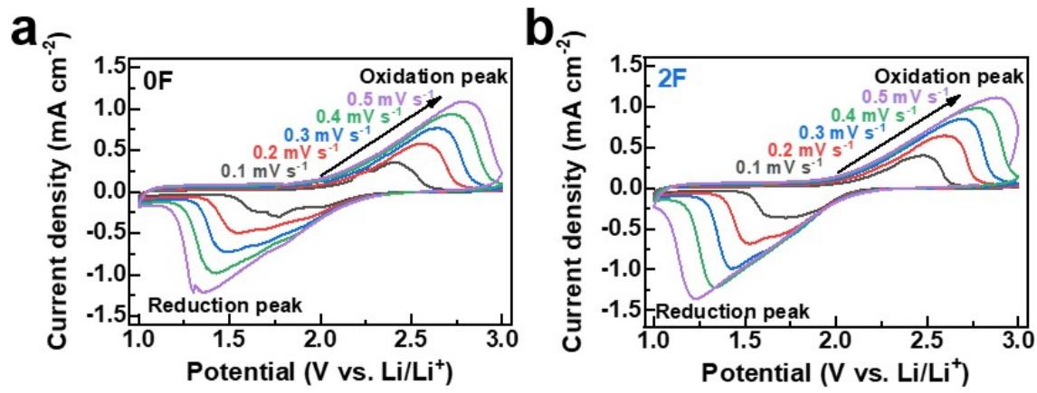
**Fig. S7.** CV curves of (a) 0F and (b) 2F from  $0.1$  to  $0.5\text{ mV s}^{-1}$ .
