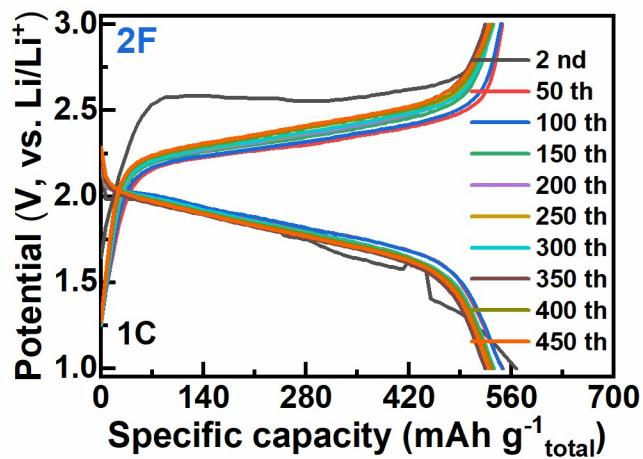
**Fig. S8.** The discharge-charge curves of 2F at various cycles.
