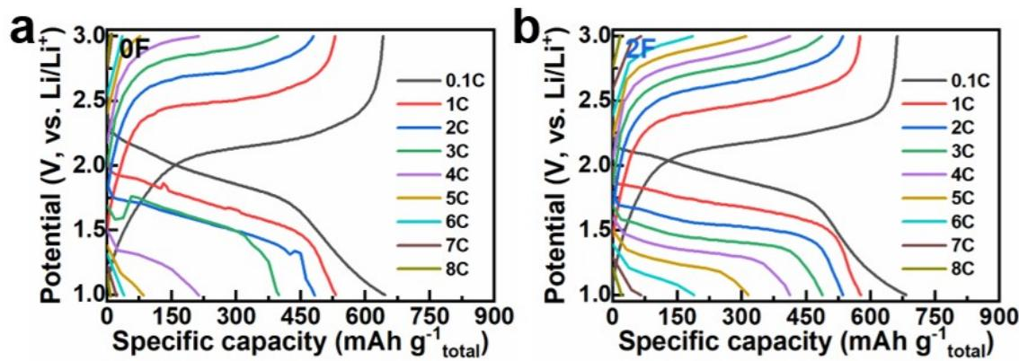
**Fig. S9.** The discharge-charge curves of (a) 0F and (b) 2F at various rates.
