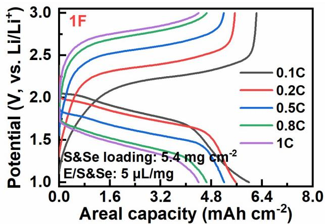
**Fig. S12.** The discharge-charge curves of 1F at different rates under practical conditions.
