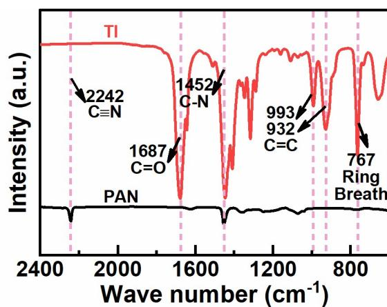
**Fig. S2.** FT-IR spectrum of TI and PAN.
