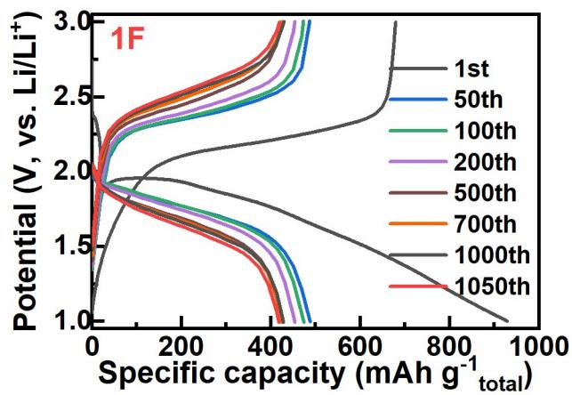
**Fig. S11.** The discharge-charge curves of 1F at different cycles.
