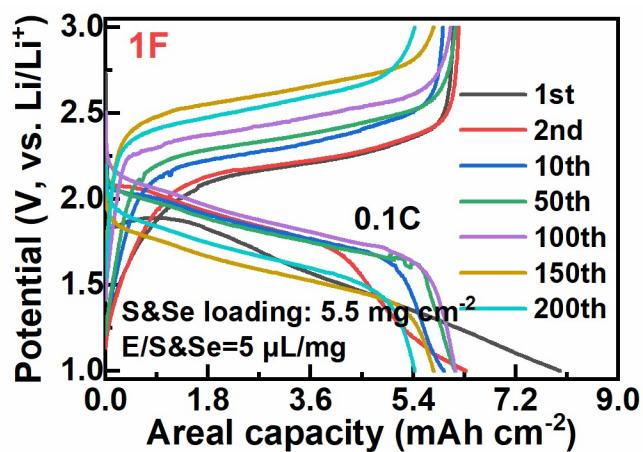
**Fig. S13.** The discharge-charge curves of 1F at different cycles under practical conditions.
