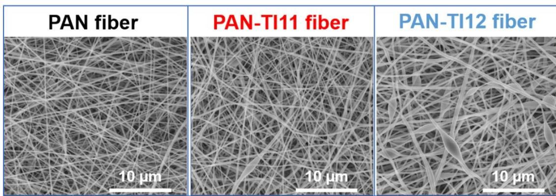
**Fig. S1.** SEM images of PAN fiber, PAN-TI11 fiber and PAN-TI12 fiber, respectively.
