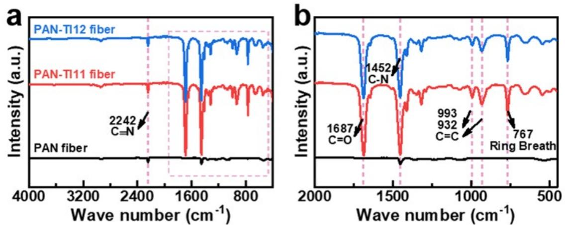
**Fig. S3.** (a) FT-IR spectrum of PAN fiber, PAN-TI11 fiber and PAN-TI12; (b) The partial enlarged FT-IR spectrum.
