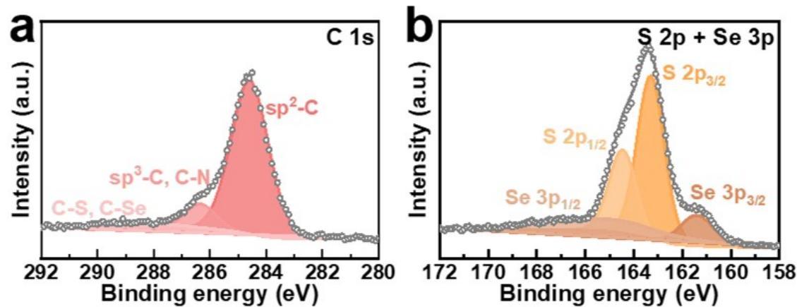
**Fig. S5.** (a) C 1s and (b) S 2p + Se 3p XPS spectra of  $\text{Se}_{0.05}\text{S}_{0.95}\text{PAN-TI12}$  fiber.
