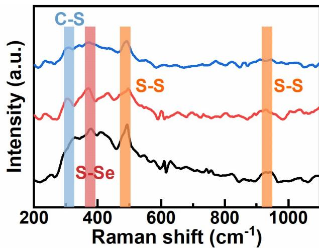
**Fig. S4.** Local enlarged Raman spectra of  $\text{Se}_{0.05}\text{S}_{0.95}\text{PAN}$  fiber,  $\text{Se}_{0.05}\text{S}_{0.95}\text{PAN-TI11}$  and 12 fibers.
