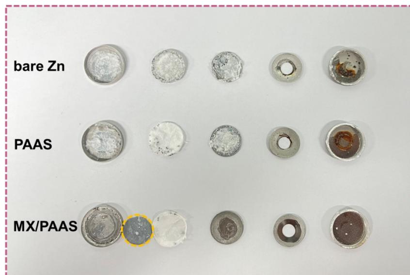
Figure. S25 The corresponding optical images of each component for bare Zn, PAAS@Zn and MX/PAAS@Zn symmetric batteries after 2000 plating/stripping cycling
