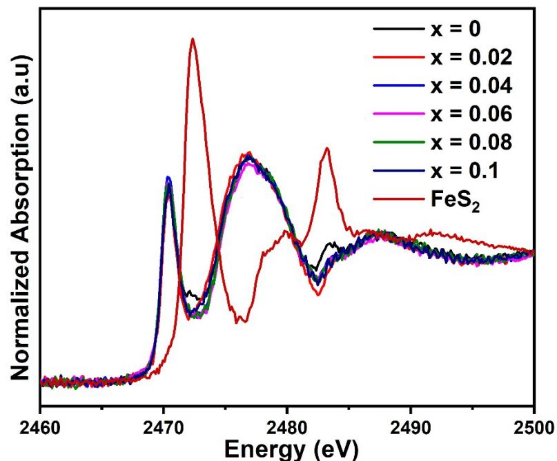
**Figure S2.** Sulfur absorption spectra for  $\text{Cu}_{1-x}\text{Cr}_x\text{FeS}_2$  ( $0 \leq x \leq 0.1$ ) and  $\text{FeS}_2$ .
