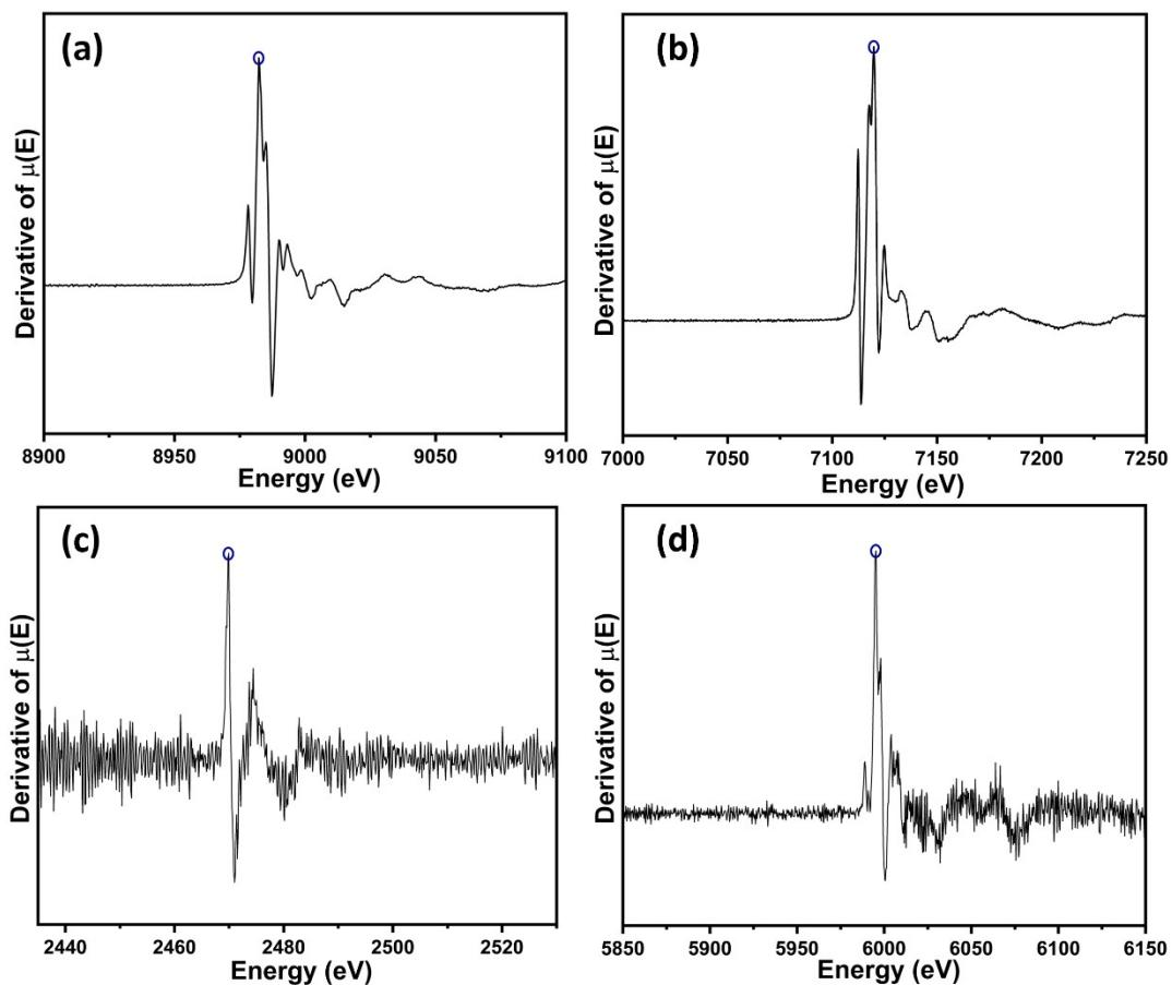
**Figure S1.** The first derivative of the absorption ( $\mu(E)$ ) of the (a) copper (b) iron (c) chromium and (d) sulfur spectra for  $\text{Cu}_{0.92}\text{Cr}_{0.08}\text{FeS}_2$ . The K-edge absorption energies were extracted from the maxima as shown by blue circles.
