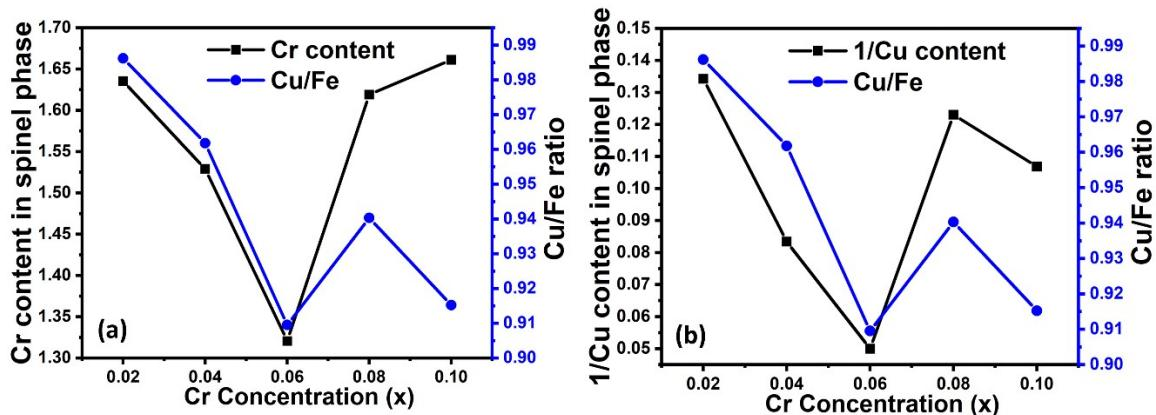
**Figure S4.** The dependence of (a) Cr content and (b)  $1/\text{Cu}$  in the spinel secondary phase, on the Cu:Fe ratio in the main phase plotted as a function of nominal Cr concentration ( $x$ ).
