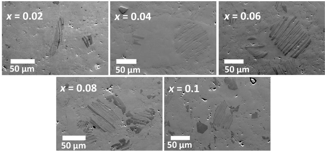
**Figure S3.** SEM images of  $\text{Cu}_{1-x}\text{Cr}_x\text{FeS}_2$  ( $0.02 \leq x \leq 0.1$ ) samples showing the spinel-type secondary phase.
