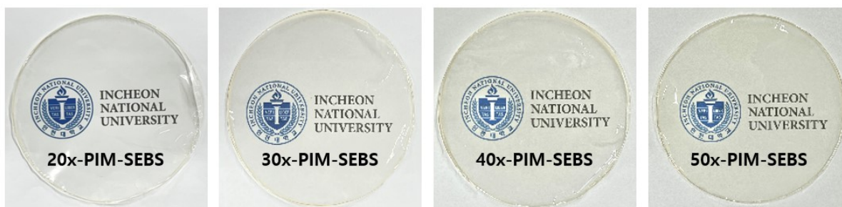
Figure S3. Photographs of the crosslinked (PIM- N -methyl piperidinium)-SEBS membranes (x-PIM-SEBS) with different crosslinking degrees
