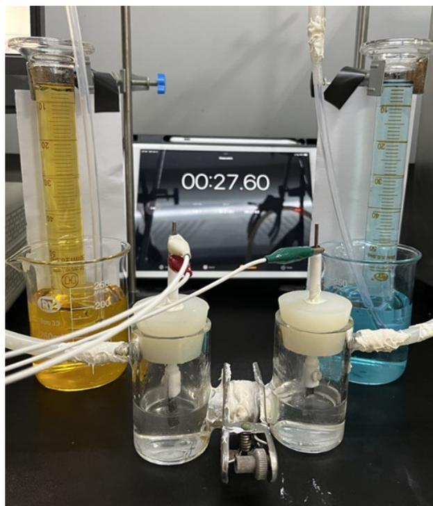
**Fig. S24** Device diagram for measuring Faraday efficiency at the ambient condition. The electrolyte in the electrolytic cell is separated by a Nafion membrane.
