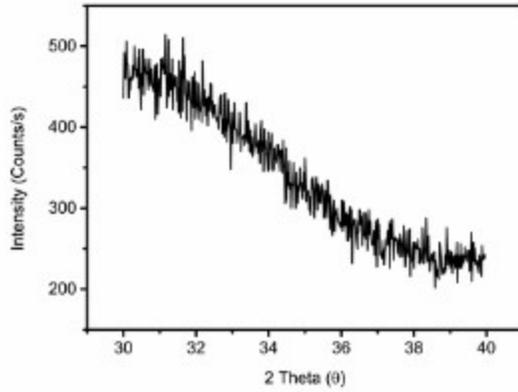
**Figure S9** X-ray diffractogram of ITO sputtered on glass at room temperature under DC power of 75 W for 7 min.
