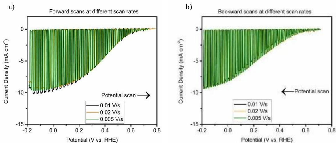
**Figure S3** Current-density potential curves of CZTS/CdS/Pt at different scan rates of 0.01 V/s, 0.02 V/s and 0.005 V/s in 1 M  $\text{K}_2\text{HPO}_4/\text{KH}_2\text{PO}_4$  (pH 7) solution under chopped AM 1.5G light irradiation for (a) Anodic and (b) Cathodic directions.
