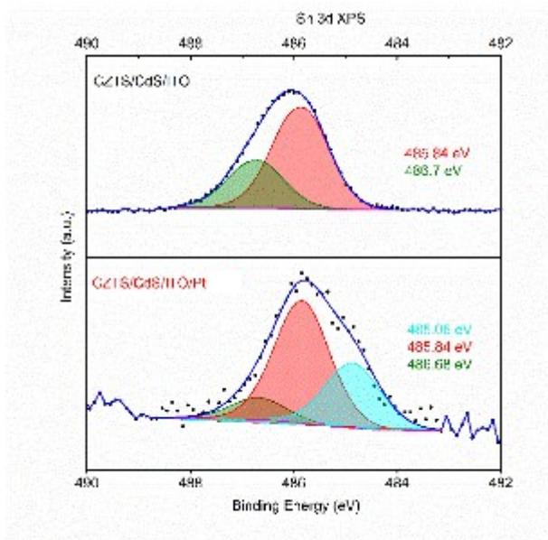
**Figure S4** Sn 3d XPS spectra of CZTS/CdS/ITO (top panel) vs CZTS/CdS/ITO/Pt (bottom panel). The peaks are assigned to Sn<sup>4+</sup> (green) and Sn<sup>2+</sup> (red) in tin oxide and metallic tin (blue).<sup>1</sup>
