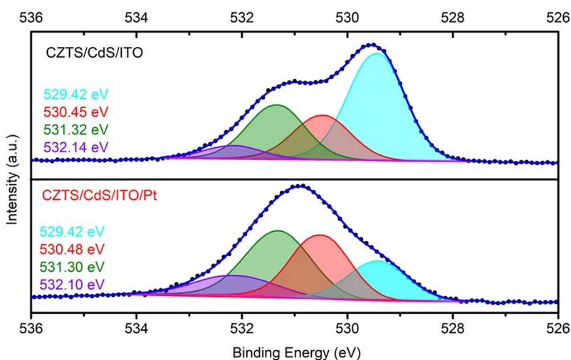
**Figure S5** O 1s XPS spectra of CZTS/CdS/ITO and CZTS/CdS/ITO/Pt. The peaks are assigned to lattice oxygen (blue) and oxygen adjacent to oxygen-deficient positions (red) in indium oxide (In<sub>2</sub>O<sub>3</sub>), surface hydroxide or oxyhydroxide (green), and unidentified surface contaminants (purple).
