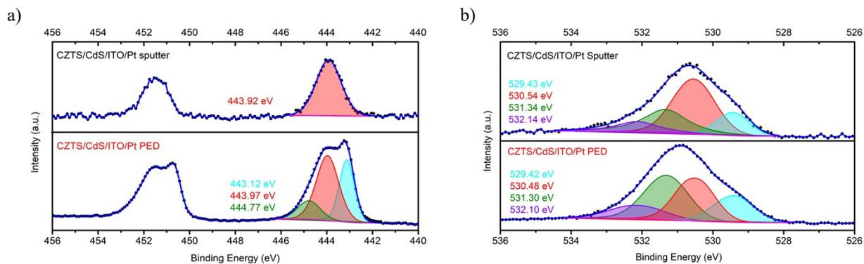
**Figure S6** (a) In 3d XPS spectra of CZTS/CdS/ITO with Pt sputter vs CZTS/CdS/ITO with Pt photoelectrodeposited (PED). (b) Corresponding O 1s XPS Spectra. The peaks are assigned to indium oxide ( $\text{In}_2\text{O}_3$ ) (red), indium hydroxide ( $\text{In}(\text{OH})_3$ ) (green), metallic
