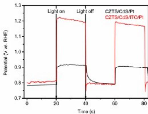
**Figure S10** Open circuit potential measurements for CZTS/CdS/Pt (black) and CZTS/CdS/ITO/Pt (red) in 1 M  $K_2HPO_4/KH_2PO_4$  solution (pH7) under constant AM 1.5G light irradiation.
