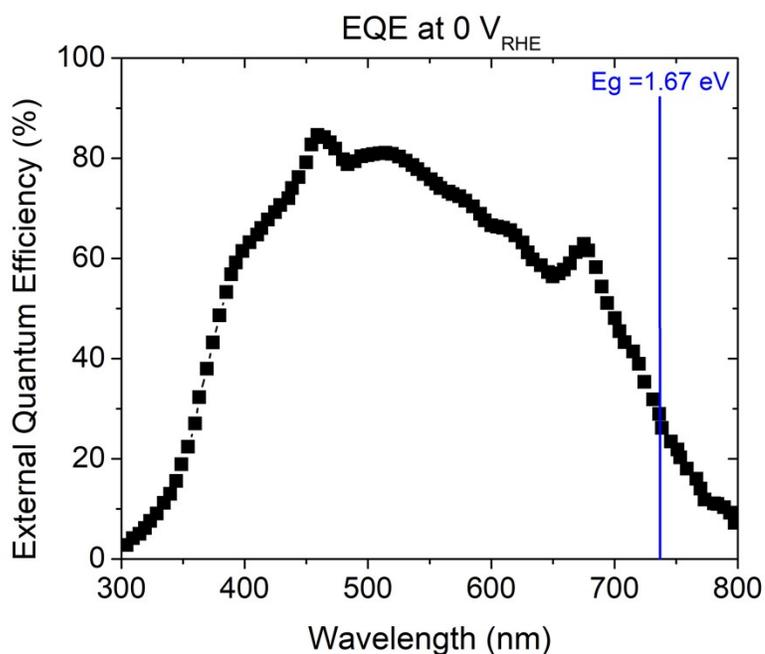
**Figure S1** External Quantum Efficiency (EQE) of CZTS/CdS/ITO/Pt photocathode stacks in 1 M K<sub>2</sub>HPO<sub>4</sub>/KH<sub>2</sub>PO<sub>4</sub> (pH 7) solution under applied potential of 0 V<sub>RHE</sub>. d(EQE)/dE is used for band gap extraction.
