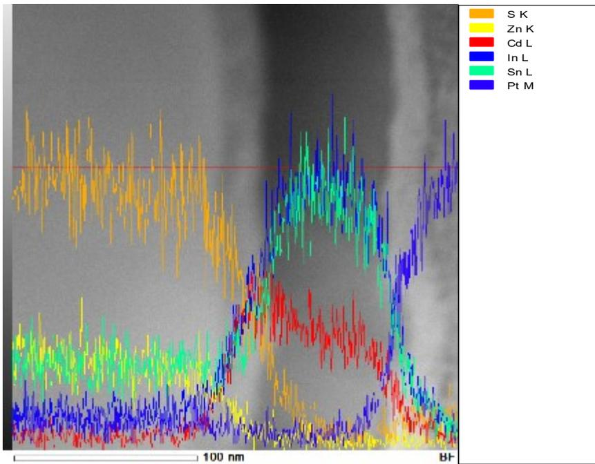
**Figure S8** TEM EDX Line scan of CZTS/CdS/ITO interface.
