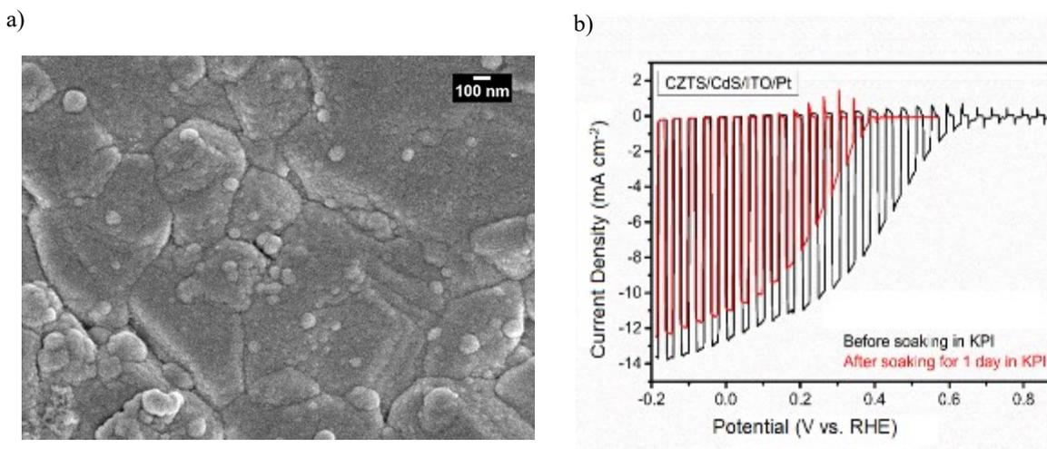
**Figure S15** Scanning Electron Microscope (SEM) of CZTS/CdS/ITO/Pt after immersing in 1M  $\text{K}_2\text{HPO}_4/\text{KH}_2\text{PO}_4$  (pH 7) overnight in the dark without any applied potential. (b) Current density-potential curve of CZTS/CdS/ITO/Pt under chopped solar-simulated AM 1.5G light irradiation before and after immersing in 1M  $\text{K}_2\text{HPO}_4/\text{KH}_2\text{PO}_4$  (pH 7) for 1 day in the dark.
