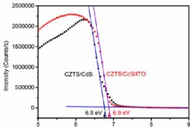
**Figure S11** UPS He(I) spectra at an applied bias of -10V for CZTS/CdS (black) and CZTS/CdS/ITO (red).
