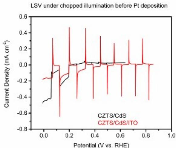
**Figure S2** Current density-potential curves of CZTS/CdS and CZTS/CdS/ITO in 0.1 M  $\text{Na}_2\text{SO}_4$  electrolyte (pH 9.5) under chopped solar-simulated AM 1.5G light irradiation.
