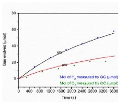
**Figure S13** Time-course curves of  $\text{H}_2$  and  $\text{O}_2$  evolution of CZTS/CdS/ITO/Pt photocathode in the same electrolyte under the same measurement conditions. Solid lines represent the time-course curve for  $e^-/2$  (black) and  $e^-/4$  (red) determined from current measured and dots representing  $\text{H}_2$  (blue) and  $\text{O}_2$  (green) measured by Gas Chromatography (GC) at regular intervals of 10 min.
