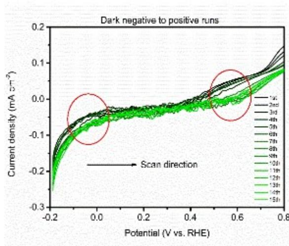
**Figure S12** Linear sweep voltammetry scans done in the dark condition from  $-0.2 V_{\text{RHE}}$  to  $0.8 V_{\text{RHE}}$
