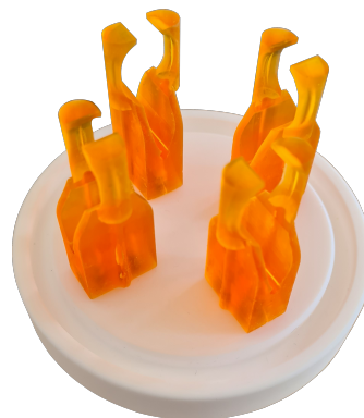
(b) Picture of the robotic sampleholder with four applied grippers for the gold coated alumina substrate.
