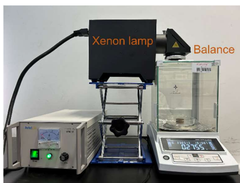
Fig. S34. Schematic diagram of photo-driven solvent evaporation experimental set-up.
