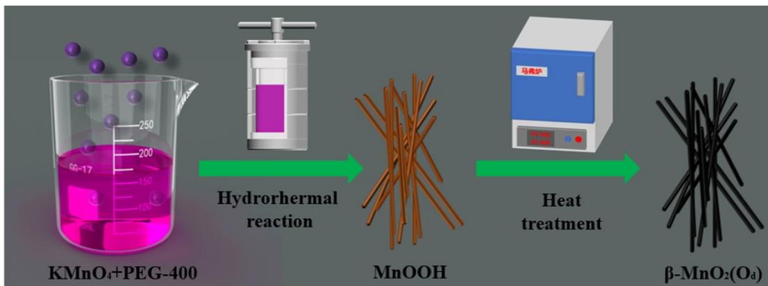
3 **Figure S1.** Preparation schematic of  $\beta$ - $\text{MnO}_2$  ( $\text{O}_d$ ) electrode material.
