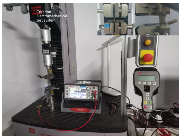
Figure S4. Picture of the criterion electromechanical test equipment
