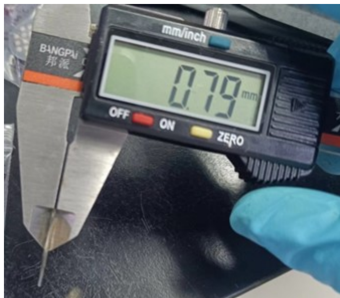
Fig. S6. Schematic diagram of wafer thickness.
