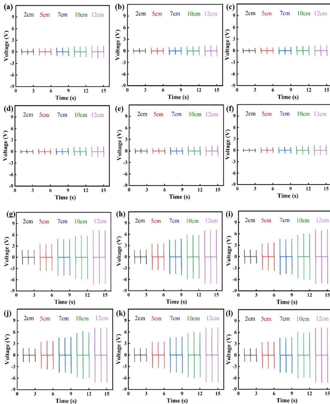
**Fig. S7** Power generation stability of the superhydrophobic-coated ferromagnetic TENG in extreme environments. The electrical signals of (a-f) ferromagnetic TENG and (g-l) superhydrophobic-coated ferromagnetic TENG in deionised water, acid (0.1 M HCl), alkali (0.1 M NaOH), salt (3.5 wt.% NaCl), tea and coffee environments, respectively.
