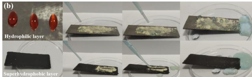
**Fig. S5 (a)** Different types of liquid droplets with a spherical shape on a superhydrophobic layer: deionized water, Cola, Coffee, acid (0.1 M HCl), base (0.1 M NaOH), and salt (3.5 wt.% NaCl). **(b)** Photographs showing the self-cleaning process of the hydrophilic layer of bare steel and superhydrophobic layer of ferromagnetic TENG (with a small inclination angle ( $<5^\circ$ )) after chalk ash deposition.
