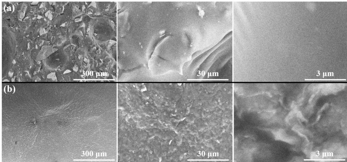
**Fig. S1** SEM images of **(a)** merkel disc magnetic elastomer base surface and **(b)** MXene-coated merkel disc magnetic elastomer base surface at different magnification.
