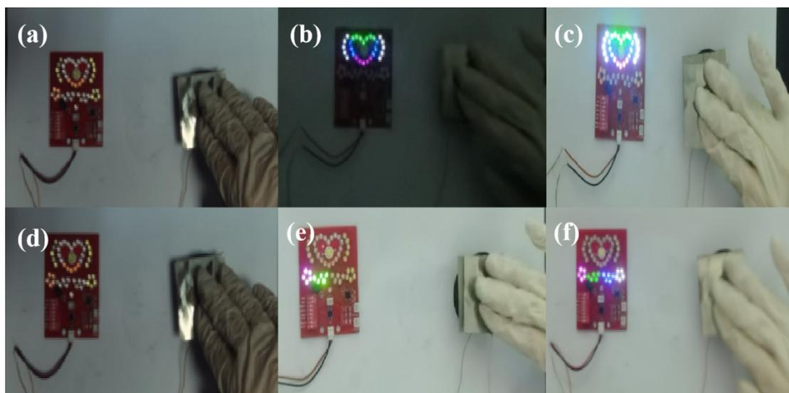
Fig. S4 LED bulbs lit with TENG in the background of (a-c) direct current mode and (d-f) alternating current mode.
