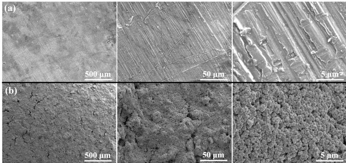
**Fig. S2** SEM images of **(a)** ferromagnetic TENG surface and **(b)** superhydrophobic-coated ferromagnetic TENG surface at different magnification.
