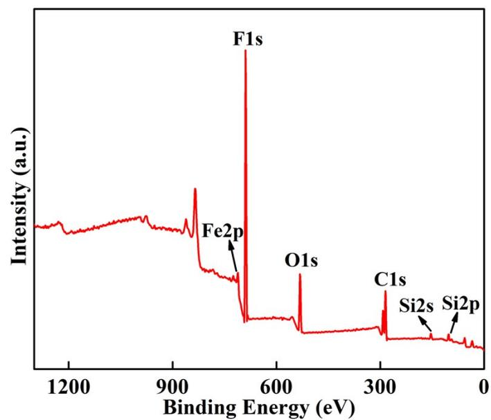
Fig. S3 XPS survey spectra of superhydrophobic layer surface.
