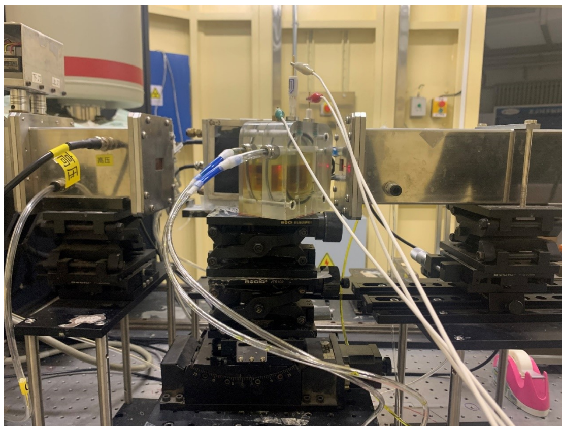
Figure S11. Photograph of the device used for in-situ XAFS measurements during electrocatalytic p -NP reduction.
