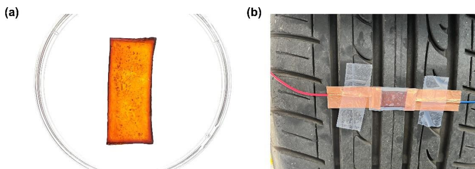
Fig. S8. Optical images of (a) the polyurethane swelled by ionic liquid and (b) the ionic liquid-based temperature sensor used in automotive loading experiments.
