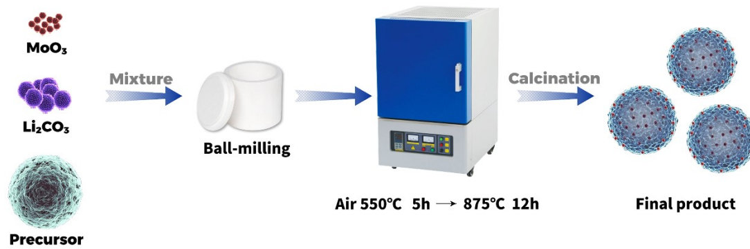
Fig. S1. Schematic diagram of material synthesis
