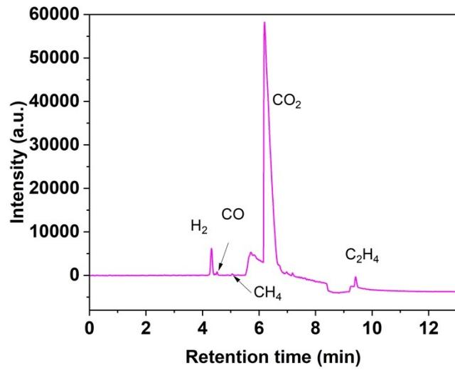
**Fig. S8** Gas chromatography for gas products in CO<sub>2</sub>RR on the Cu<sub>2</sub>O@SiO<sub>2</sub>-NH<sub>2</sub> catalyst at the current density of 280 mA cm<sup>-2</sup>.
