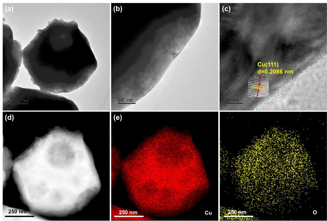
**Fig. S16** Morphological and structural characterizations of  $\text{Cu}_2\text{O}$  after the  $\text{CO}_2\text{RR}$  test. (a and b) TEM images; (c) HR-TEM image; (d) HAADF-STEM image and (e) EDX mapping.
