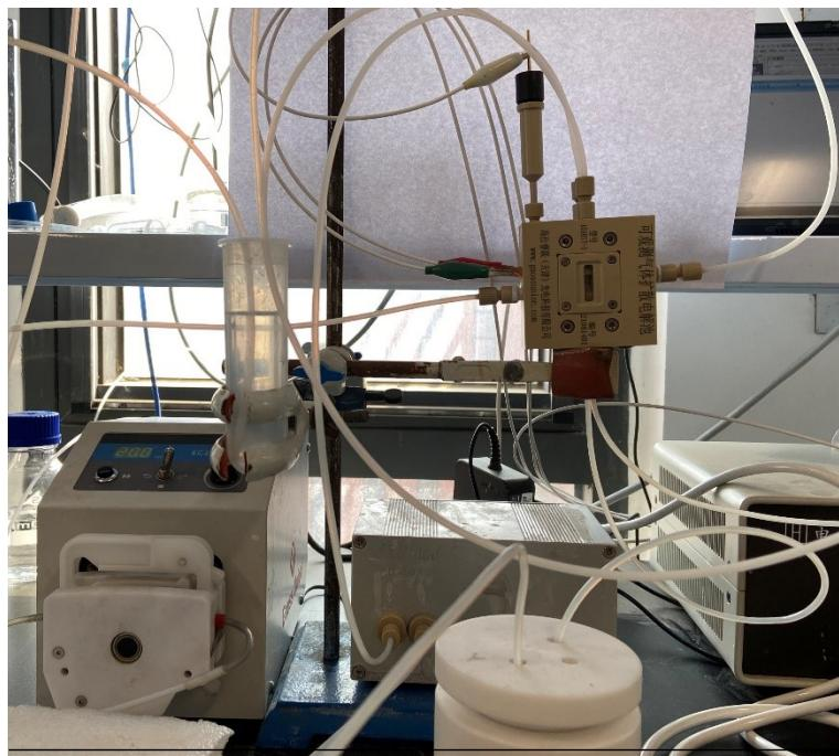
**Fig. S7** Electrochemical  $\text{CO}_2$  reduction reaction system.
