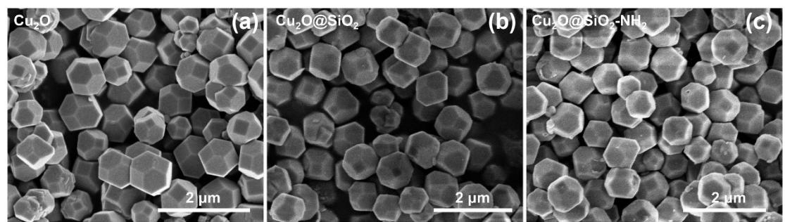
**Fig. S1** The SEM images of (a) Cu<sub>2</sub>O, (b) Cu<sub>2</sub>O@SiO<sub>2</sub> and (c) Cu<sub>2</sub>O@SiO<sub>2</sub>-NH<sub>2</sub> catalysts.
