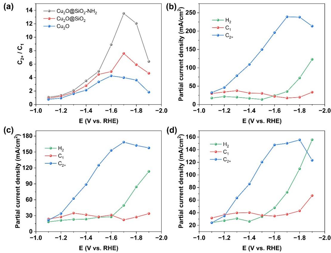
**Fig. S11** (a) The ratios of  $\text{C}_{2+}/\text{C}_1$  products and the partial current densities of products in  $\text{CO}_2\text{RR}$  on (b)  $\text{Cu}_2\text{O}@\text{SiO}_2\text{-NH}_2$ , (c)  $\text{Cu}_2\text{O}@\text{SiO}_2$  and (d)  $\text{Cu}_2\text{O}$  catalysts.
