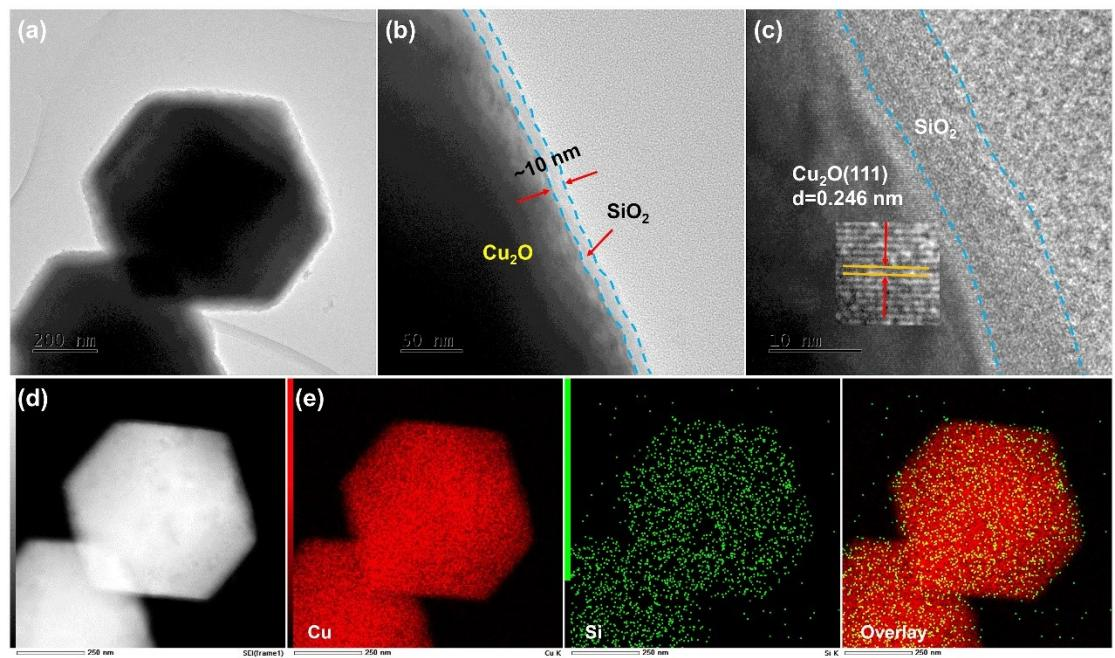
**Fig. S3** Morphological and structural characterizations of  $\text{Cu}_2\text{O}@\text{SiO}_2$ . (a, b) TEM images; (c) HR-TEM image; (d) HAADF-STEM image and (e) EDX mapping.
