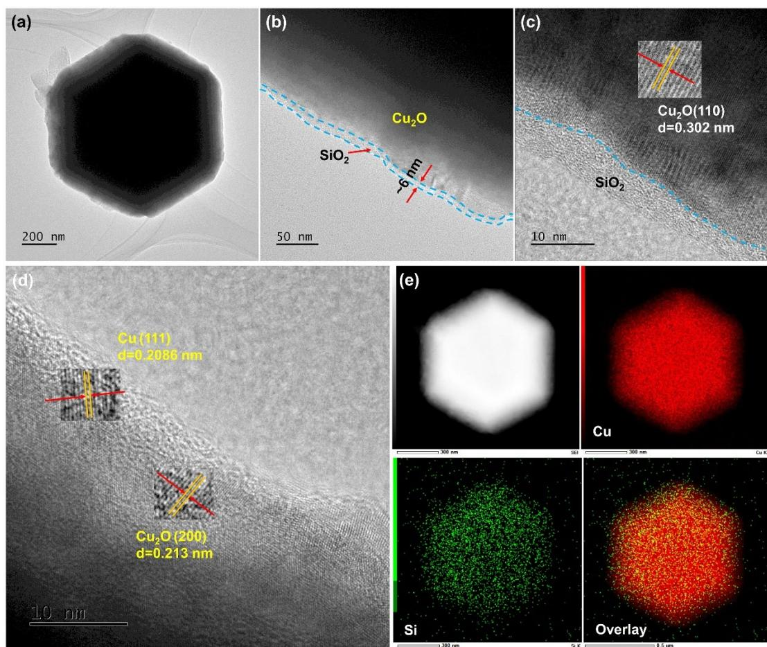
**Fig. S15** Morphological and structural characterizations of  $\text{Cu}_2\text{O}@\text{SiO}_2$  after the  $\text{CO}_2\text{RR}$  test. (a and b) TEM images; (c and d) HR-TEM images; (e) EDX mapping.
