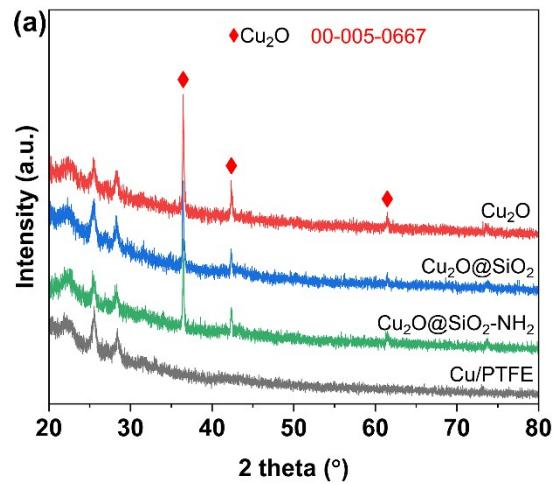
**Fig. S5** XRD patterns of  $\text{Cu}_2\text{O}$ ,  $\text{Cu}_2\text{O}@\text{SiO}_2$  and  $\text{Cu}_2\text{O}@\text{SiO}_2\text{-NH}_2$  catalysts on the Cu/PTFE substrate.
