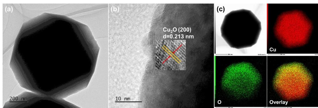
**Fig. S2** Morphological and structural characterizations of  $\text{Cu}_2\text{O}$ . (a) TEM image; (b) HR-TEM image and (c) EDX mapping.
