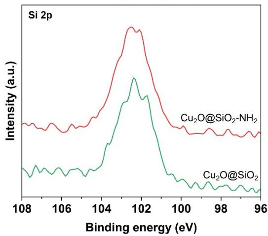
**Fig. S17** Si 2p XPS spectra of  $\text{Cu}_2\text{O}@\text{SiO}_2$  and  $\text{Cu}_2\text{O}@\text{SiO}_2-\text{NH}_2$  catalysts after the  $\text{CO}_2\text{RR}$  test.
