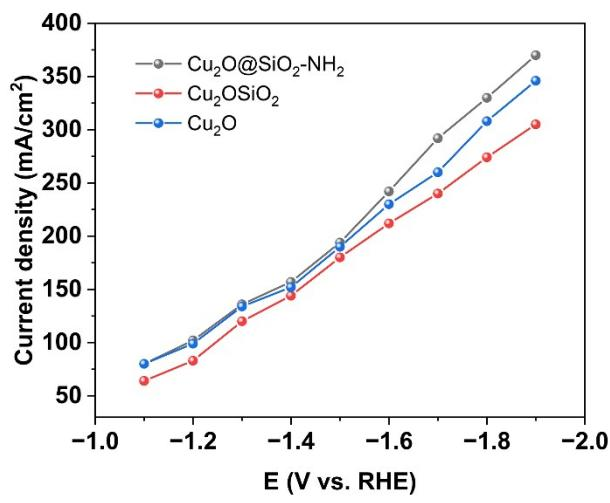
**Fig. S10** The current densities of CO<sub>2</sub>RR on Cu<sub>2</sub>O@SiO<sub>2</sub>-NH<sub>2</sub>, Cu<sub>2</sub>O@SiO<sub>2</sub> and Cu<sub>2</sub>O catalysts.
