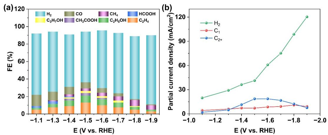
**Fig. S12** The product distributions and partial current densities of CO<sub>2</sub>RR over the Cu/PTFE substrate. (a) Product distributions and (b) Partial current densities.
