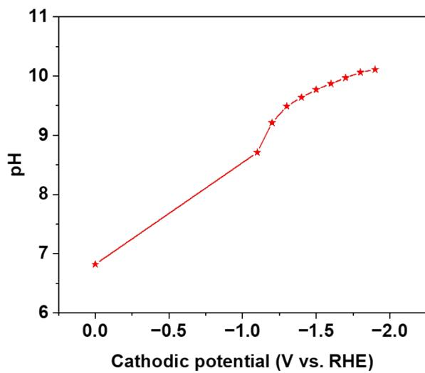
**Fig. S13** The pH values of the electrolyte during CO<sub>2</sub>RR.
