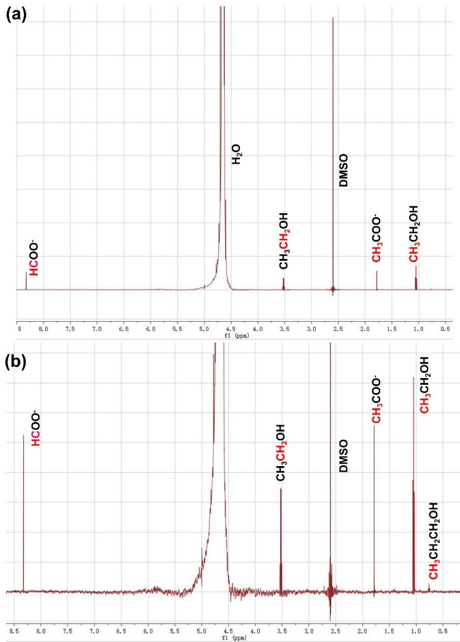
**Fig. S9** (a)  $^1\text{H}$  NMR spectrum for liquid phase products in CO<sub>2</sub>RR on Cu<sub>2</sub>O@SiO<sub>2</sub>-NH<sub>2</sub> catalyst at the current density of 280 mA cm<sup>-2</sup>. (b) is an enlarged view of (a). DMSO is used as internal standard.
