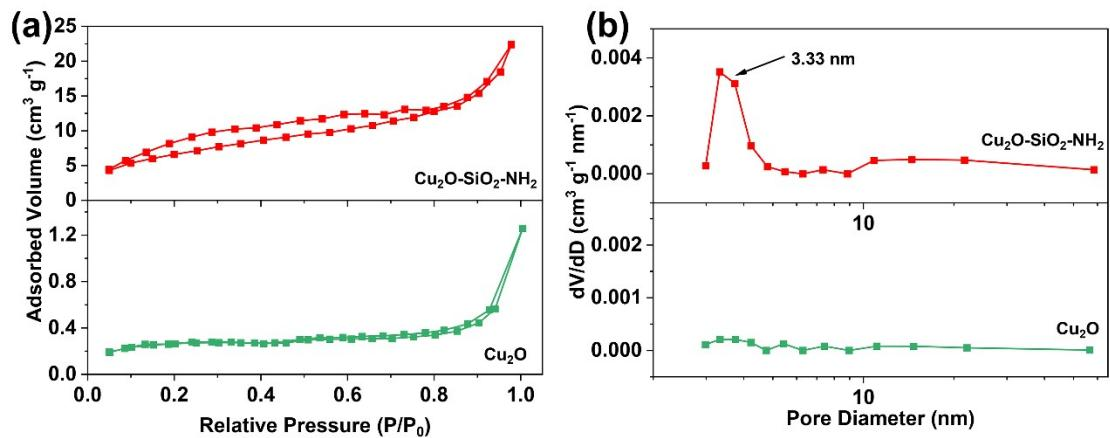
**Fig. S4.** (a) N<sub>2</sub> adsorption-desorption isotherms and (b) The pore size distribution curves of Cu<sub>2</sub>O and Cu<sub>2</sub>O@SiO<sub>2</sub>-NH<sub>2</sub> catalysts.
