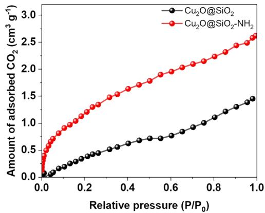
**Fig. S6** The CO<sub>2</sub> adsorption isotherms of Cu<sub>2</sub>O@SiO<sub>2</sub>-NH<sub>2</sub> and Cu<sub>2</sub>O@SiO<sub>2</sub>.
