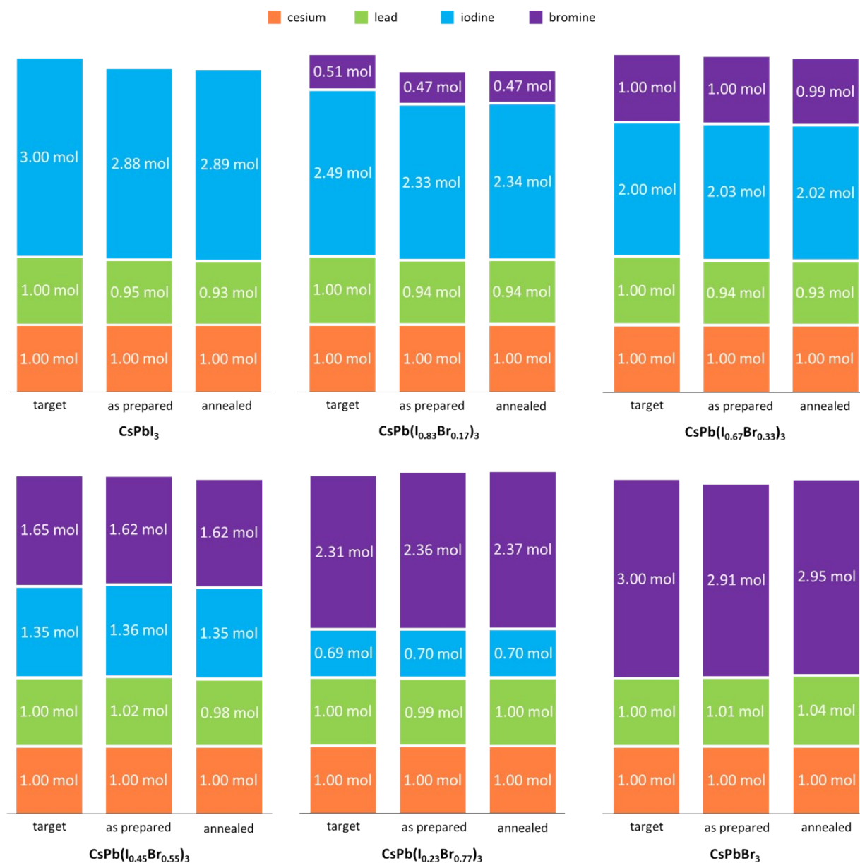
Fig. S3: Inductively coupled plasma mass spectrometry (ICP-MS) analysis of the composition of thin films prepared by CFS of mechano-chemically synthesized source powders with different iodine-to-bromine ratios. All thin films exhibit the expected composition of stoichiometric source powder indicating a direct compositional transition from powder to thin film, thus, a deposition within the flash sublimation regime. In addition, post annealing does not change the general composition of the thin films. All molar ratios have been normalized to the cesium values. The expected error of the measurement is in the range of \pm 5\%_{\text{rel}} .
