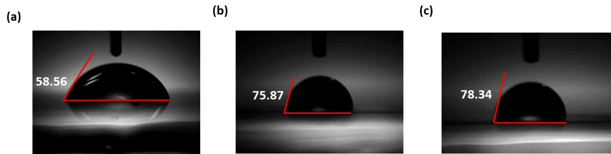
Fig. S13. Water contact angle measurement of (a) control PVK, (b) PVK/SPX-BT, and (c) PVK/SPX-TPA.
