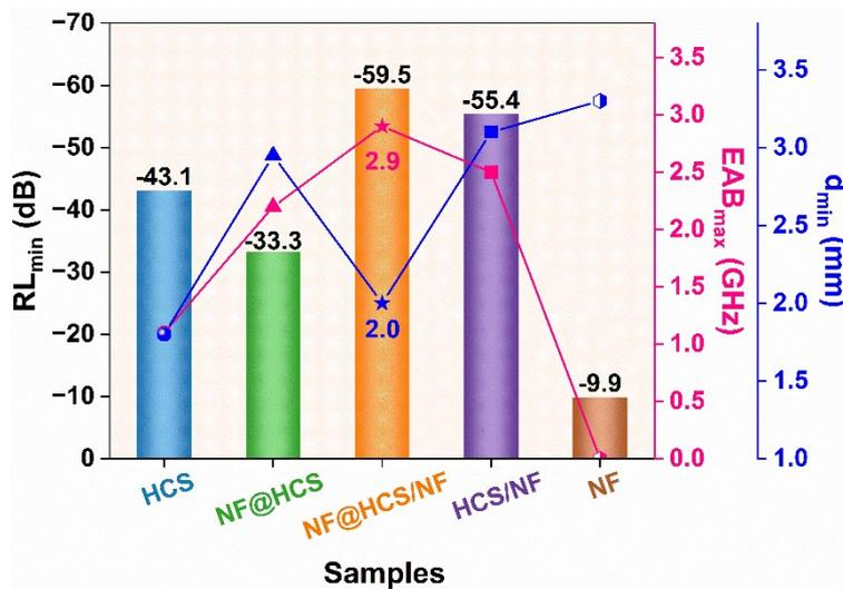
Fig. S7 The EMW absorption performance ( $RL_{min}$ ,  $EAB_{max}$ , and  $d_{min}$  values) summary graph of HCS, NF@HCS, NF@HCS/NF, HCS/NF, and NF.
