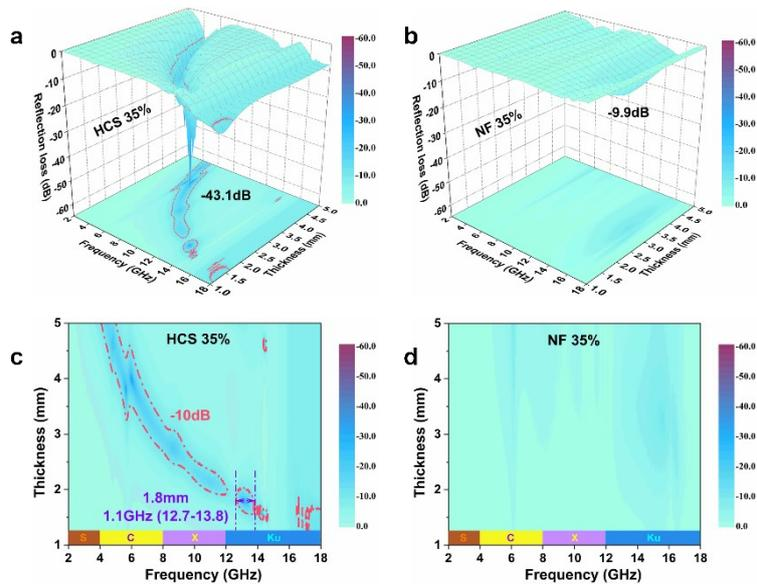
Fig. S6 The 3D RL diagrams and corresponding 2D RL mapping graphs of pure HCS and NF at filling contents of 35 wt%.
