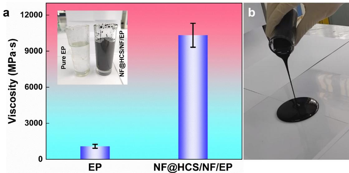
Fig. S13 (a) The viscosity of pure EP and NF@HCS/NF/EP systems, and the mass ratio of fillers is also 35% as above. Though the viscosity of NF@HCS/NF/EP (10322 MPa·s) is higher than pure EP (1088 MPa·s), the viscosity below 20000 MPa·s is still suitable for potting application. (b) The demonstration experiment showing good leveling performance of NF@HCS/NF/EP system.
