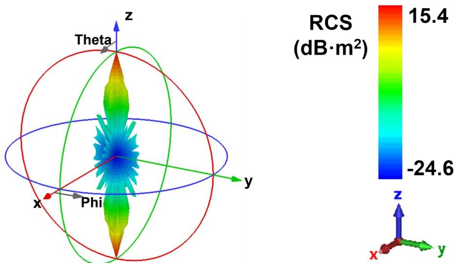
Fig. S9 CST 3D simulation plot of the perfect electric conductor (PEC) used here.
