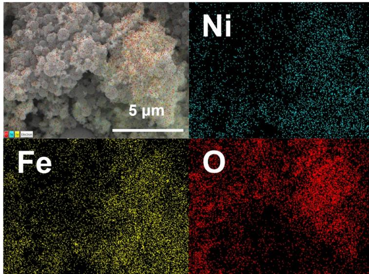
Fig. S4 The EDX mapping graphs of elemental distributions in NF@HCS powders, indicating the presence of Fe, Ni, and O elements.
