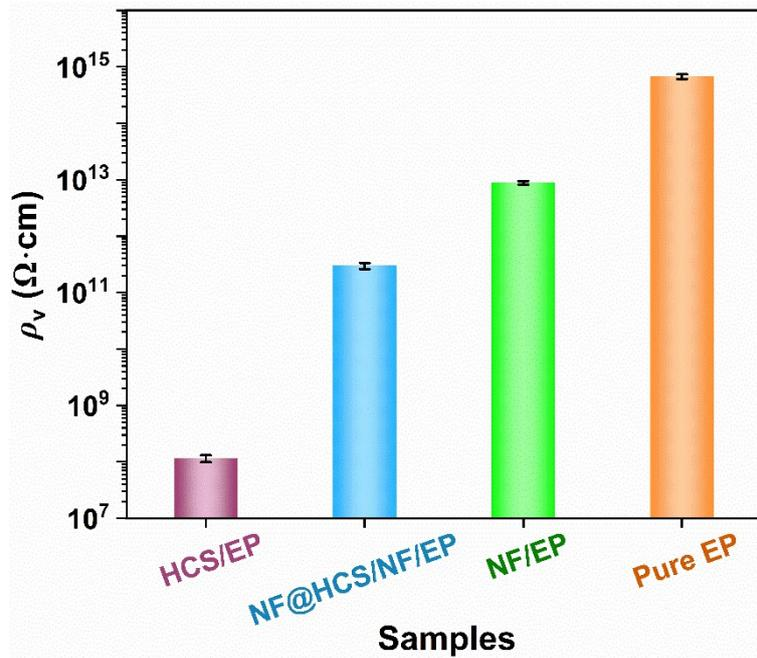
Fig. S12 The volumetric resistivity ( $\rho_v$ ) values of as-prepared composites.
