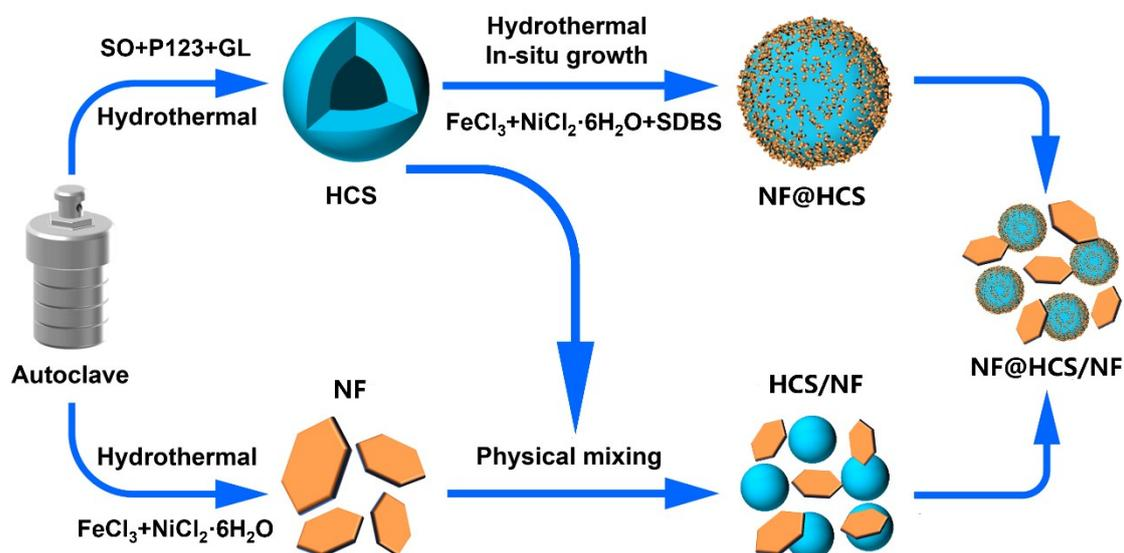
Fig. S1 The illustration of synthesis routes and relationships of HCS, NF, NF@HCS, HCS/NF, and NF@HCS/NF.
