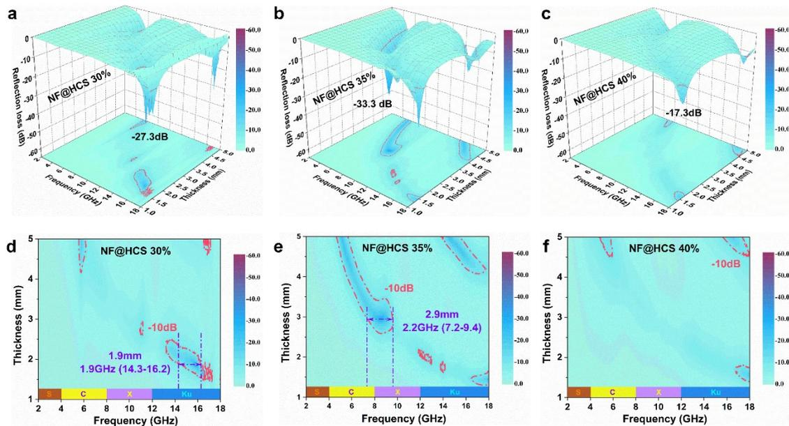
Fig. S5 The 3D RL diagrams and corresponding 2D RL mapping graphs of NF@HCS at different filling contents.
