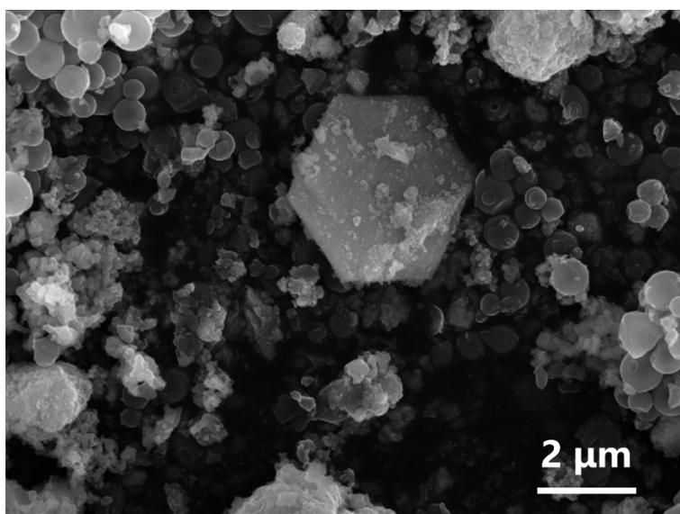
Fig. S3 The SEM image of NF@HCS/NF, showing the presence of HCS, microscale NF sheets, and nanoscale NF particles on HCS.
