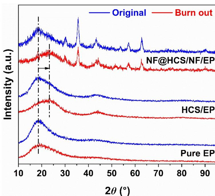
Fig. S11 The XRD patterns of pure EP, HCS/EP and NF@HCS/NF/EP before and after ignition. The red lines of burn-out samples show the phase and chemical stabilities of NF and HCS in the NF@HCS/NF/EP composites.
