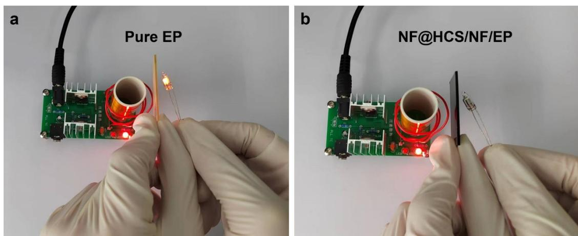
Fig. S10 The demonstration experiments via a Tesla coil showing the EMW absorption performance of (a) pure EP compared with (b) the as-prepared NF@HCS/NF/EP composite.
