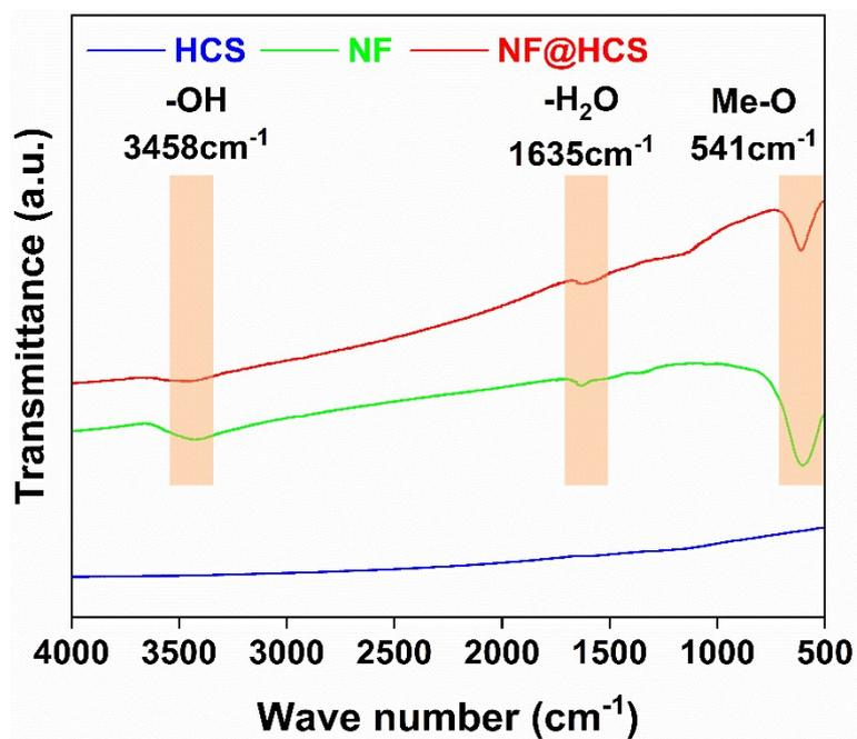
Fig. S2 The FT-IR spectroscopy of HCS, NF and NF@HCS. The Me-O vibration peaks around  $541\text{ cm}^{-1}$  show the existence of NF and successful combination of NF and HCS.
