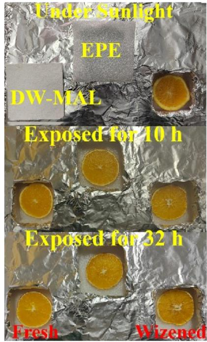
**Figure S9.** Orange preservations by the DW-MAL composite (the controlled groups were cover by a EPE foam or exposed to open air).
