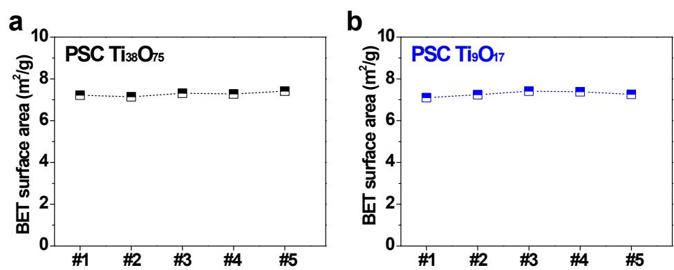
Figure S3. The specific surface area of PSC  $\text{Ti}_n\text{O}_{2n-1}$  ( $n=9, 38$ ) monoliths. (a) PSC  $\text{Ti}_{38}\text{O}_{75}$ . (b) PSC  $\text{Ti}_9\text{O}_{17}$ .
