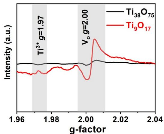
Figure S5. EPR spectra of PSC  $\text{Ti}_{38}\text{O}_{75}$  and  $\text{Ti}_9\text{O}_{17}$ .
