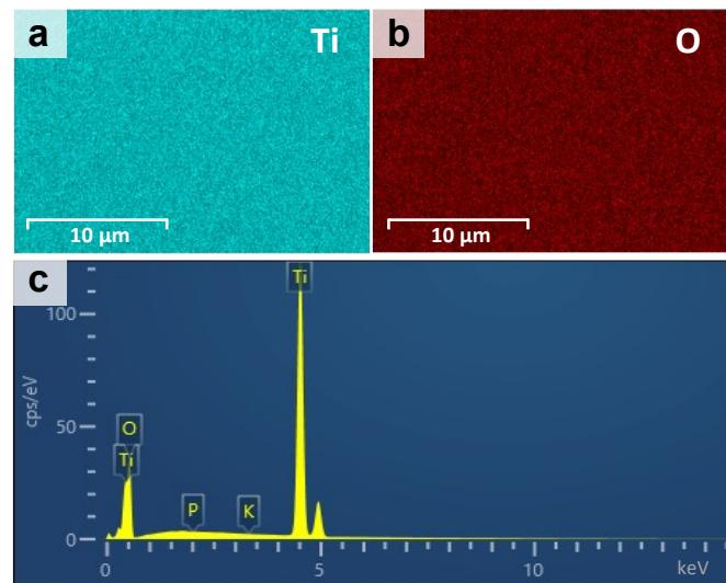
Figure S2. (a-b) Element mapping of PSC rutile  $\text{TiO}_2$  monolith. (c) EDS test of PSC rutile  $\text{TiO}_2$  monolith.
