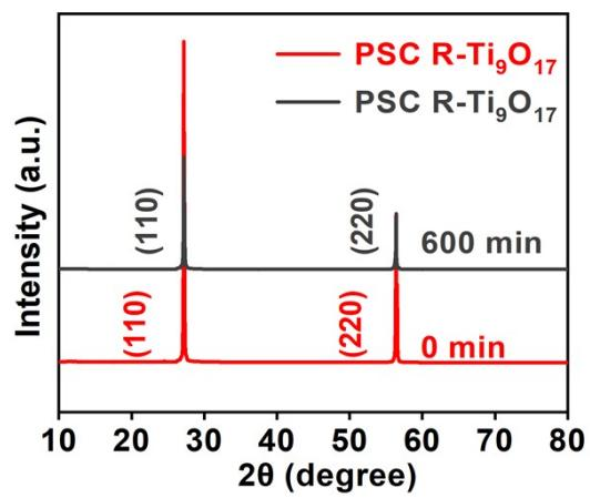
Figure S10. XRD patterns of the PSC R-Ti<sub>9</sub>O<sub>17</sub> catalyst after the stability test.
