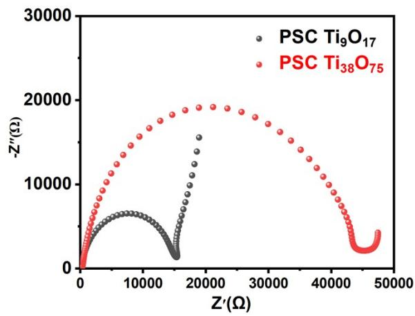
Figure S8. Impedance spectra of PSC  $\text{Ti}_9\text{O}_{17}$  and  $\text{Ti}_{38}\text{O}_{75}$  electrode in 1 M NaOH electrolyte.
