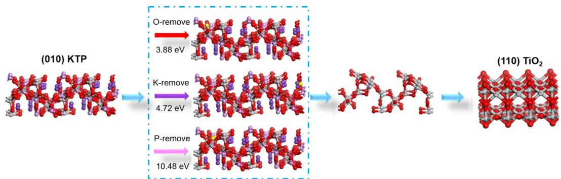
Figure S4. Theoretical calculations of energy barrier for transformation from (010) KTP to rutile (110)  $\text{TiO}_2$ .
