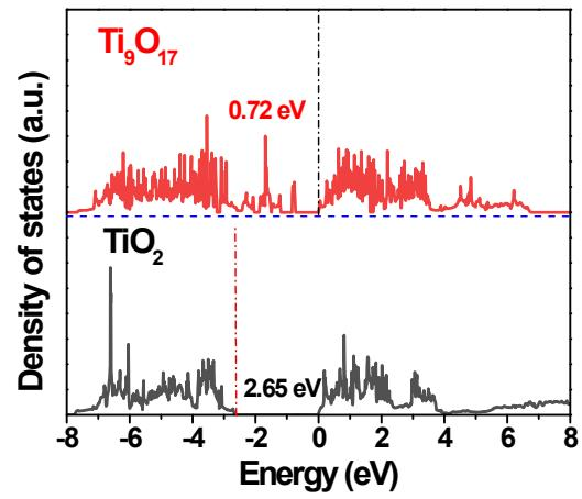
Figure S6. Density of states for rutile  $\text{TiO}_2$  and  $\text{Ti}_9\text{O}_{17}$ .
