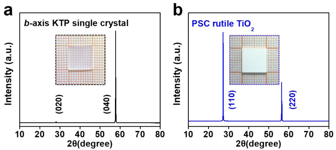
Figure S1. (a-b) XRD patterns of (020) KTP single crystal and PSC rutile (110)  $\text{TiO}_2$ . The insets are optical photographs, respectively.
