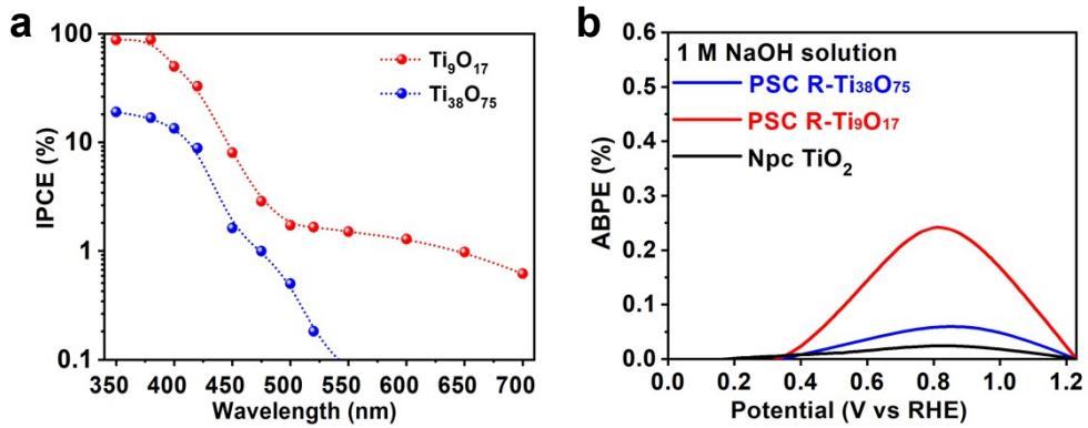
Figure S9. (a) IPCE measurements for PSC rutile (110)  $\text{TiO}_2$  at 1.23V in 1M NaOH. (b) ABPE curve for PSC rutile (110)  $\text{TiO}_2$  monolith under 10 AM 1.5 G illumination.
