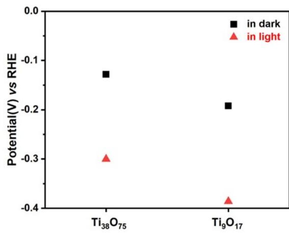
Figure S7. Open circuit potential for PSC  $\text{Ti}_{38}\text{O}_{75}$  and  $\text{Ti}_9\text{O}_{17}$  photoelectrodes under dark and illuminated conditions in 1 M NaOH electrolyte.
