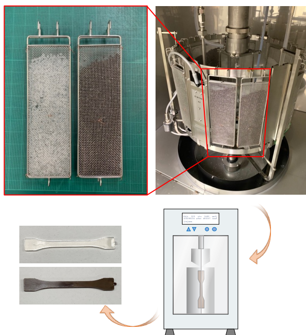
Figure S2. Overview of the degradation/recycling flow used in this study. Pellets are inserted into a stainless steel mesh holder with a gap roughly the width of a pellet, which ensures fairly uniform exposure by limiting overlap and crowding. After 300 MJ/m 2 of UV irradiation (equivalent to at least 1 year of sunlight), the pellets are carefully removed and either injected molded as-is or subjected to further processing before molding.
