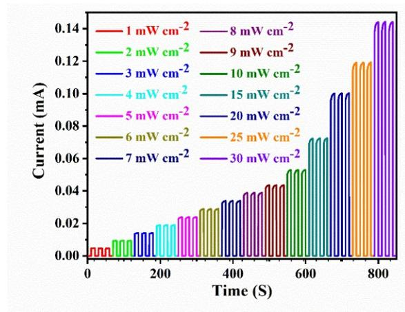
**Figure S10.** Photocurrent response to on/off light of photodetector irradiated in 1050 nm light with different power density from 1 to 30  $\text{mW cm}^{-2}$
