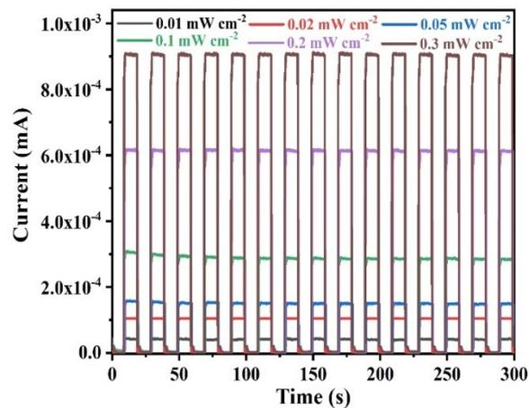
**Figure S11.** Photocurrent response to on/off light of photodetector irradiated in weak irradiation with the power density lower than  $0.3 \text{ mW cm}^{-2}$
