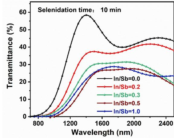
**Figure S6.** the Ultraviolet-Visible-near infrared (UV-Vis-NIR) spectrum of films with different In/Sb ration selenized for 10 min.
