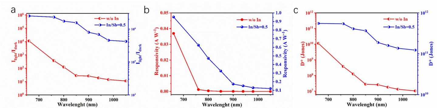
**Figure S8.** Supplementary comparison of response for  $\text{AgSbS}_2/\text{CdS}$  heterojunction device without and with indium. The comparison of (a) switching ratio, (b) responsivity, (c) detectivity for the two photodetectors.
