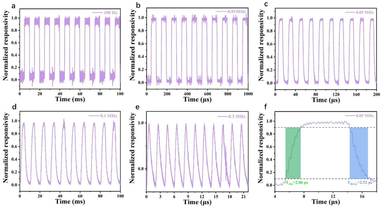
**Figure S12.** Frequency response of photodetector on 980 nm laser. The response of the Ge detector to square wave incident light source with the frequencies of (a) 100Hz, (b) 0.01MHz, (c)0.05MHz, (d) 0.1 MHz, (e) 0.3MHz, and (f) response time of the photo detector.
