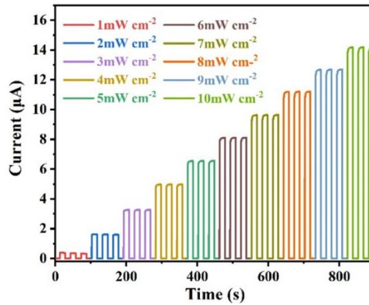
**Figure S7.** Photocurrent response of indium-free photodetector to on/off light at different power densities of 660 nm.
