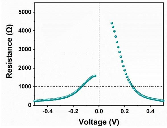
**Figure S9.** Resistance of the devices derived from J-V curve test in dark.
