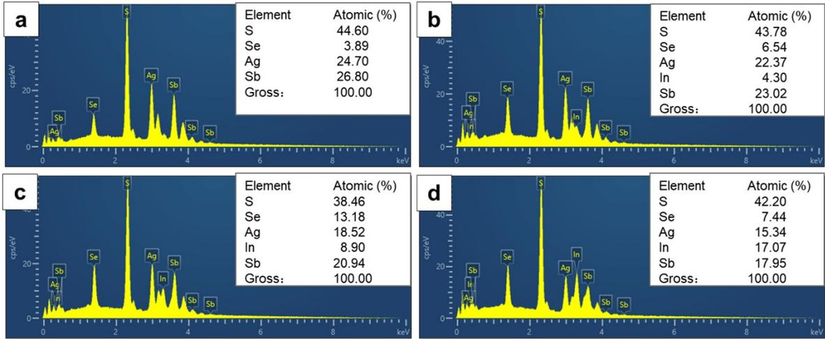
**Figure S1.** The EDS analysis for  $\text{AgSbS}_2(\text{Se})$  films that selenized for 4 min with different indium concentration. (a)  $\text{In/Sb}=0$ , (b)  $\text{In/Sb}=0.2$  (c)  $\text{In/Sb}=0.5$  and (d)  $\text{In/Sb}=1$
