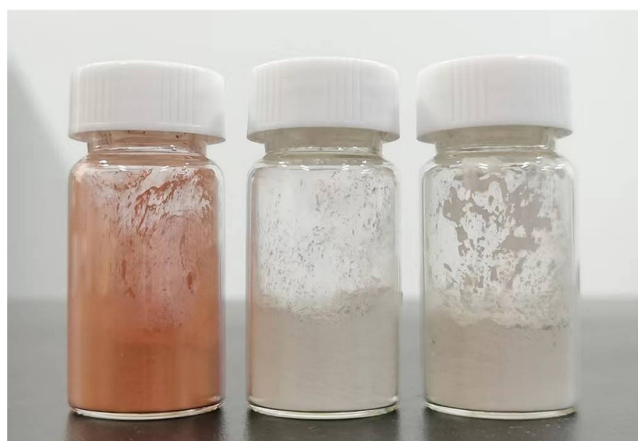
Fig. S15 Photographs of Cu powder, tetradecahedral Cu@Ag powder (Sample S1), and spherical Cu@Ag powder (Sample S2).
