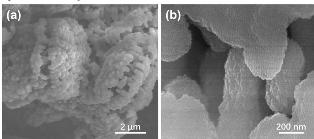
**Figure S4.** SEM images of shell-like carbon superstructures.
