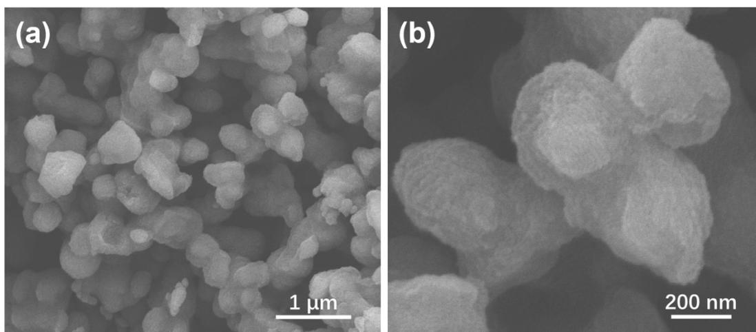
**Figure S2.** SEM images of sphere-like carbon materials.
