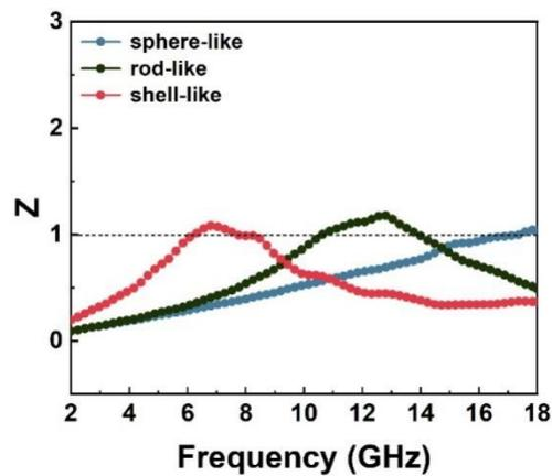
**Figure S9.** Z values vs frequency of three samples at the thicknesses corresponding to their respective strongest reflection loss values.
