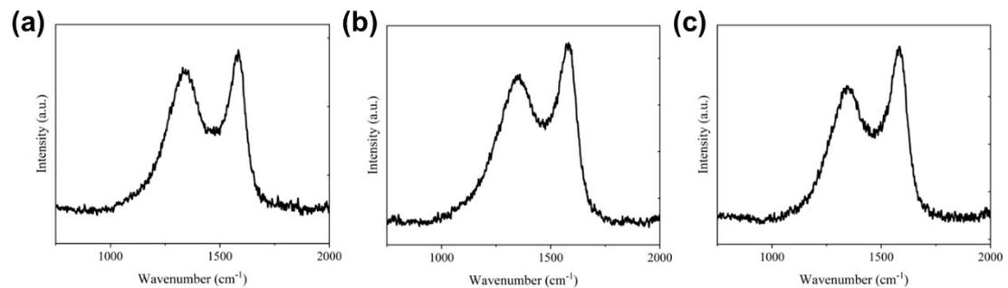
**Figure S7.** Raman spectra of (a) sphere-like, (b) rod-like, and (c) shell-like carbon superstructures.
