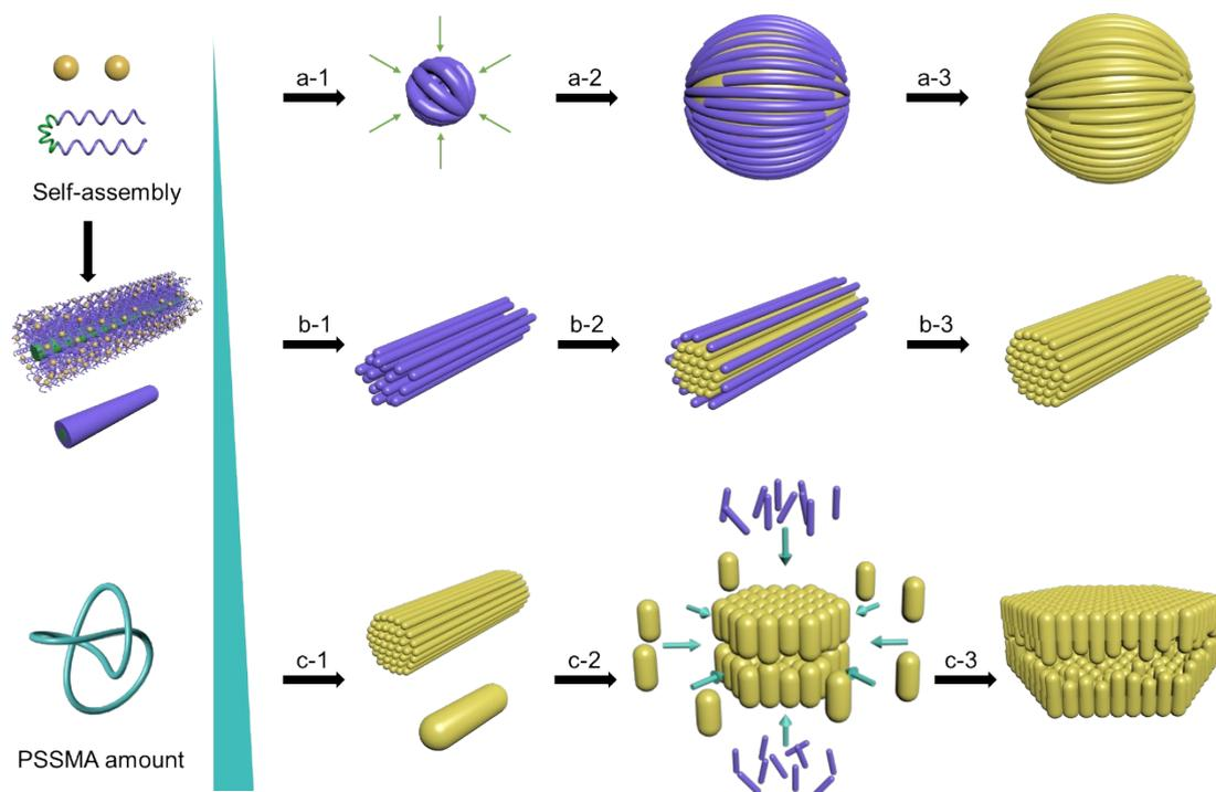
**Figure S1.** The formation mechanism of various carbon materials with different PSSMA amount. (a) sphere-like carbon material without PSSMA, (b) rod-like carbon material with 100 mg of PSSMA, and (c) shell-like carbon superstructure with 150 mg of PSSMA.
