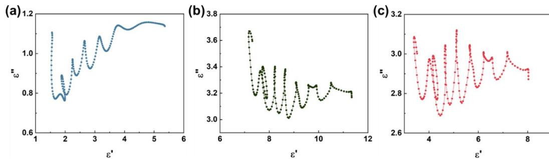
**Figure S10.** Cole-Cole curves vs frequency of (a) sphere-like, (b) rod-like, and (c) shell-like carbon superstructures.
