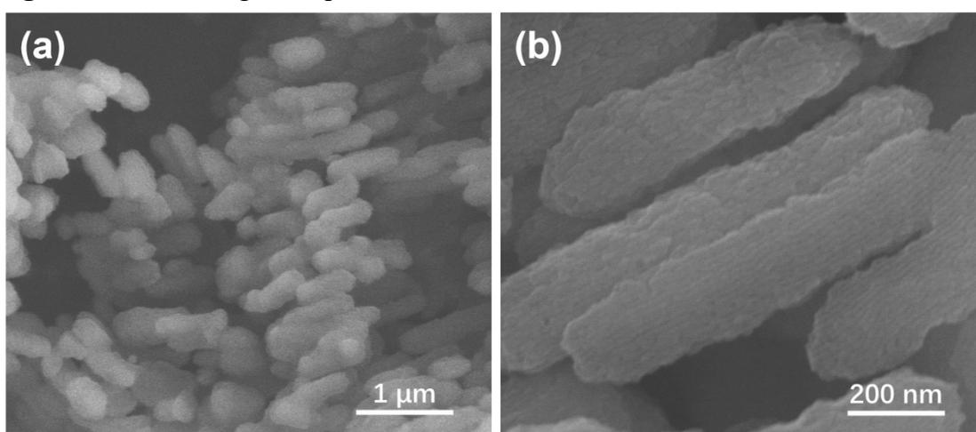
**Figure S3.** SEM images of rod-like carbon materials.
