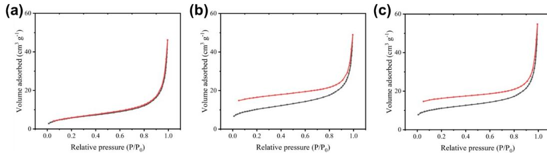
**Figure S6.** Nitrogen adsorption-desorption isotherms of (a) sphere-like, (b) rod-like, and (c) shell-like carbon superstructures.
