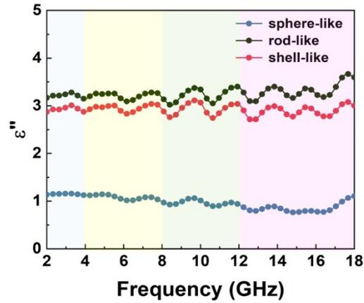
**Figure S8.** Imaginary part of the permittivity vs frequency of sphere-like, rod-like and shell-like carbon superstructures.
