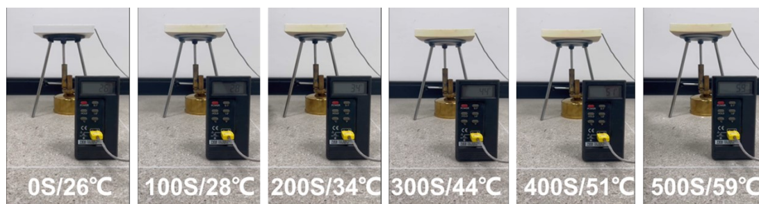
Figure S10. Live view of alcohol blowtorch heating aerogel plate.
