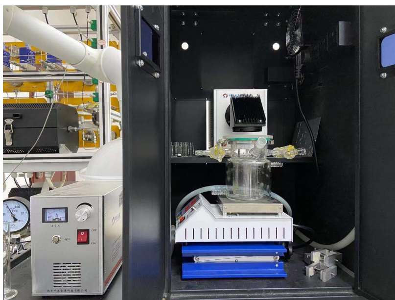
Fig. S1. The device picture of photocatalytic reduction of CO 2 reaction.
