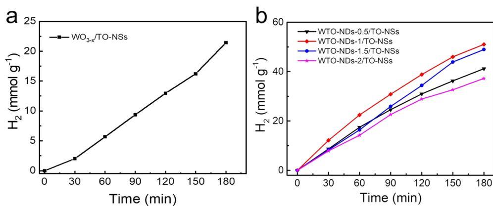
Figure S7. Hydrogen generation over  $\text{WO}_{3-x}/\text{TO-NSs}$  photocatalyst (a) and various WTO-NDs/TO-NSs heterostructures (b)
