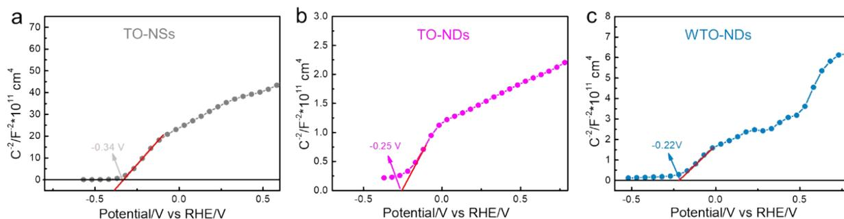
Figure S12. Mott-Schottky plots of TO-NSs, TO-NDs and WTO-NDs measured in a NaOH (1 M; pH 13.6) electrolyte at frequencies 1000 Hz.
