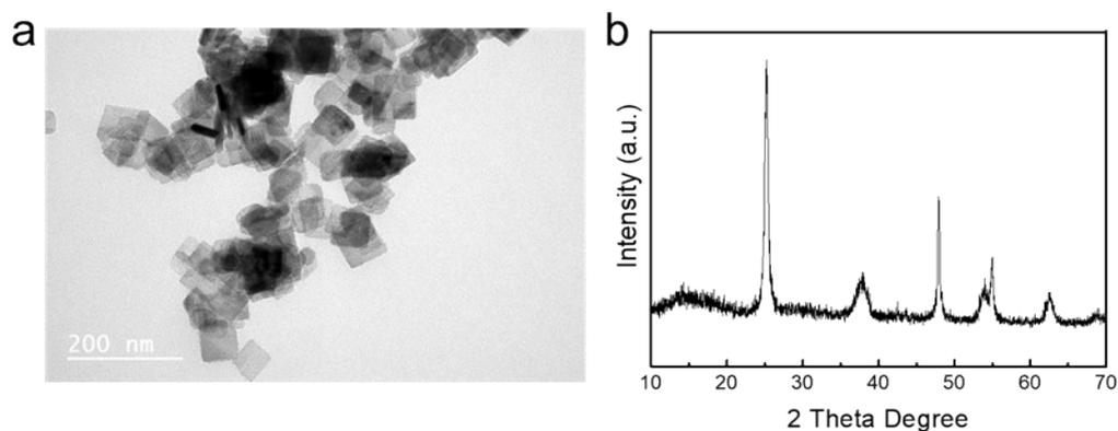
Figure S8. The TEM image and XRD patterns of WTO-NDs/TO-NSs heterostructures after photocatalysis
