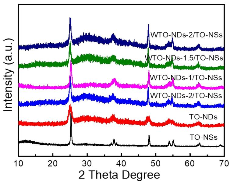
Figure S3. XRD patterns of WTO-NDs/TO-NSs heterostructures
