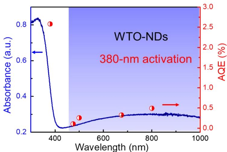
Figure S10. DRS and apparent quantum efficiency (AQE) of WTO-NDs with 380-nm activation during photocatalytic hydrogen generation.
