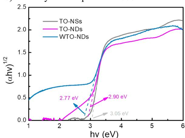
Figure S13. The transformed Kubelka-Munk function vs the energy of light for TO-NSs, TO-NDs and WTO-NDs.
