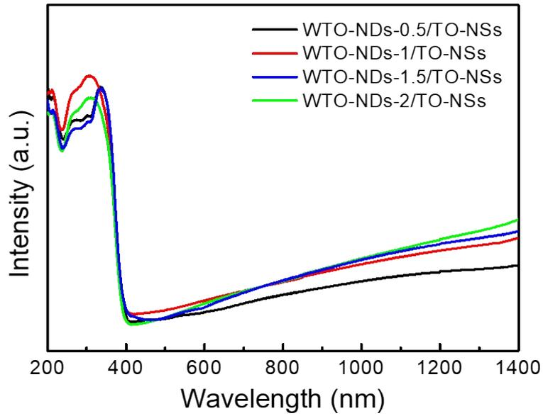
Figure S4. DRS spectral of WTO-NDs/TO-NSs heterostructures
