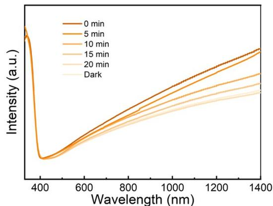
Figure S6. UV-vis-NIR DRS changes of WTO-NDs-1/TO-NSs heterostructure after stopping light irradiation
