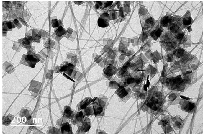
Figure S2. The TEM image of the  $\text{WO}_{3-x}/\text{TO-NSs}$  photocatalyst
