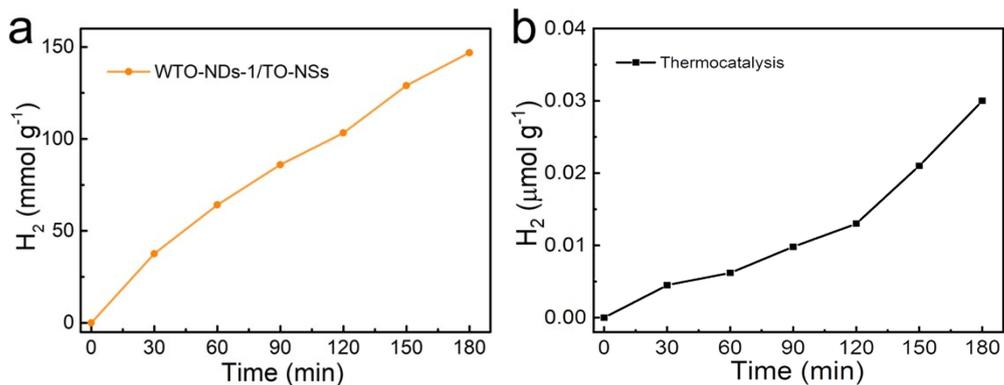
Figure S9. The photothermocatalytic (a) and thermocatalytic (b) hydrogen generation over WTO-NDs-1/TO-NSs heterostructure
