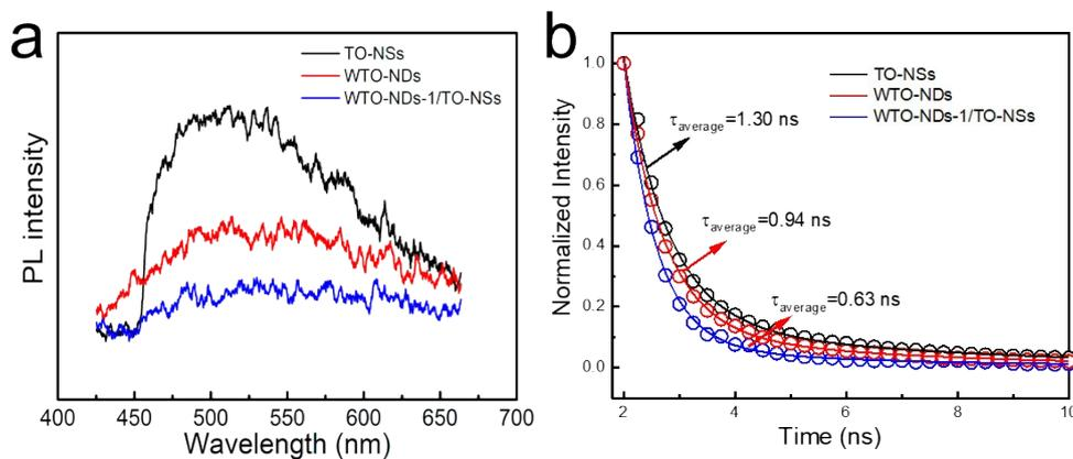
Figure S11. The steady-state and time-resolved PL spectra of TO-NSs, WTO-NDs and WTO-NDs-1/TO-NSs
